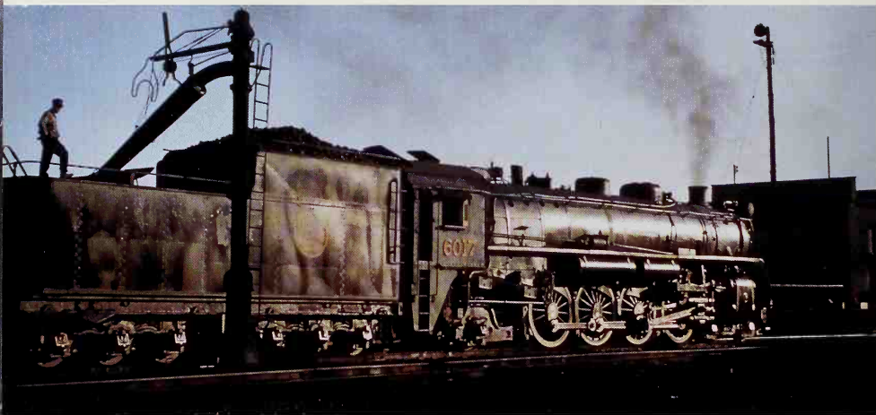
A Canadian National 4-8-2 Mountain type catches a glint of the setting sun as it is being watered. CN operated a large fleet of 4-8-2s and was one of the first railroads to adopt the 4-8-4 wheel arrangement, essentially an expansion of the 4-8-2 type. Donald Fellows
