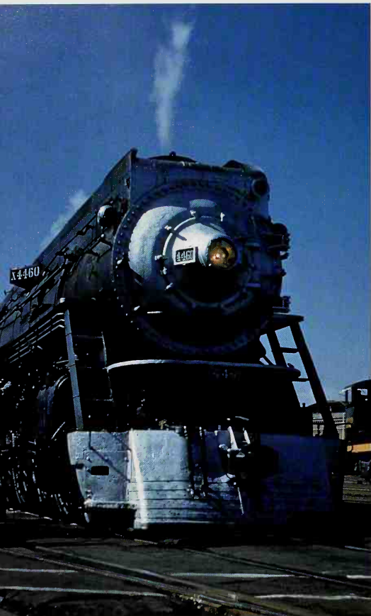
Southern Pacific's last new 4-8-4s were 10 GS-6s built by Lima in 1943. These were built to comply with War Production Board restrictions and were less impressive than SP's earlier GS-4 and GS-5 4-8-4s. They used smaller drivers, and did not feature the elaborate Daylight coloring as SP's earlier Lima 4-8-4s. Fred Matthews
