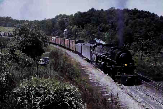
On July 31, 1958, a Norfolk & Western A Class 1233 leads an eastbound mixed freight at Blue Ridge, Virginia. One of N&W's big Y class 2-8-8-2 Mallet Compounds is shoving hard on the rear of the train. N&W developed the A class simple articulated in 1936 for high-speed mainline service, and ultimately N&W built 43 of the type. Richard Jay Solomon
