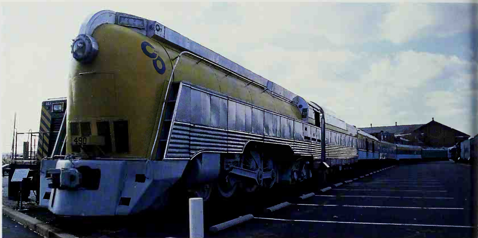
In 1946 and 1947, Chesapeake & Ohio rebuilt five 4-6-2 Pacifics into modern 4-6-4 Hudsons. They featured roller bearings and rotary cam poppet valves. Four received distinctive stainless-steel shrouding. One locomotive was preserved, and it is one of only a handful of American streamlined steam locomotives that escaped the scrap heap. Today it is displayed at the Baltimore & Ohio Railroad Museum in Baltimore, Maryland. Brian Solomon
