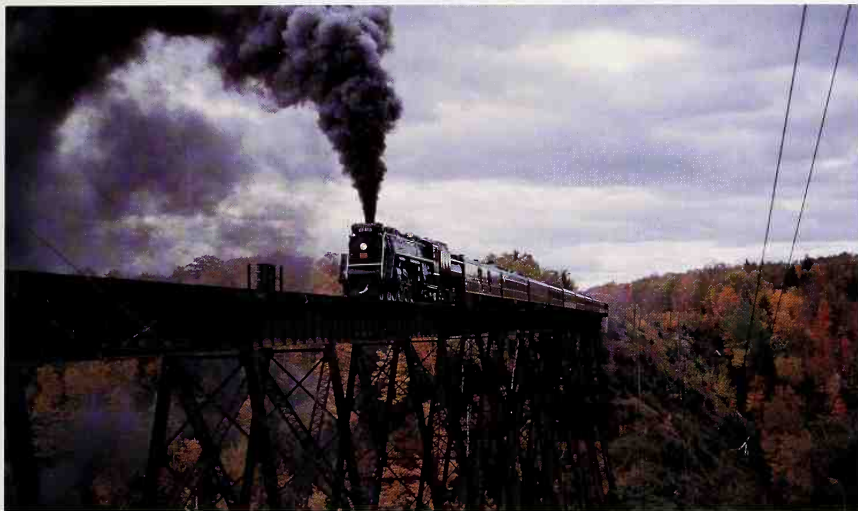
Canadian National operated more 4-8-4s than any other railroad in North America. Its 4-8-4s were lightweights compared to most operated in the United States. No. 6218 weighed just 399,000 pounds, 110,000 pounds less than Santa Fe's big 4-8-4s of the same period. CN 6218 leads an excursion across a large trestle in Quebec in October 1964. Richard Jay Solomon
