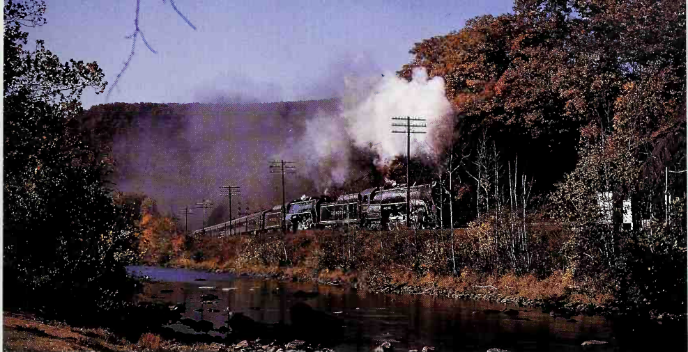
A pair of Reading T-1s, led by No. 2100, haul a well-patronized "Reading Ramble" excursion in eastern Pennsylvania on a crisp October day in 1963. Between 1945 and 1947, Reading constructed 30 4-8-4s using boilers from old 2-8-0 Consolidations. The T-1 4-8-4s were intended for freight service, but three of them operated in passenger excursion service after Reading dieselized its freight operations. Richard Jay Solomon
