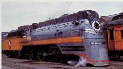
Milwaukee Road was famous for its high-speed streamlined 4-4-2 Atlantics and 4-6-4s, but it also streamlined some older power. It rebuilt two of its F5 Pacifics with Otto Kuhler-designed shrouds for service on the Sioux Falls, South Dakota, section of the Midwest Hiawatha . Streamlined Pacific No. 801 is seen at Sioux City, Iowa, in the 1940s.
