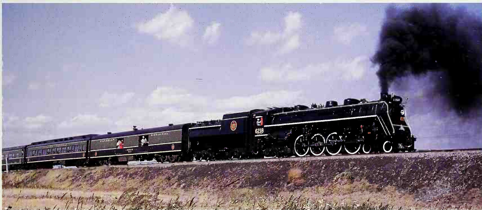
Canadian National 6218 is a Class U-2-g 4-8-4 that was built by the Montreal Locomotive Works, Alco's Canadian affiliate, in September 1942. It was a typical example of CN's later 4-8-4s featuring 73-inch drivers, which made it ideal for both passenger and freight work. It is seen hauling an excursion in Quebec in October 1964. Richard Jay Solomon
