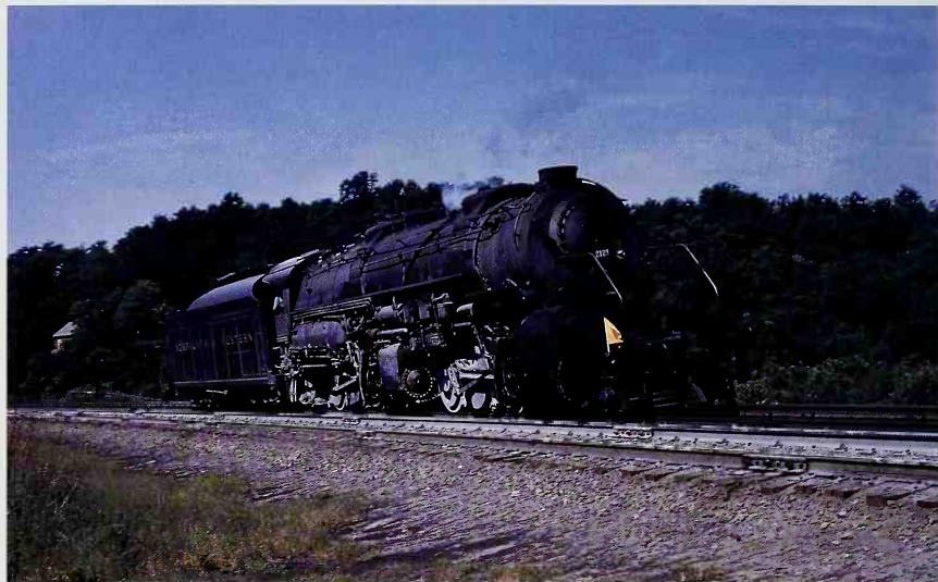
Norfolk & Western Y6 2-8-8-2 No. 2129 drifts downgrade at Blue Ridge, Virginia, after working as a pusher on the end of a heavy freight. A compound locomotive is easily identified by its enormous low-pressure front cylinders. By 1958, N&W was one of the last railroads operating big steam, and its compounds were a technological anomaly; most American railroads abandoned compound steam designs in the 1920s. Richard Jay Solomon
