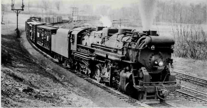
The secret to the Berkshire's success was its large firebox and ample boiler, which allowed the engine to haul heavy tonnage at sustained speeds without running out of steam. In 1938, a 12-year-old Lima-built A-1 Berkshire leads a freight through Englishman's Curve at East Chatham, New York, on the west end of the Boston & Albany line. It was on this piece of railroad that Lima's first 2-8-4 demonstrated its abilities in 1925. J. R. Quinn collection
