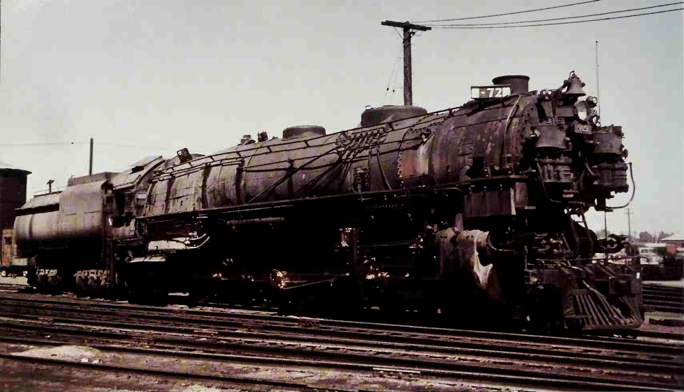
In the 1920s, Alco promoted the three-cylinder simple locomotive as a way of obtaining greater power from a nonarticulated engine. The third cylinder was located below the smoke box between the two outside cylinders and drove a cranked axle. The largest three-cylinder locomotives were a fleet of 88 4-12-2s built for Union Pacific between 1926 and 1930. These were also the largest American locomotives with a rigid frame and were designated the Union Pacific type. Union Pacific 4-12-2 No. 9051 rests at Omaha, Nebraska, in 1954. Union Pacific Museum Collection
