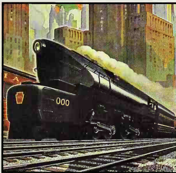
One of the largest fleets of streamlined steam locomotives was Pennsylvania Railroad's unusual T1 Duplexes. These locomotives featured two complete sets of running gear on a rigid frame and were designed for 100-miles-per-hour operation. PRR T1 is portrayed in a World War II-era advertisement. Author collection
