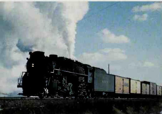
In February 1958, a Nickel Plate Road 2-8-4 Berkshire leads a westbound freight through Hobart, Indiana. The last steam locomotive built by Lima was Nickel Plate 2-8-4 No. 779. It was constructed in 1949, roughly 25 years after Lima had introduced the type with its famous A-1. Russ Porter
