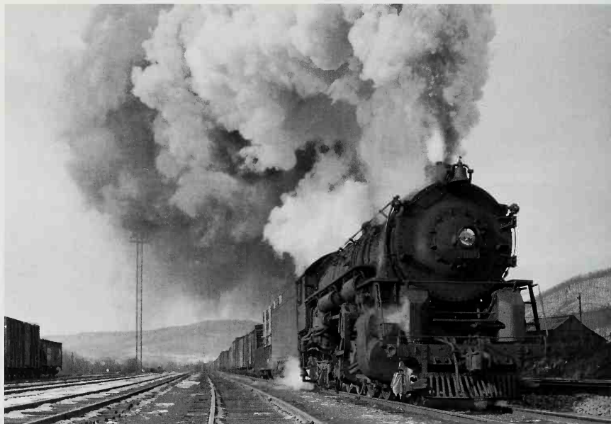
The Erie Railroad was the first line to use Berkshires capable of high-speed freight operation. Its 2-8-4s used 69-inch drivers, instead of the 63-inch drivers used on the original A-1 Berkshire. The Erie was one of several railways under control of the Van Swerigan brothers, and Erie's Berkshires set a precedent for motive power design on the other Van Swerigan lines. A Baldwin-built S-3 2-8-4 leads a freight out of Erie's East Hornell, New York, yards. John Long, Erie Railroad, Tim Doherty collection
