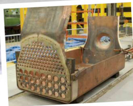
↑ The Unknown Warrior's inner firebox crownsheet and tubeplate temporarily assembled at Crewe. ZOE HUNTER
