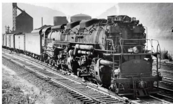
← Chesapeake & Ohio Class 'H8' 2-6-6-6 No. 1638 leaves Handley, West Virginia, in August 1953. Despite the final batch being received in late 1948, by 1954 all 60 engines were out of service, although a few were briefly brought back into use during 1956. Two examples have been preserved. J. G. COLLIAS
