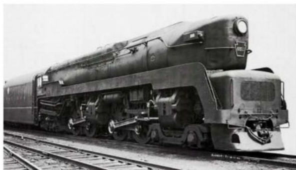
← Pennsylvania Railroad 'Duplex' four-cylinder rigid frame 4-4-4-4, No. 5511, one of 52 such locomotives built in 1942 and 1945-46, retired between 1951-53. AUTHOR'S COLLECTION
