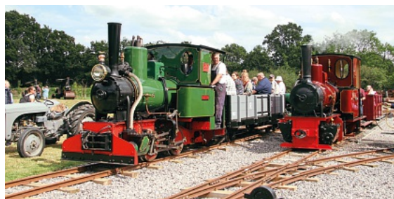
Arn Jung 3175/1921 0-4-OWT Jenny arrives at Richmond Light Railway's main station (visiting Simplex 9869/1953 No. 12 Bicknor is on the tail) with a branch line train, while Orenstein & Koppel 3136/1908 0-4-OWT Susan (right) waits to depart with the other passenger train around the main circuit. CLIFF THOMAS
