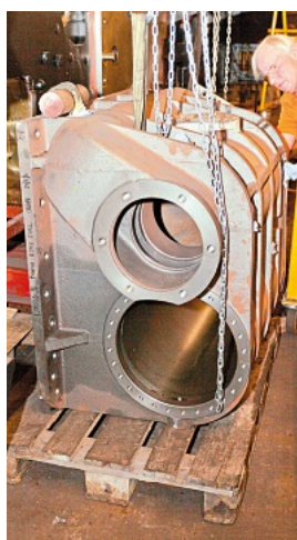
The new-design cylinders are offered to the frames of No. 6024 in early September. CHRIS NICHOLSON
