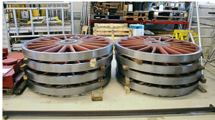
The eight proof-machined 6ft 2in driving wheels for the P2 sit neatly stacked at Darlington. The tyres have been delivered and the target is to have a rolling chassis by next winter. A1SLT
