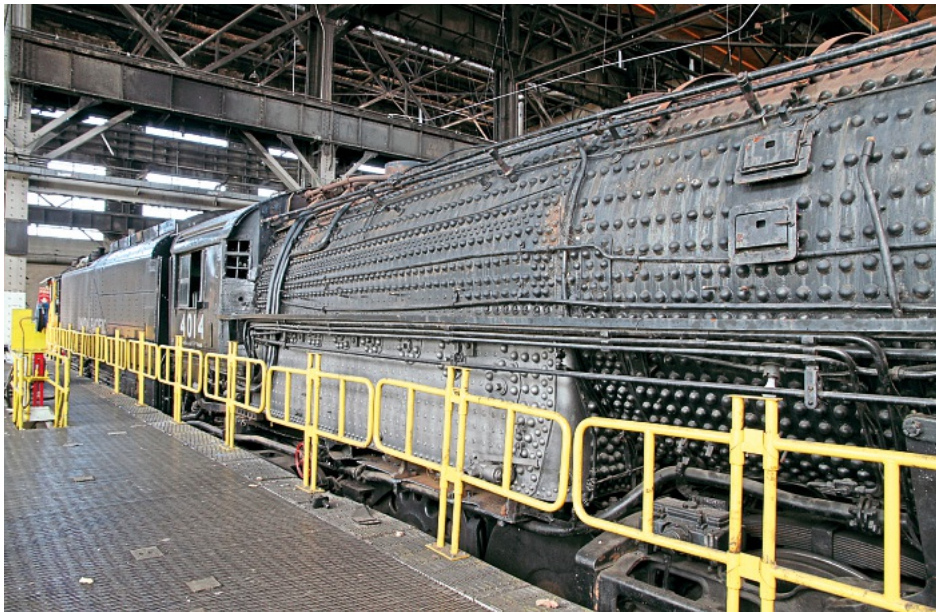
Above: No. 4014 inside the UP heritage workshop at Cheyenne in September 2014. A false ceiling that was the height of the small girder above the tender has been removed to allow a 250-ton travelling crane to be installed. CHRIS MILNER
