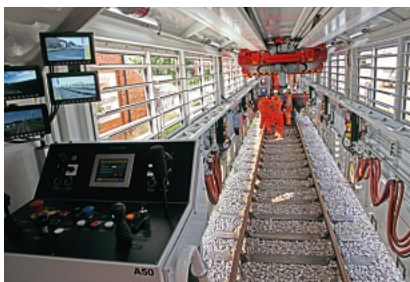
The view inside the maintenance carriage with its extendable sides.
