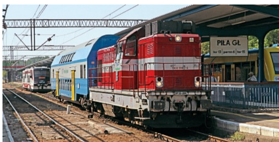
Possibly the last of its type in passenger service: PR-operated SP32 206 at Piła on August 19, deputising for a DMU with a single double-deck coach, working a service to Chojnice. Four built 150 of these ETH-fitted locos in Romania between 1985 and 1991. Never very reliable, 10 were rebuilt with MTU 12V396TC14 diesel engines from 2000 onwards. Only around 15 SP32s remain officially in service – mostly the rebuilt SP 32 200 series locos – although almost all of these are stored, especially at Krzyż and Chojnice in Northern Poland. KEITH FENDER
