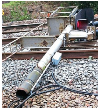
The corroded signal post lying across the down line. RAIB
