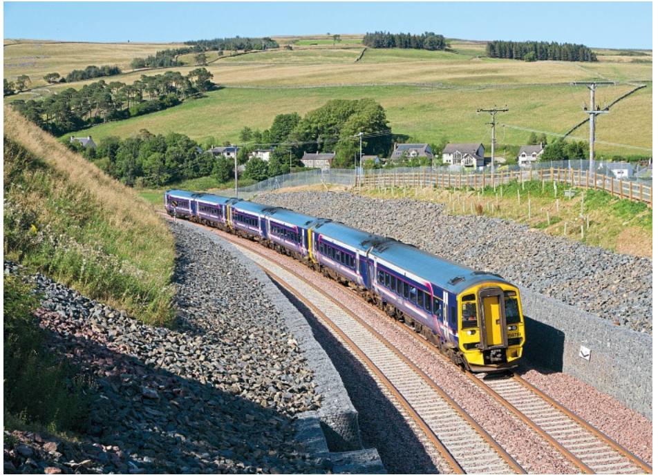
Above: Slowing for the station call at Stow on September 6 are unit Nos. 158718/712/714 arriving with the 14.11 Waverley to Tweedbank. The gabions are a feature at locations along the line to strengthen embankments. CHRIS MILNER
