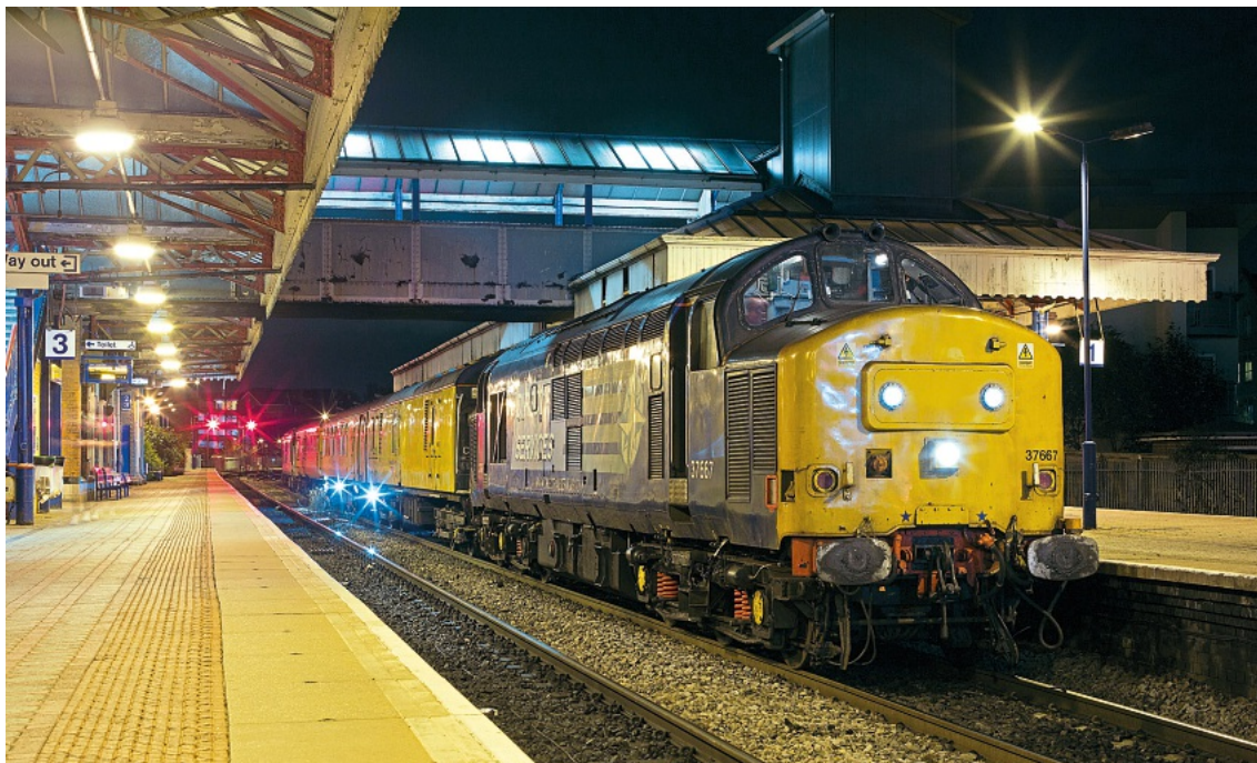
DRS Class 37 No. 37667 top-and-tails with 37605 on an ultrasonic test train at Aylesbury on August 28. Train 3Q23 was the 19.58 from Old Oak Common to Derby RTC and had paused at platform 2 to allow the ultrasonic probes to be lowered, ready to monitor the single line to Claydon Jct. ANDREW ROYLE
