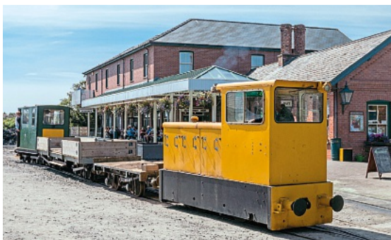
Tallyllyn Railway's ex-RNAD Trecwn 99hp Baguley Drewry diesel (3779/1983) No. 11 enjoyed a rare appearance in the limelight during The 1865-2015 gala, held at the line on August 7-9. It is seen at Wharf on August 8 with a demonstration works train. The second of TR's ex-Trecwn locos to be regauged from 2ft 6in to 2ft 3in by Alan Keef Ltd (No. 12) returned to Tywyn on August 4. The pair will be officially named Trecwn and St. Cadfan . BARBARA FULLER
