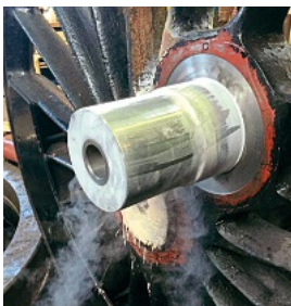
One of the new crank pins being fitted to the wheels of No. 70013 at Bury on September 16, having been frozen in liquid nitrogen to ensure an accurate fit. IAN RILEY
