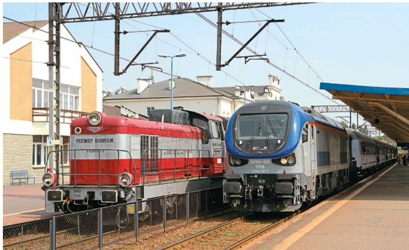
New this year – in service since April – the first Pesa 'Gama' diesel for PKP IC, SU160001, at Lublin on August 13, backing on to a TLK semi-fast train to Rzeszów. On the left is older PR-operated SU42 535, being used as station pilot loco, moving empty stock. These locos have lost nearly all their passenger work. KEITH FENDER
