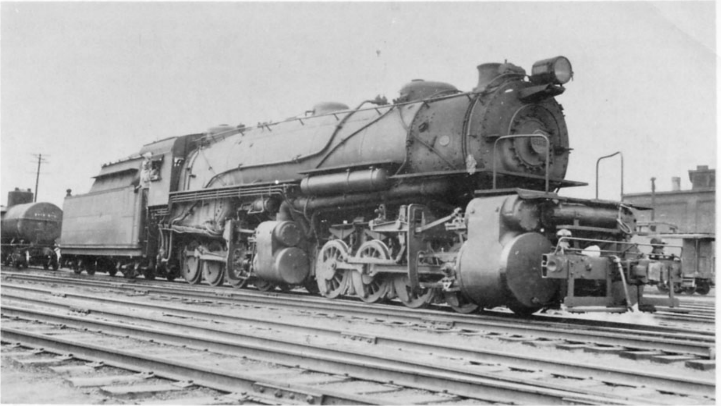
Mallets for heavy switching, particularly hump work, were a feature of the Eastern American scene. Pennsylvania CC-2S No 8183, a compound 0-8-8-0, is seen above at Columbus, Ohio, in April 1938
