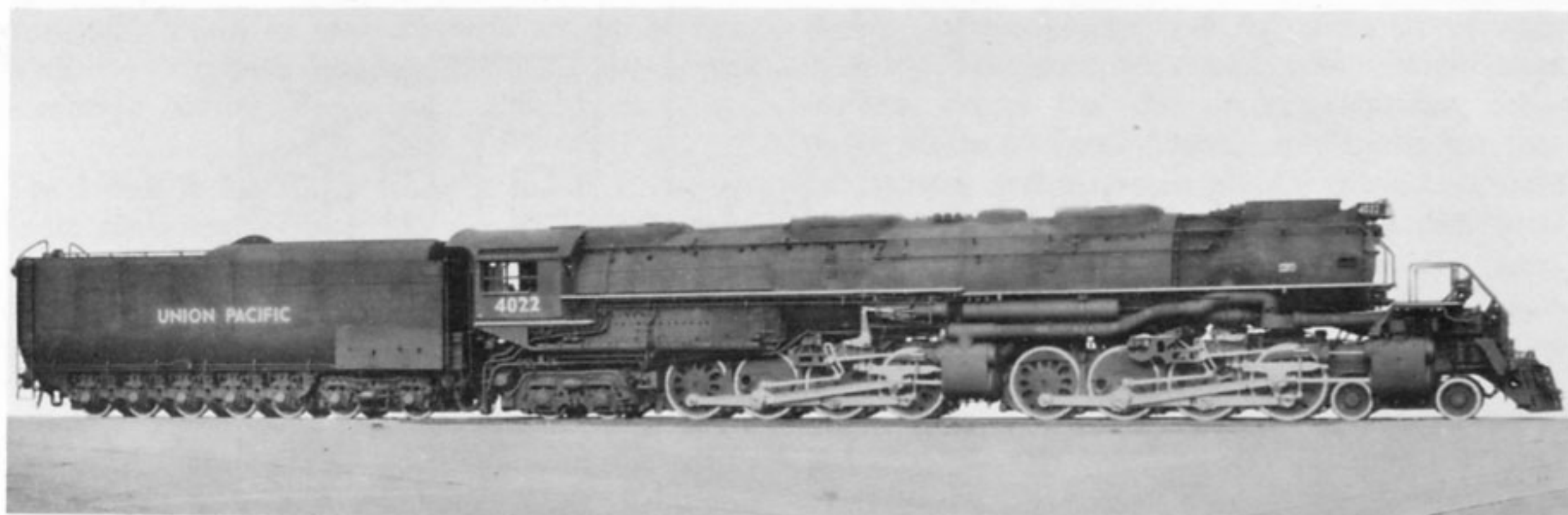
Final Mallet development was Union Pacific's class of gigantic yet superbly proportioned 'Big Boy' 4-8-8-4s. A straight enlargement of the Challenger 4-6-6-4, they combined 80mph speed potential with the highest haulage capacities
