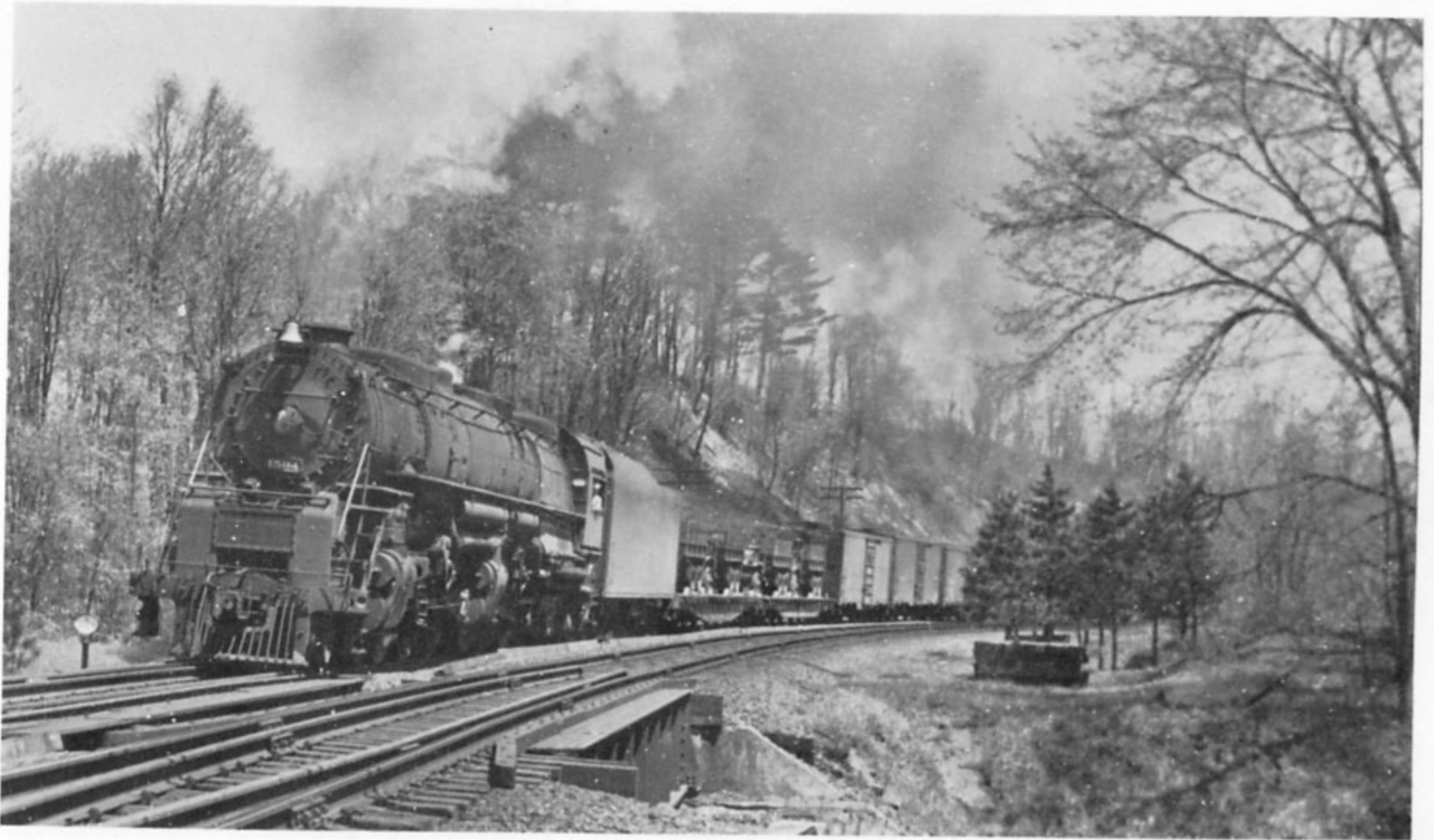
Delaware & Hudson's 4-6-6-4s, uncluttered and with shapely chimney, were Anglicised in style if not in size. Here No 1504 leaves Schenectady, NY, home of its builder Alco, with a 73-car westbound freight in 1950
