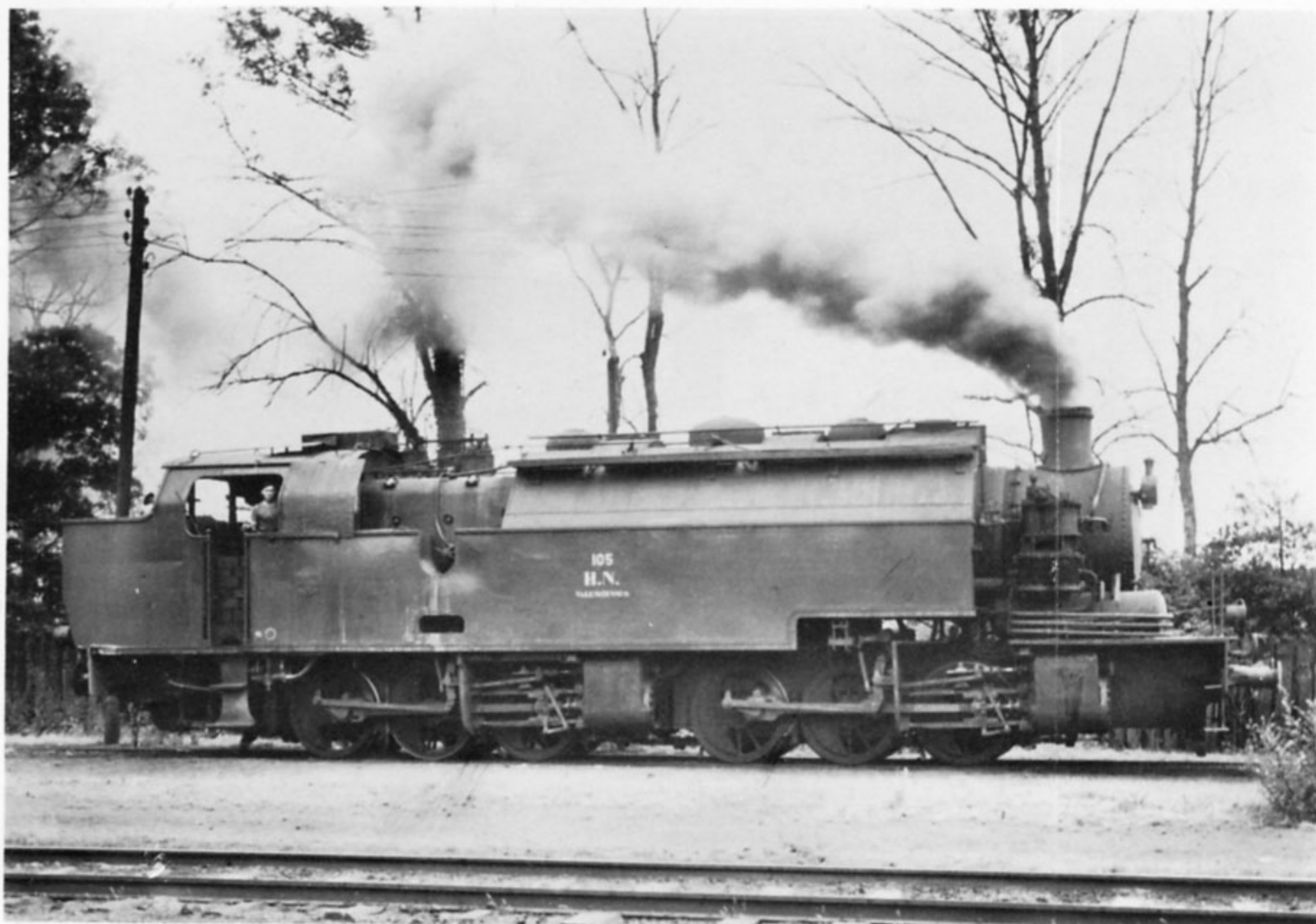
French simple expansion Mallets—3, HN No 105, built in 1940 with combined saddle and side tanks. Valenciennes, 1952
