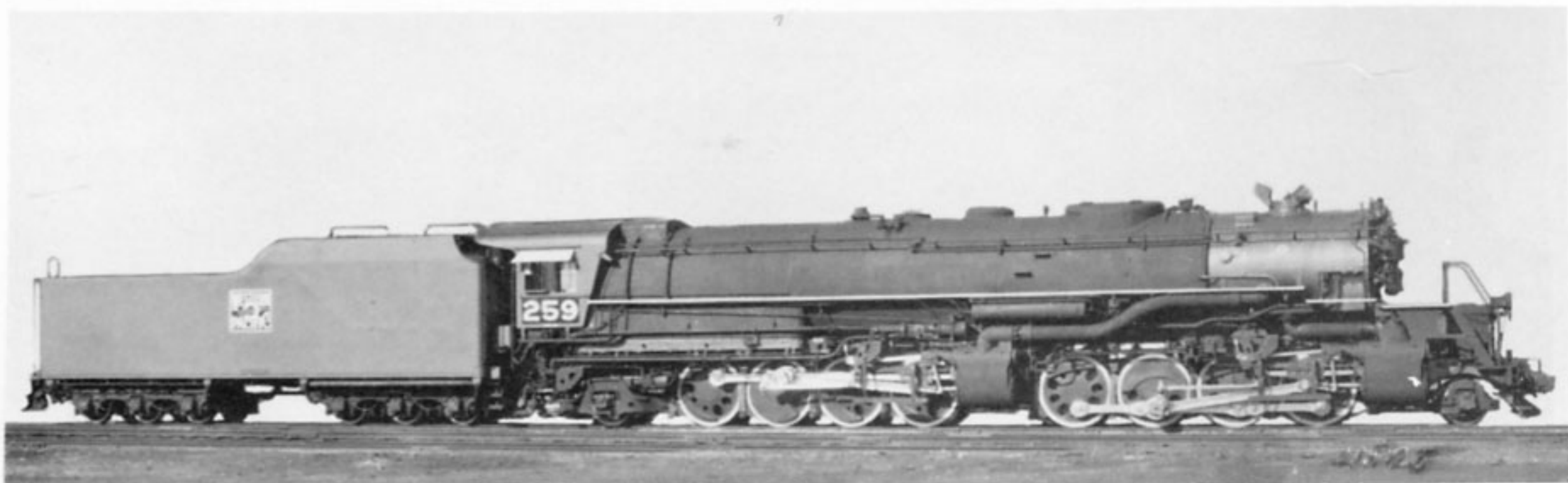
American 2-8-8-2 Mallets: Western Pacific's massive simple expansion engines of 1938 were among the largest of this type ever built
