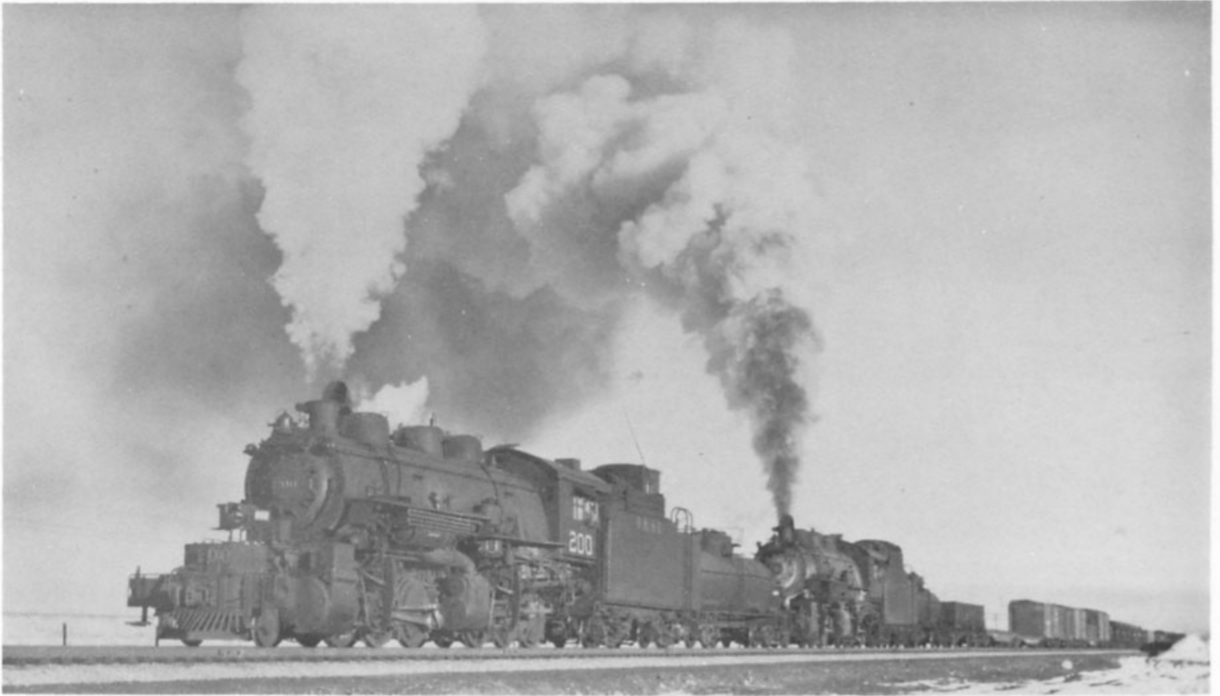
Two 2-6-6-0s on the Denver & Salt Lake Railroad, No 200 (rebuilt from 0-6-6-0) and No 216, storm up a 1 in 50 gradient near Leyden Junction, Colorado, in November 1947 hauling sixty-one bogie cars
