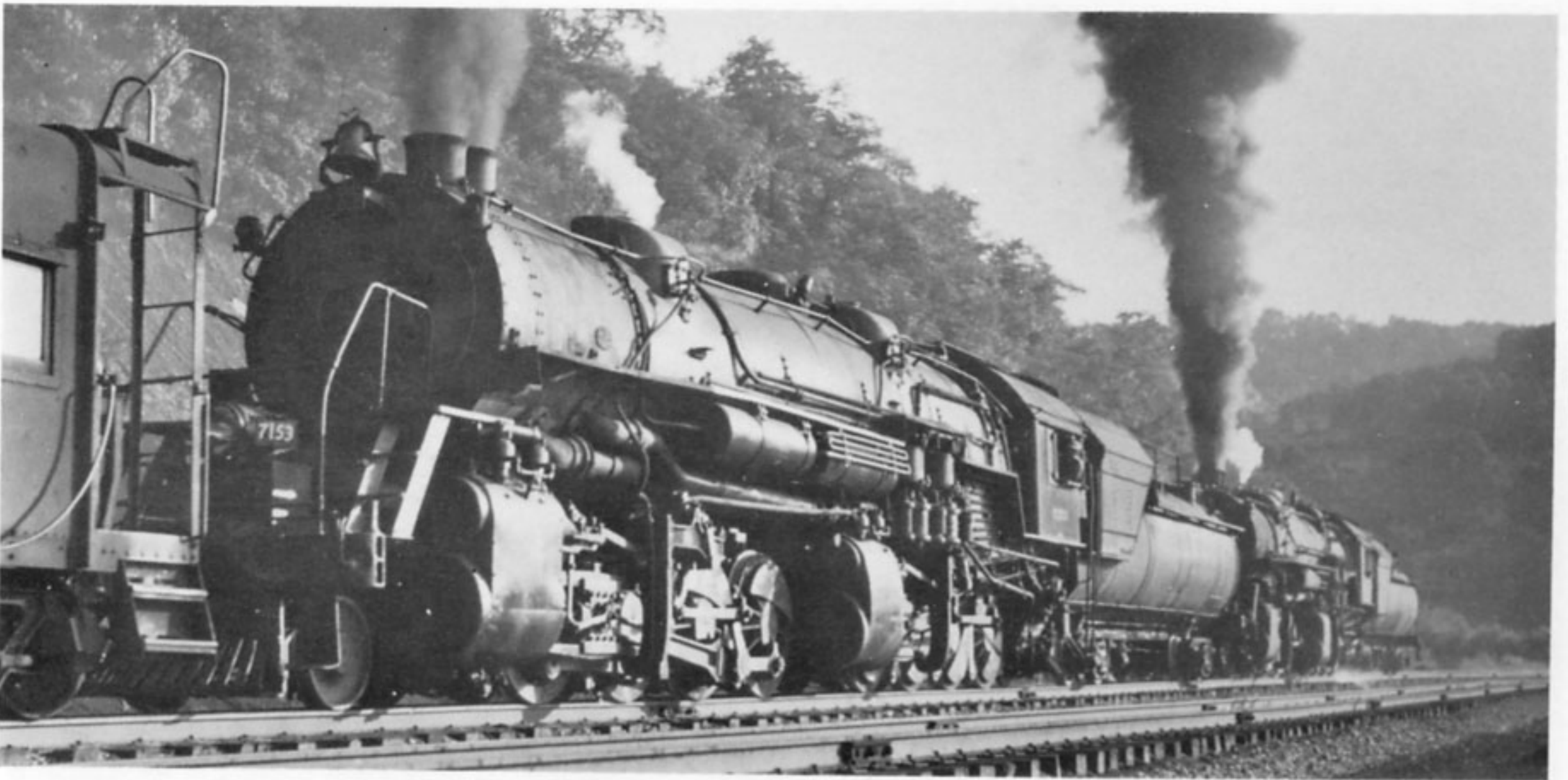
Blasting furiously with the stuttering exhaust from a simple articulated's unsynchronised units, EL-5A 7153 and EL-3A 7133, both 2-8-8-0s, bank EM-1 2-8-8-4 on coal through the wooded hills of West Virginia in July 1949
