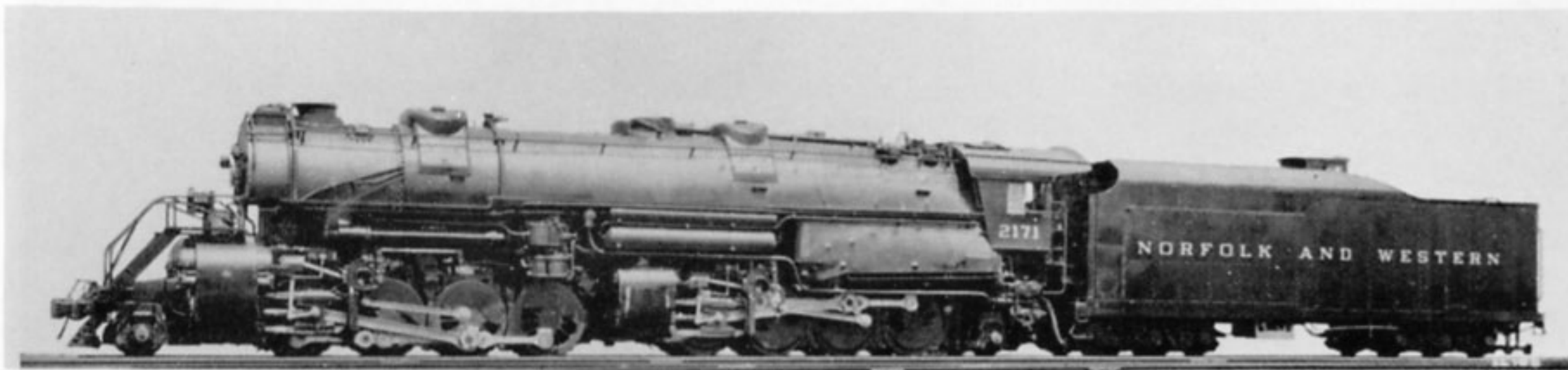
Norfolk & Western's final heavy coal hauler, the Y6b compound 2-8-8-2, heaviest of its type built
