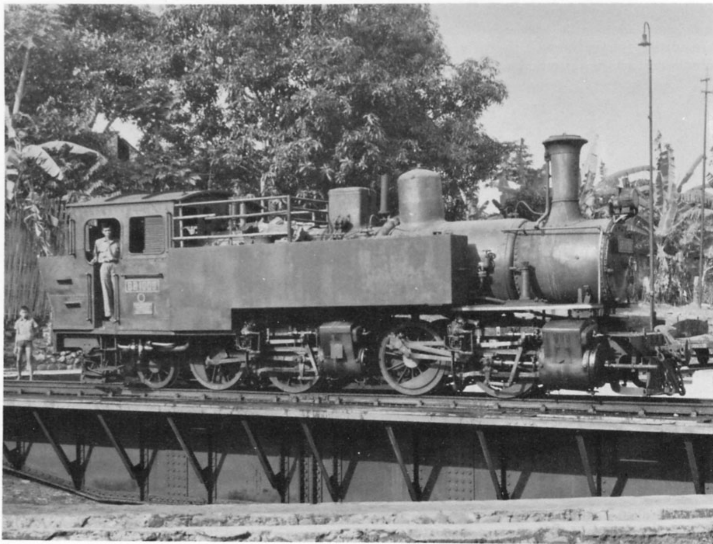
First batch of Mallets for Java's Staats Spoorwegen, a Hartmann 0-4-4-2T, now Indonesian Railways (PNKA) class BB10. Here BB1009 poses on the turntable at Bandjar in October 1970
