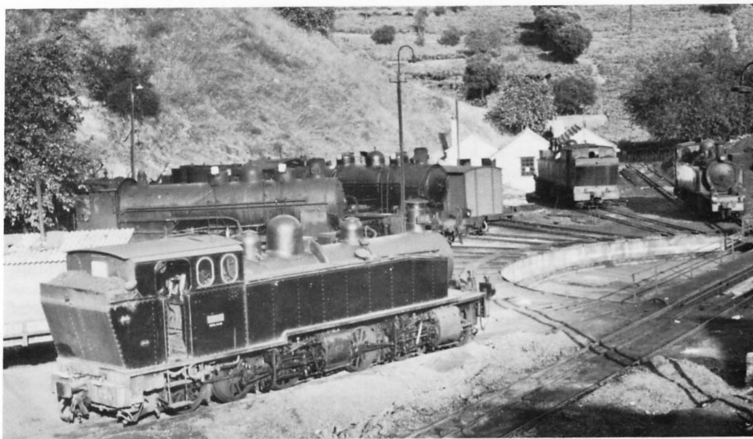
The mixed (5ft 6in and metre) gauge engine yard at Regua, in Portugal's Douro Valley. Three metre-gauge 2-4-6-0Ts cluster round the turntable in 1966, sharing accommodation with two broad-gauge 2-8-0s
