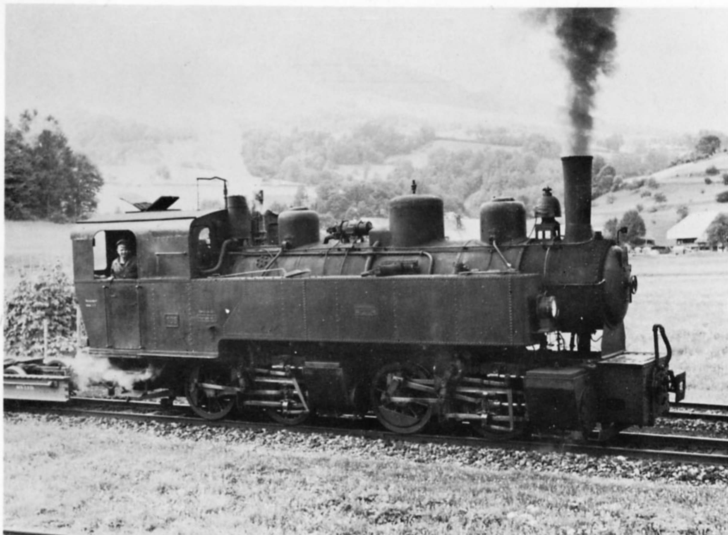
Zell-Todtnau's metre-gauge 0-4-4-0T, No 105, at work in pastoral Baden. This locomotive is now on Switzerland's Blonay-Chamby line
