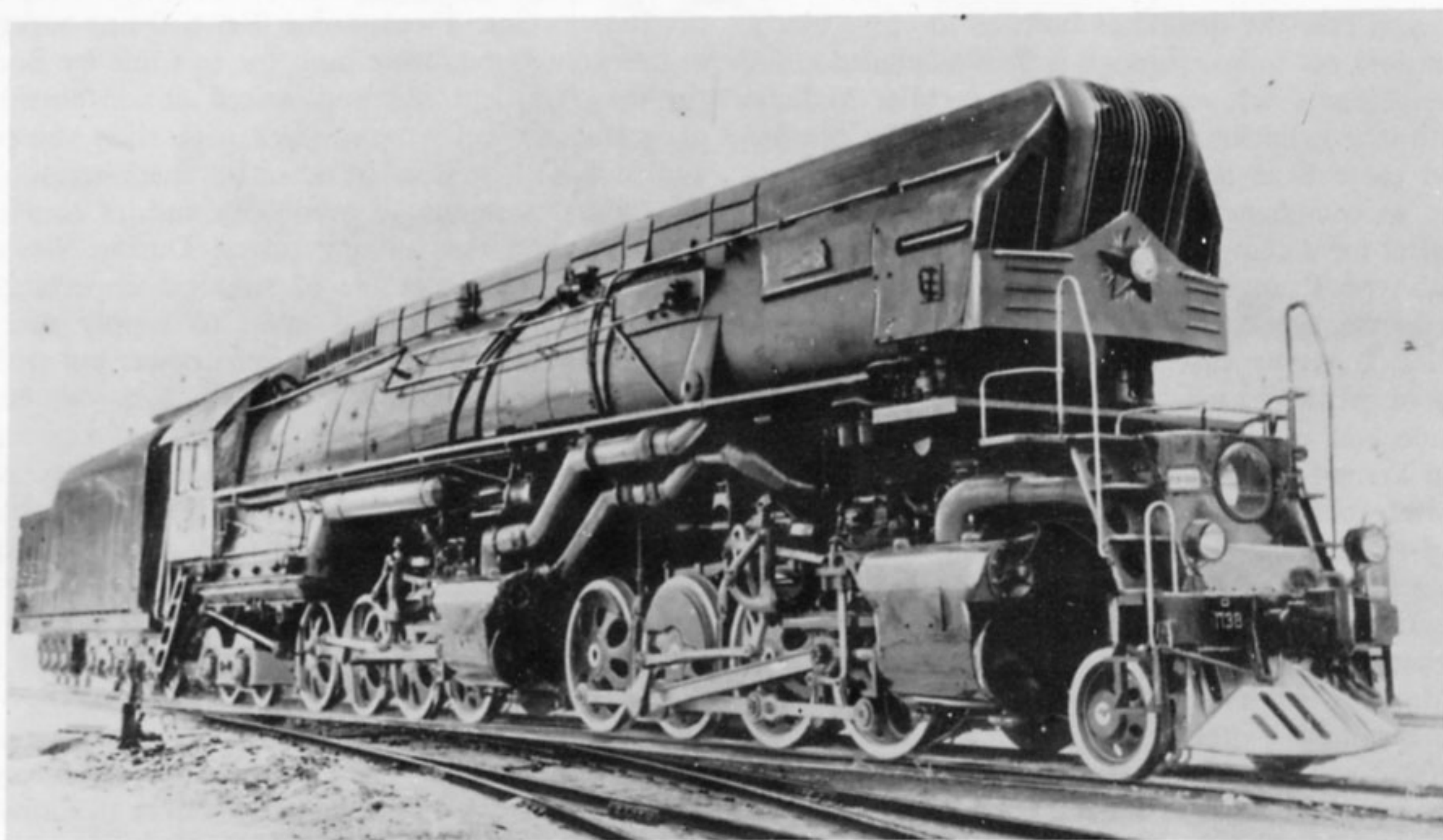
Soviet Russia's two ventures into Mallets culminated in the immense TT38, 2-8-8-4, Kolomna-built in 1954 and spoilt in appearance by the jukebox front end treatment. It has probably been scrapped, though this is uncertain
