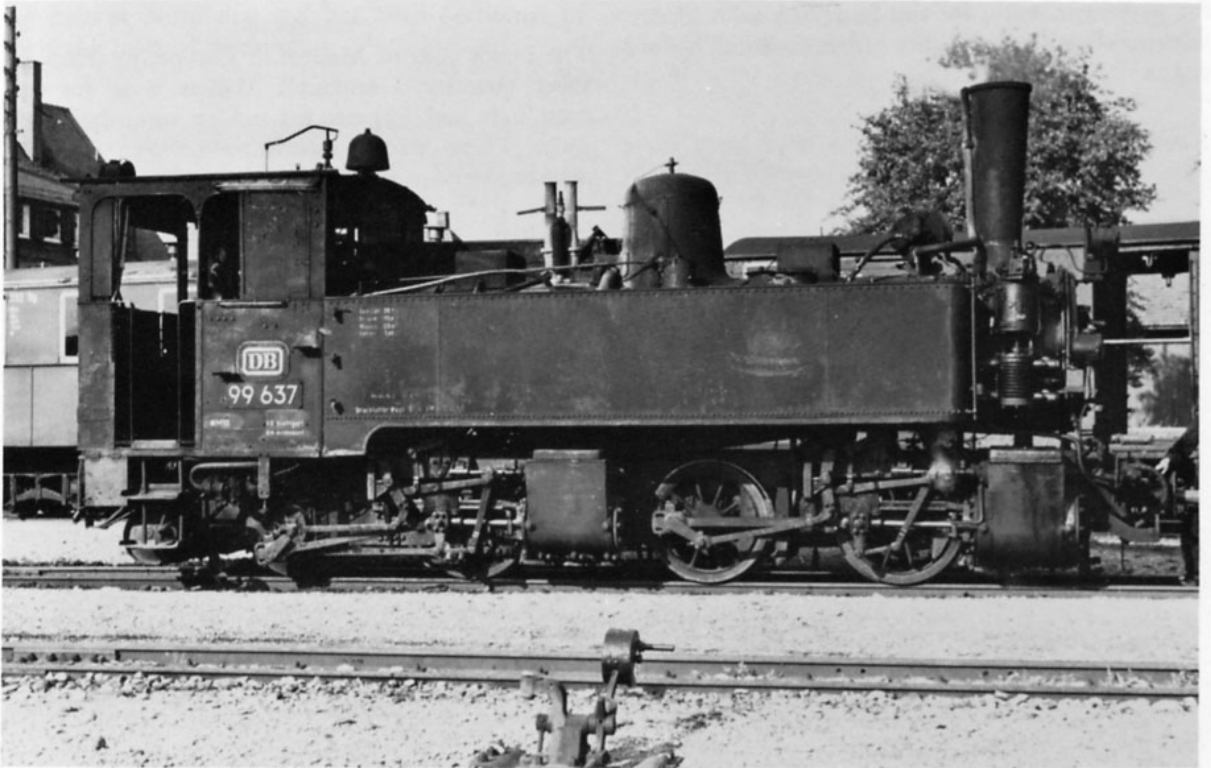
German Federal Railways 0-4-4-0T No 99.637, a 750mm gauge Mallet built for the former Württemberg State Railways, seen at Buchau in 1963
