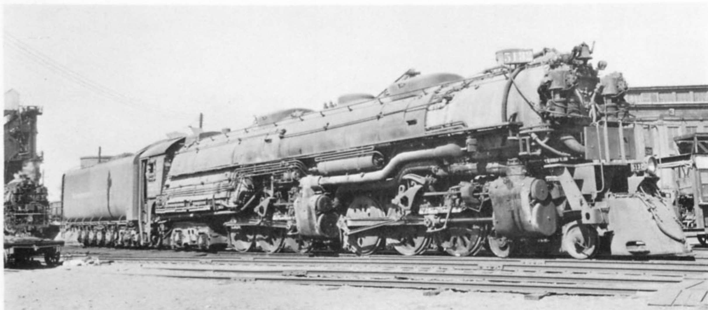
Northern Pacific followed close behind UP with the 4-6-6-4, using giant grates to burn 'Rosebud' lignite. Above, No 5132 from the second series simmers at Missoula, Montana, in September 1952
