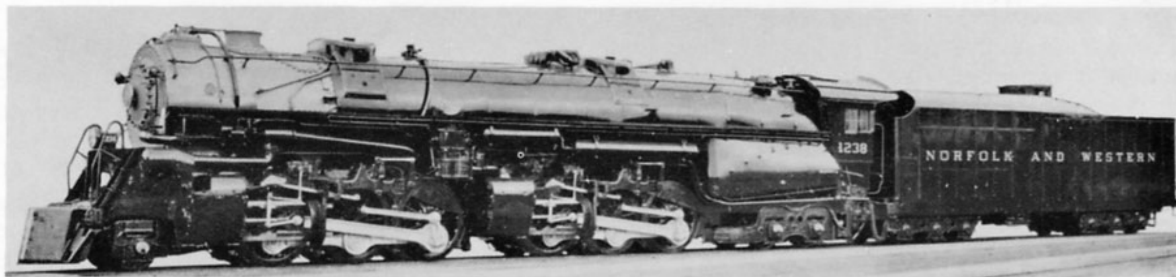
Norfolk & Western's two Mallet designs evolved for high utilisation. An 'A' class 2-6-6-4 simple of the final batch with roller-bearing crankpins
