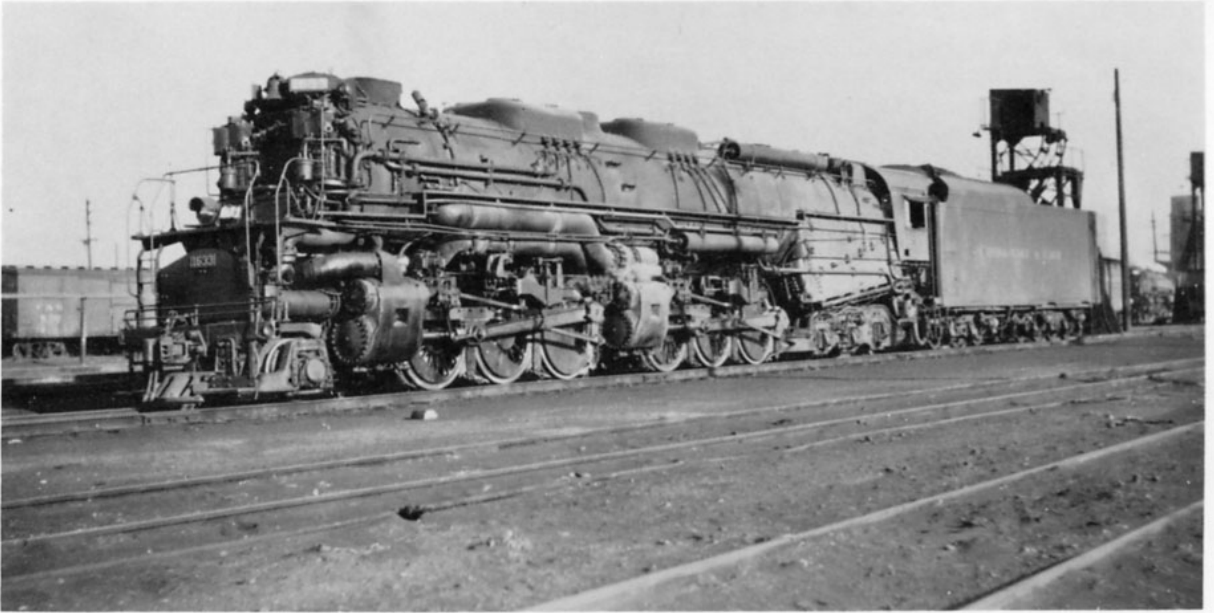
Final development of the six-coupled Mallet was Lima's 2-6-6-6 for the Chesapeake & Ohio, only marginally lighter than Union Pacific's 'Big Boys'. No 1633 of class 'H' stands in the yard at Fulton, Virginia, in September 1940
