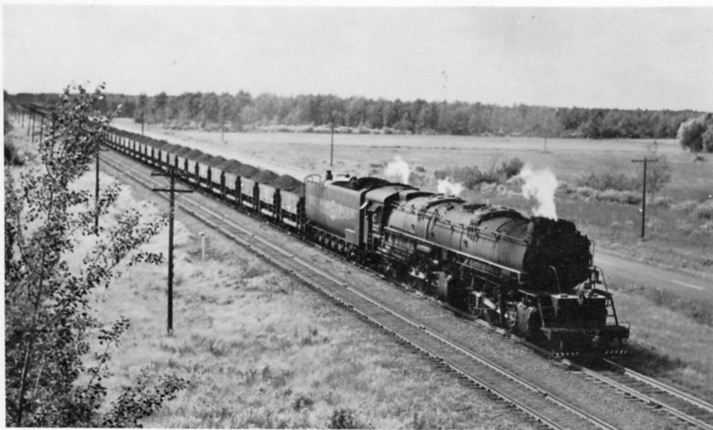
171 bogie hoppers of iron ore, totalling about 15,000 long tons gross, represent an everyday assignment for Duluth, Missabe & Iron Range 2-8-8-4 No 227, seen here ascending Saginaw Hill, Minnesota, in 1959
