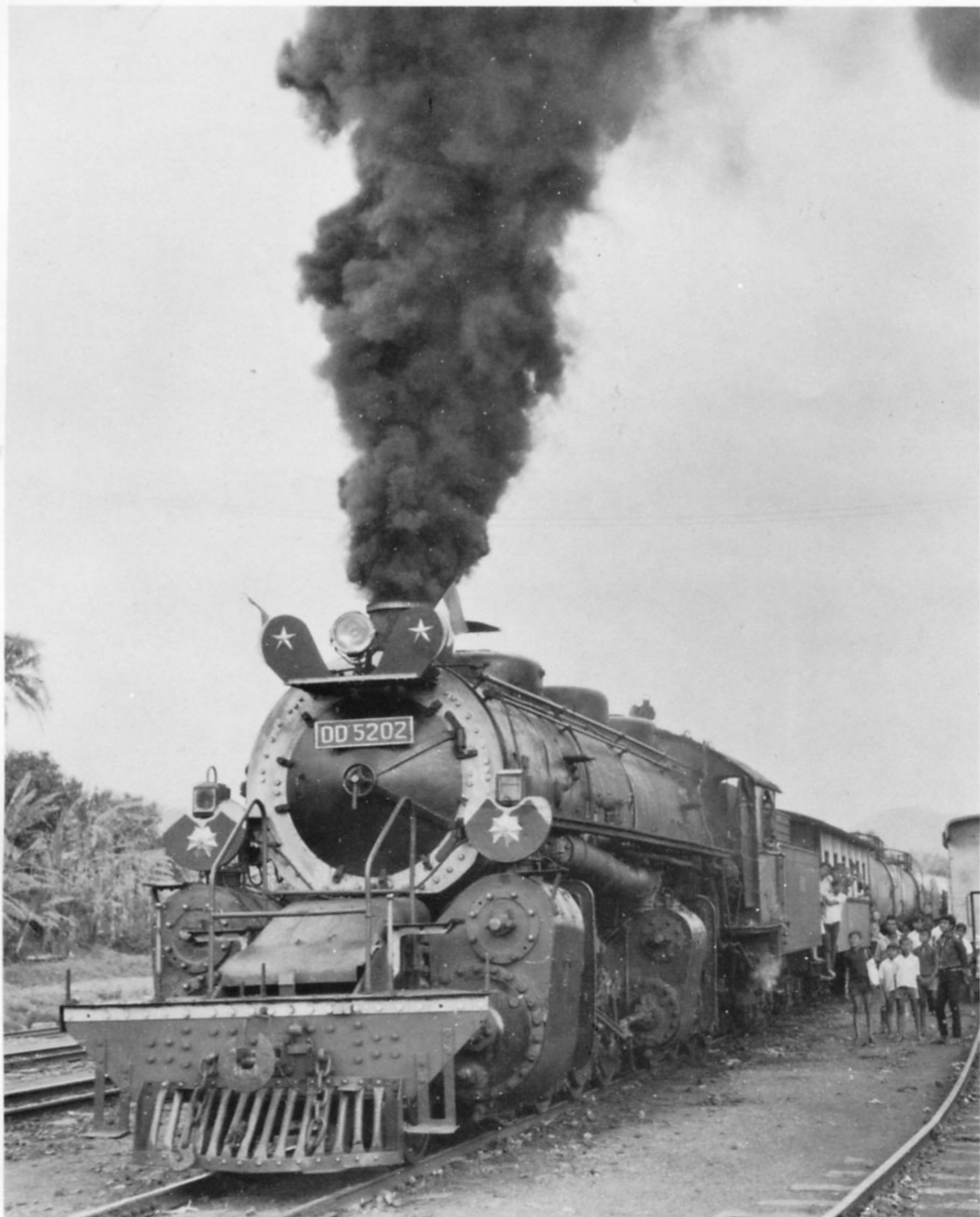
The last mainline Mallets in the world are in Indonesia. Here compound 2-8-8-0 DD 5202 brews up at Tjitjalengka with a mixed train in October 1970
