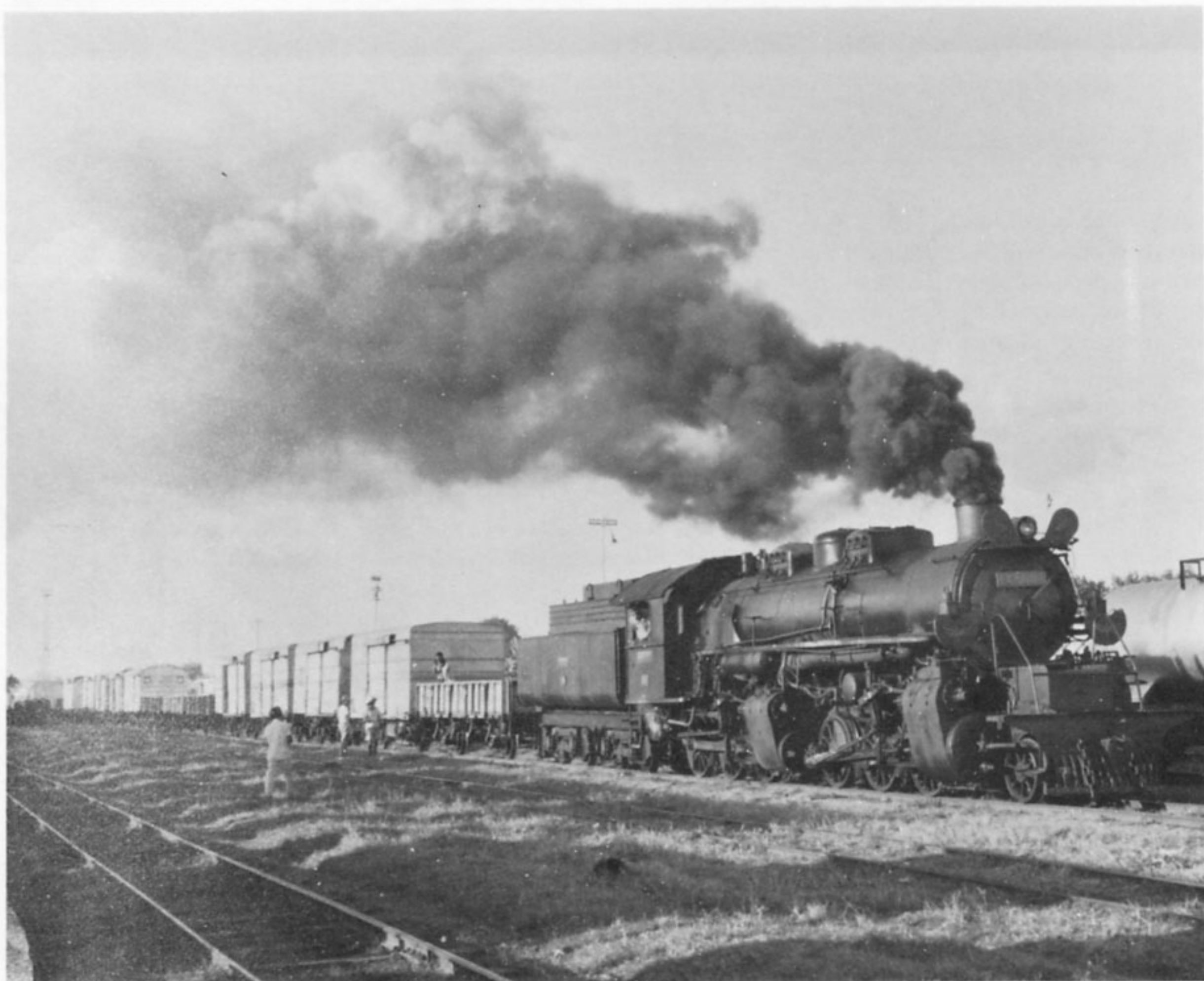
Last tender Mallets for Java, the 2-6-6-0s, now PNKA class CC50, totalled thirty engines, most of which are in stock today. Here No CC5004 prepares to depart from Surabaya (Sidotopo) on a freight in October 1970
