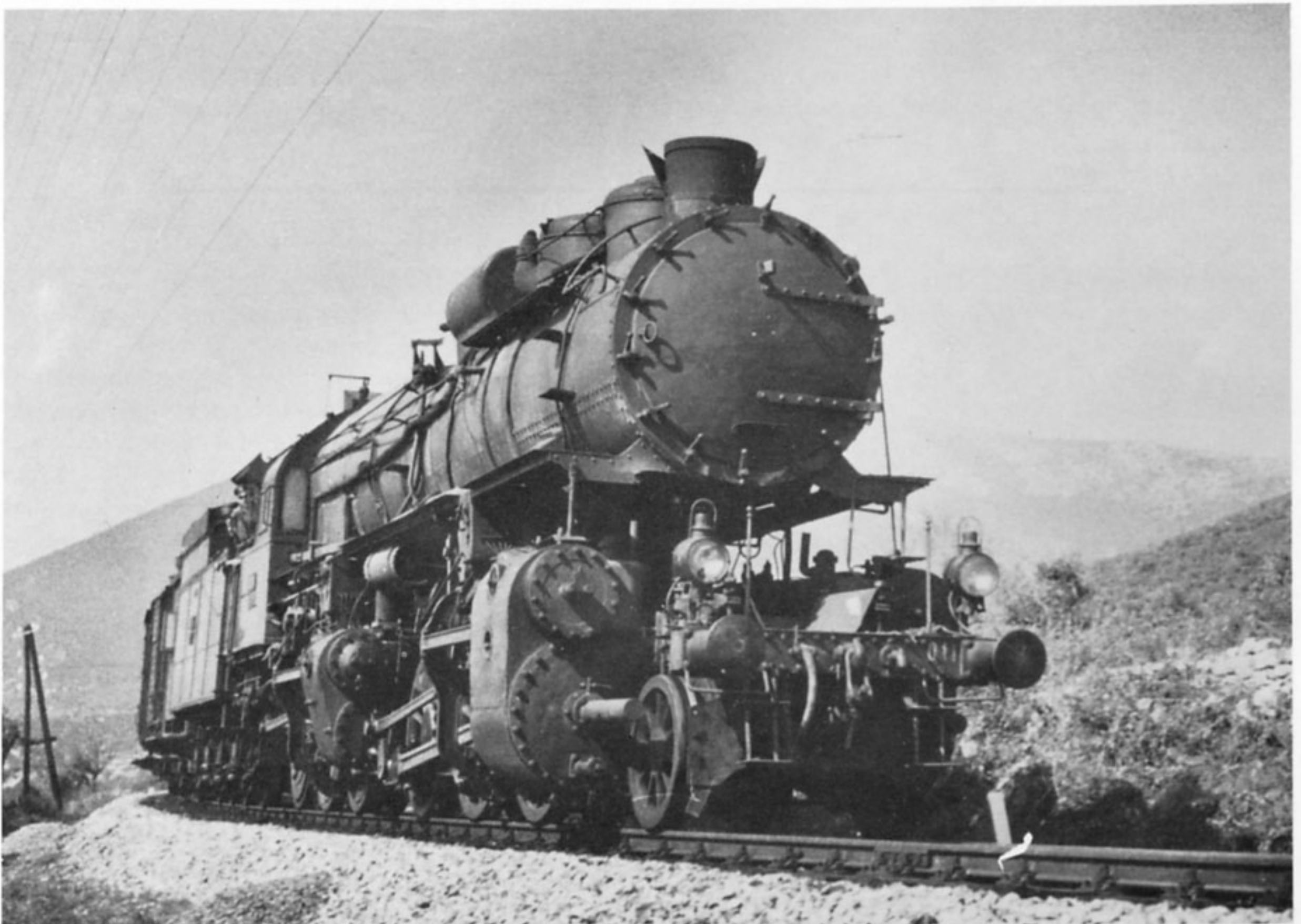
Last mainline duty of Yugoslavia's ex-Hungarian 2-6-6-0s was freight haulage up the Dalmatian escarpment from Split to Knin. Here No 32.011 rolls through Kastel Stari in 1957, the year before diesels
