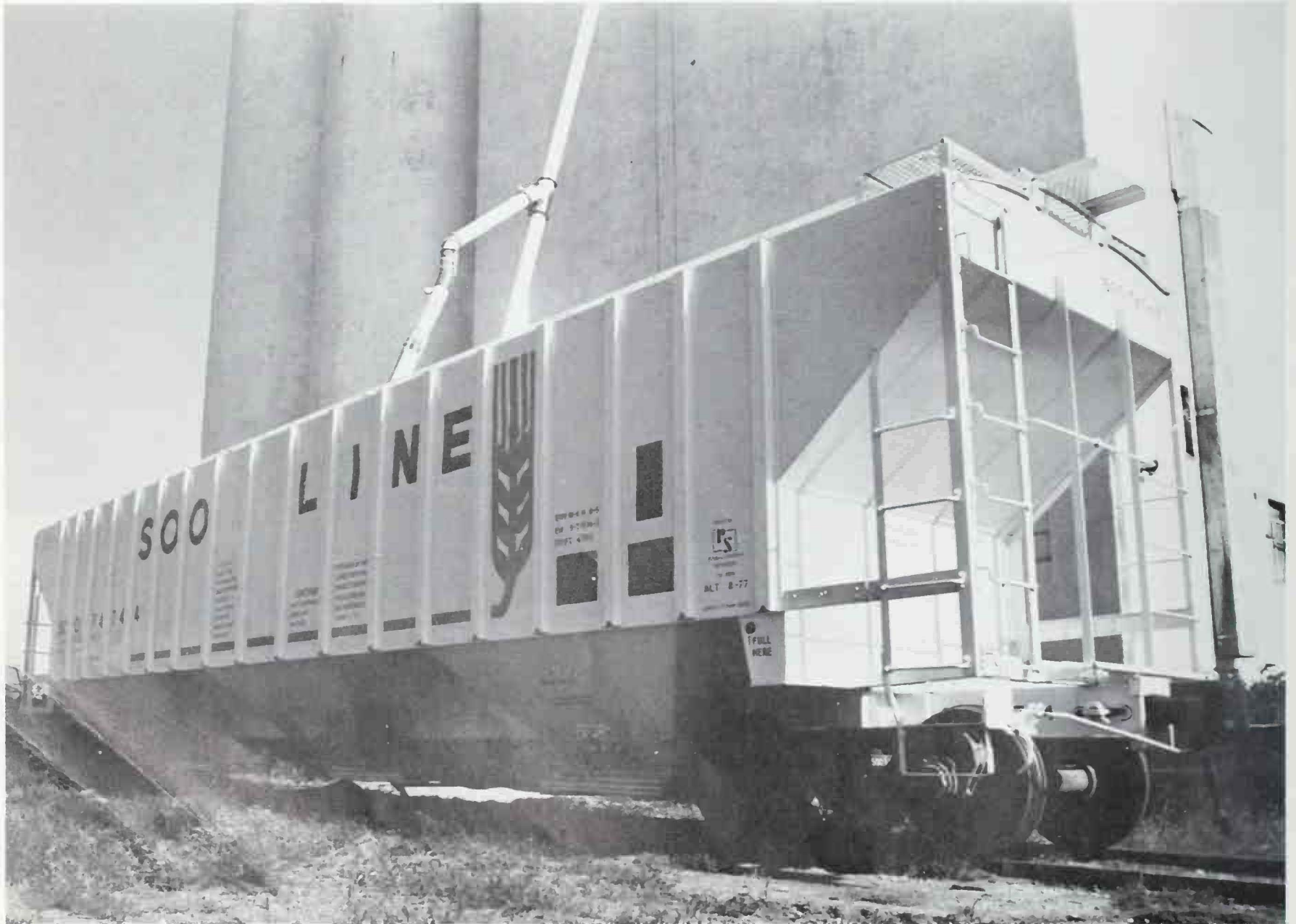
Hopper cars carry loose materials like fertilizer and rock. This car is being loaded with grain.
