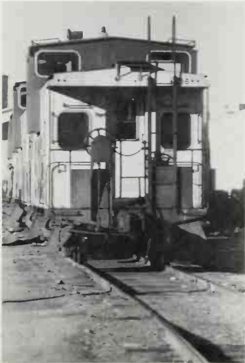
When the caboose wheels are moving, they turn these wheels which operate a generator that provides electricity inside the caboose.
