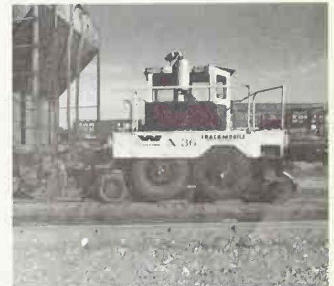
A Trackmobile for moving cars a short distance
