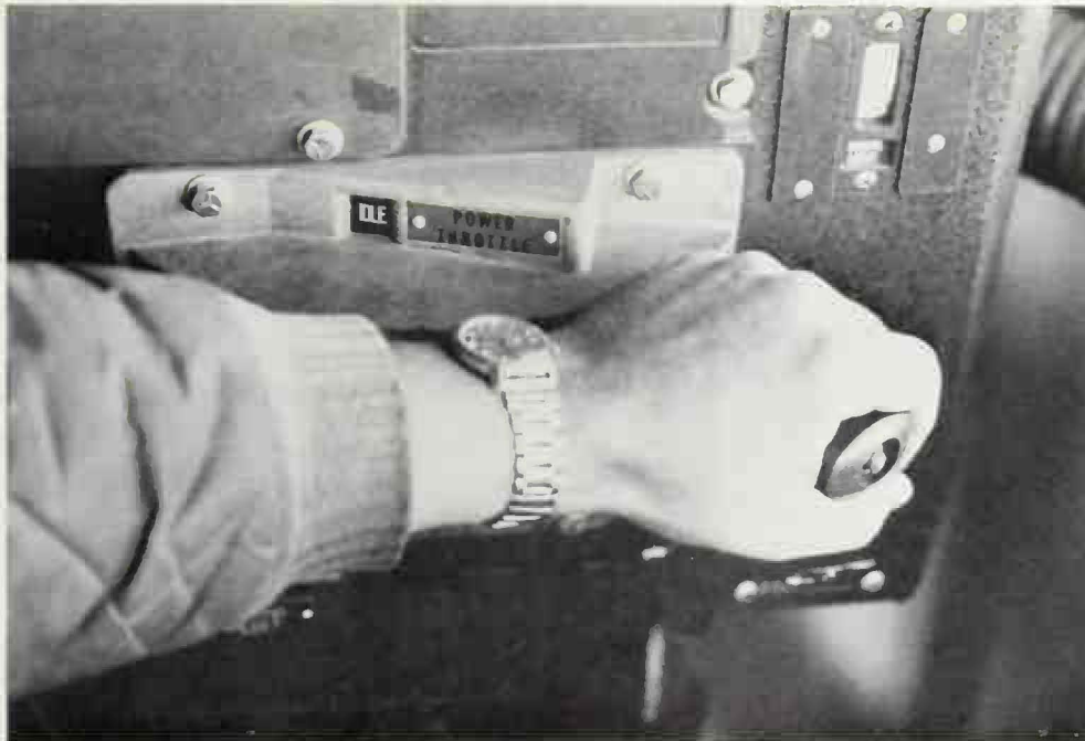
The engine power throttle
