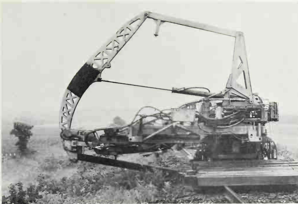
A work machine inserting new ties
