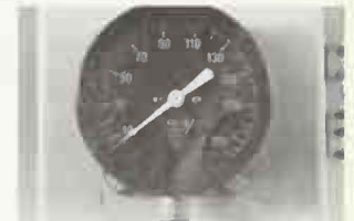
Air pressure gauge for the air brakes
