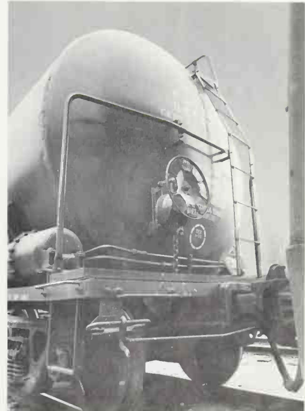
This tank car has a ladder and a brake wheel on the end.
