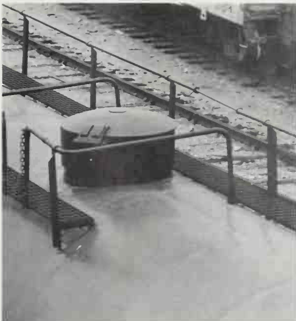
Tank cars are loaded through top hatches and unloaded near the bottom.
