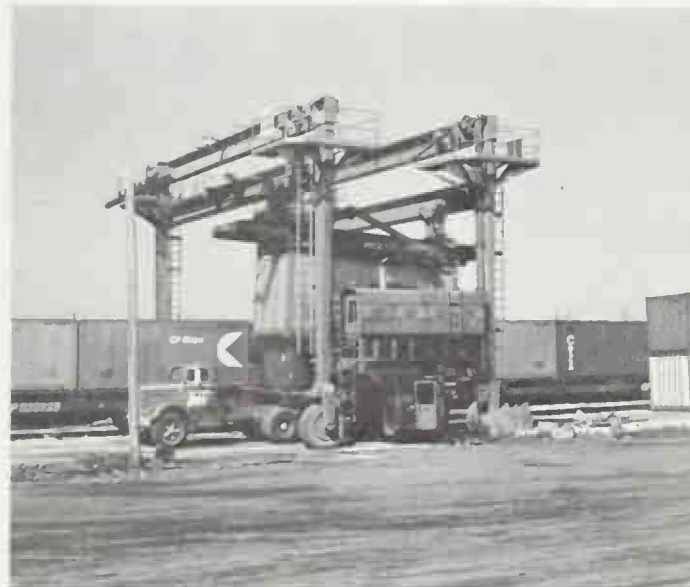
This truck will drive away and leave its whole trailer on the piggyback car.
