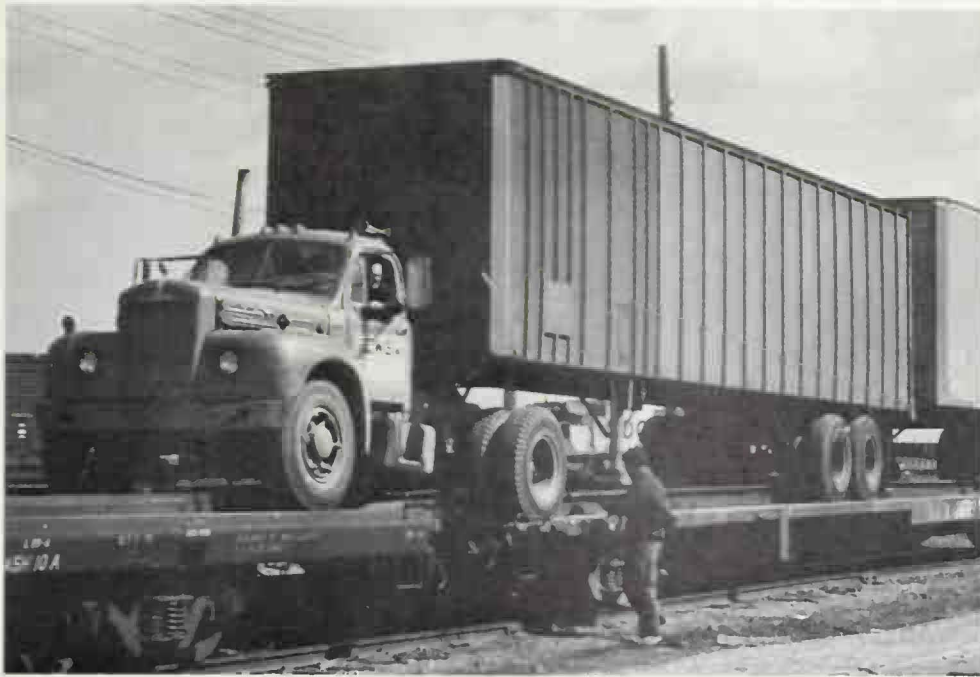
This truck will drive away and leave its whole trailer on the piggyback car.
