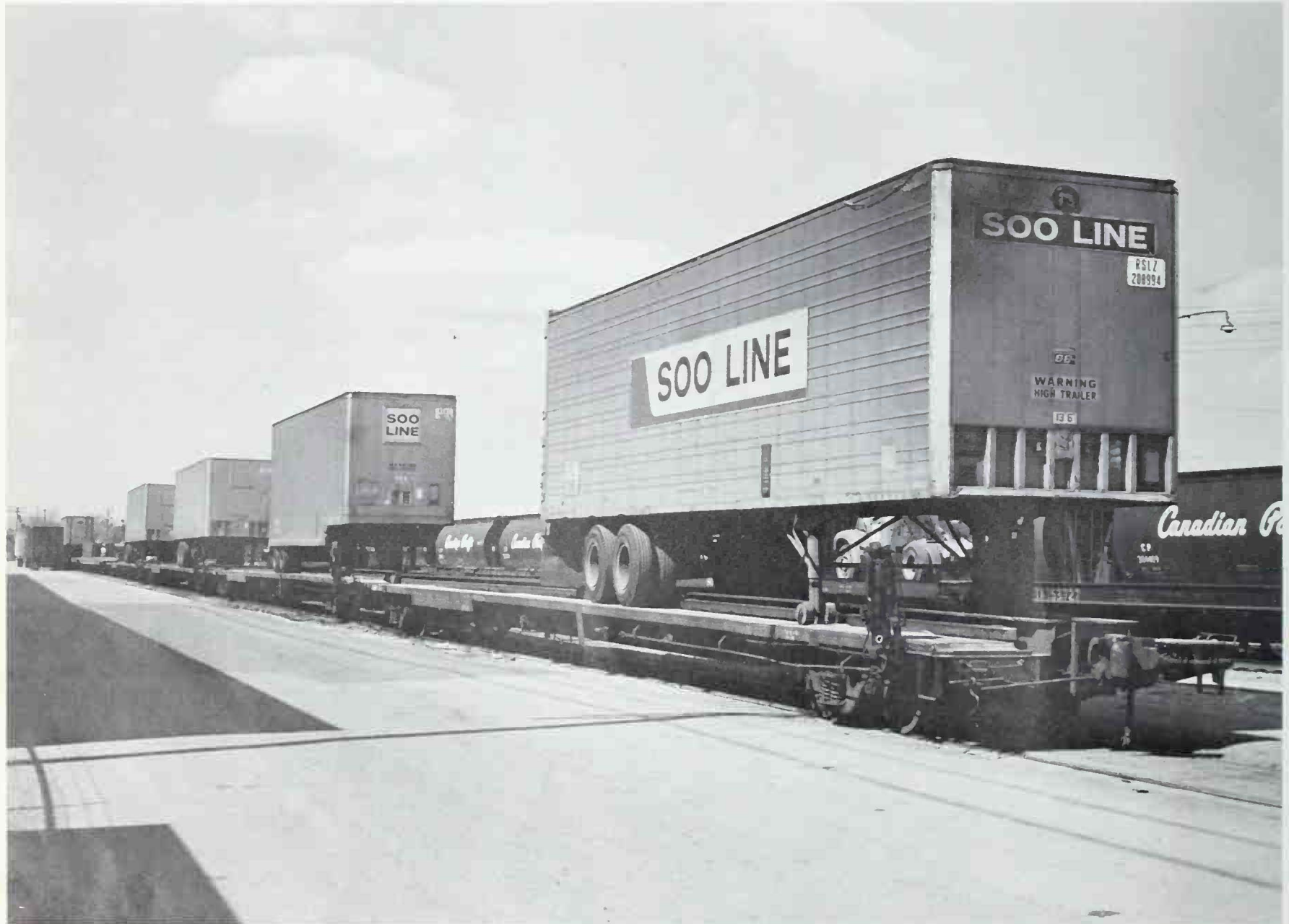
Piggyback cars are longer than flatcars and have special fasteners to attach trailers.
