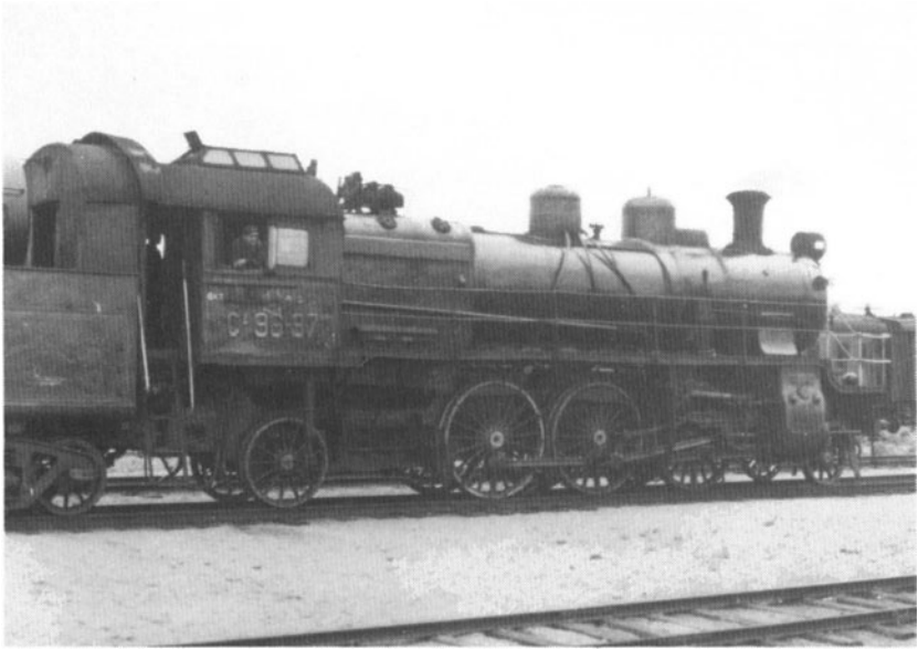
8. An Su passenger locomotive of the first series, one of the early post-revolutionary designs.
