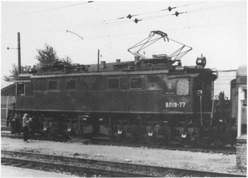
25. The VL19 type, an early Soviet development of the General Electric design.
