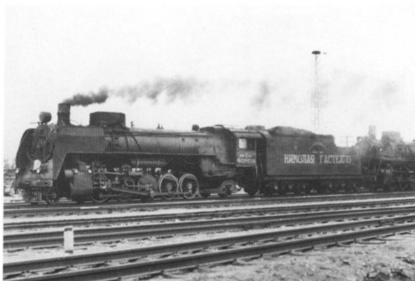
16b. Two FD type locomotives head a freight train near Moscow in 1959. The chimney extension and smoke deflectors were later additions.
