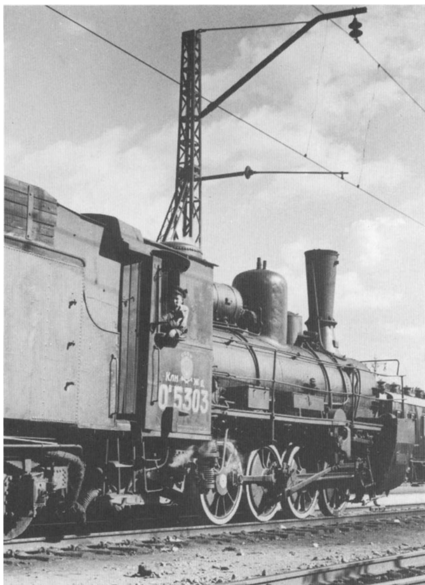
1. A veteran O type freight locomotive still at work in 1959 on an electrified section of the Moscow network.
