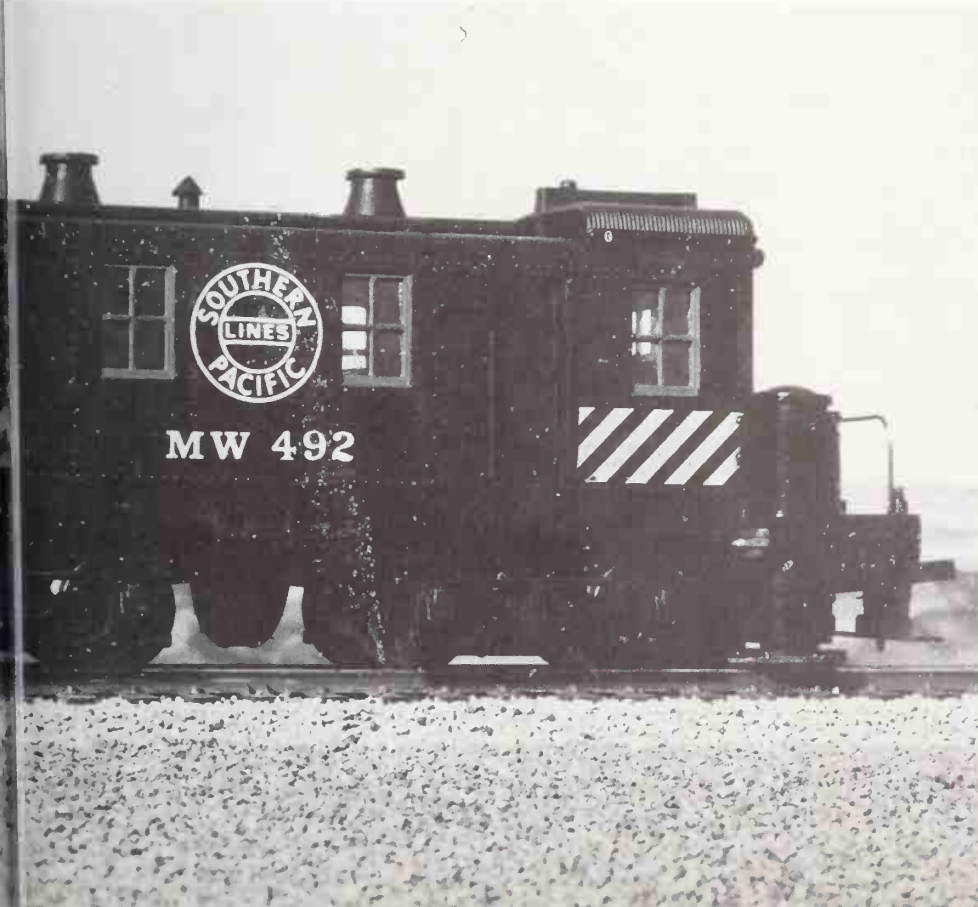
Track-clearing vehicles are now available, disguised as conventional rolling stock and thus able to circulate with a conventional train. The modern alternative is an automatic generator connected between controller and track which deals immediately with any dirt interrupting the current supply.
