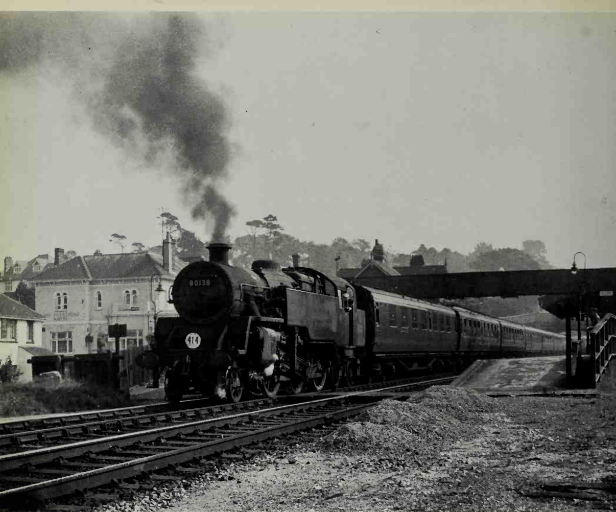
Heavy expresses required help on the severe 1 in 50/60 climb up Parkstone bank. Standard Class '4' 2-6-4T No. 80138 provides powerful rear-end assistance to the 9.25 a.m. from Weymouth as the train hammers through Parkstone station on 20 August 1966.
