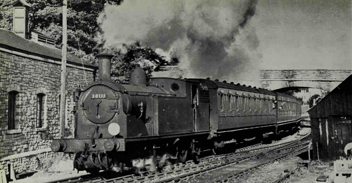
Drummond 'M7' 0-4-4T No. 30111 leaves Swanage with its rake of L.S.W.R. coaches in the evening of 25 August 1956. The ten mile branch from Worgret Junction (a mile west of the market town of Wareham) was opened on 20 May 1885, with one intermediate station at Corfe Castle. An engine for the branch train was stabled overnight in the small shed seen on the left. [G. D. King]
