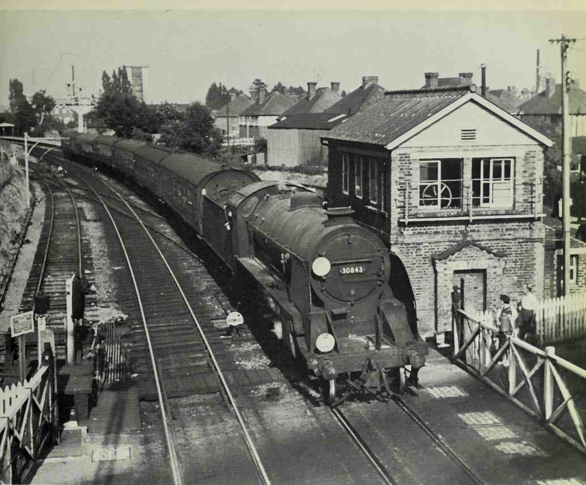
During the summer of 1964, a Feltham 'S15' 4-6-0 was rostered to the 5.10 p.m. Southampton Terminus to Bournemouth (Central) stopper. No. 30843 has the turn on 2 July and is seen pulling away from Totton. The large wheel in the signal box operates the level crossing gates.
