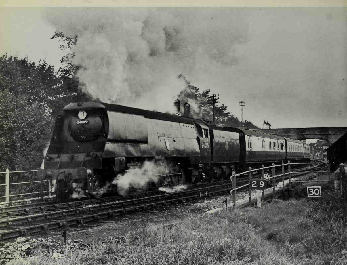
The Saturday morning through train to Waterloo leaves Swanage behind No. 34005 Barnstaple on 8 September 1956. The engine is still largely in its original form, the few modifications include the extended smoke deflectors, angled cab spectacles and the removal of the side sheeting between the cylinders and buffer beam. As the 'West Countries' were notorious for slipping, it is noteworthy that the driver is using the steam sanders to gain adhesion, even on the level start out of the station.
