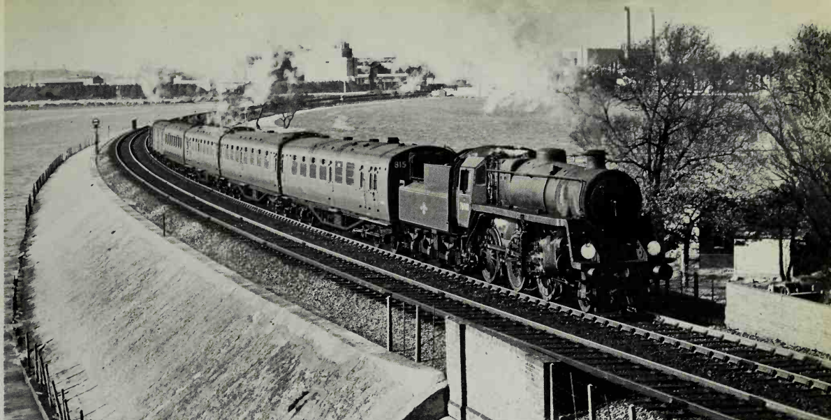
Standard Mogul No. 76008 tackles the 1 in 60 from Poole up to Parkstone with an up stopping train, 13 October 1961. These 2-6-0s, with 5ft. 3in. wheels, were useful replacements for the veteran Drummond types which were withdrawn in the 1950s.
