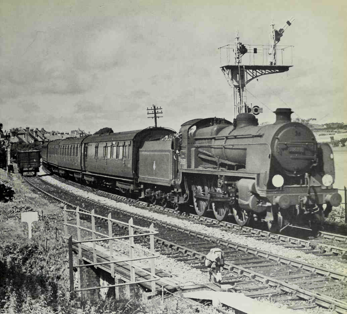
During the summer months, several trains arrived at Swanage from various centres. No. 31633, one of Maunsell's 'U' Class 2-6-0s of 1927, is seen arriving at the attractive Dorset resort with a train from Basingstoke, 27 August 1956. These 6ft. Moguls were ideal motive power for such turns. [G. D. King]
