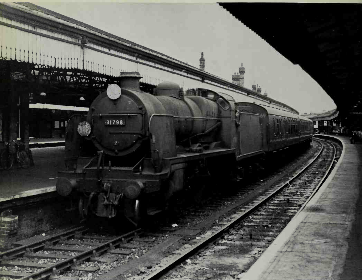
Yeovil (72C) shed had a stud of 'U' Class Moguls for many years. One of these, No. 31798, stands in Salisbury station after working a train from Bournemouth. The flat-sided tender attached to the 2-6-0 has a capacity of five tons of coal and 3500 gallons of water.
