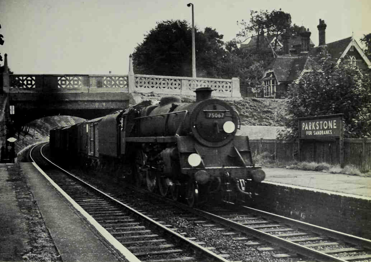
Yet another Standard class at work in the Bournemouth area, this time one of the Class '4' 4-6-0s, several of which were allocated to Eastleigh shed at the period. Double-chimney No. 75067 rolls down the grade through Parkstone with a freight on 25 August 1964. With their 5ft. 8in. wheels, these 4-6-0s were virtually tender versions of the Class '4' tanks, of which No. 80138 on the previous page is an example.
