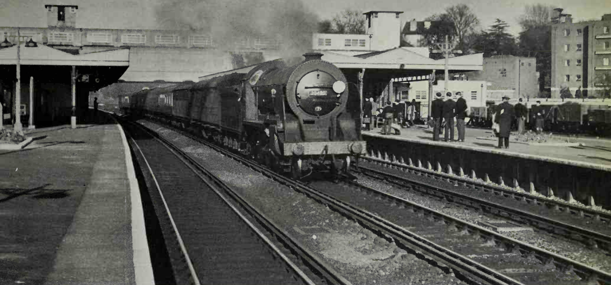
The big 4-6-0s designed by Drummond in the early 1900s were expensive failures. When Robert Urie succeeded as C.M.E. in 1912 his first task was to produce a reliable heavy mixed traffic engine. The result was the first 'H15', numbered 30482 in BR stock, which is seen running past Surbiton on the down through road on 22 March 1957. Nos. 482 to 491 were always known as the 'Chonkers', a nickname which suited them admirably. [A. R. Butcher]
