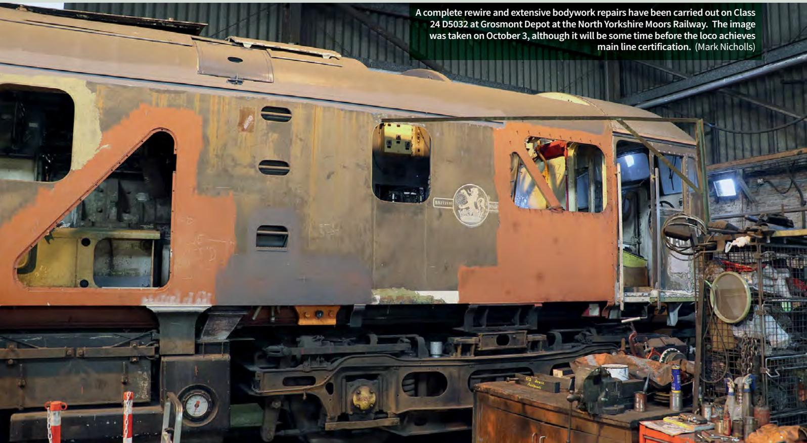
A complete rewire and extensive bodywork repairs have been carried out on Class 24 D5032 at Grosmont Depot at the North Yorkshire Moors Railway. The image was taken on October 3, although it will be some time before the loco achieves main line certification. (Mark Nicholls)
