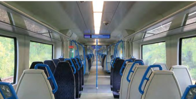
Four-across seating and wide walk through carriage connections are the hallmark of the Siemens Class 700 fleet used by GTR. The seats are not particularly wide, to allow for more standing passengers, and they are quite firm, but the design gives a feeling of space and the overhead information screens can show where more room is available within the train. (Wikimedia Commons/RM)
