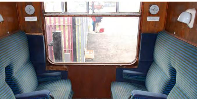
The interior of a typical Mk 1 Second Class compartment, configured to seat six. The armrests could be raised to seat one extra person on each side, but on dedicated commuter rakes the arm rests were removed, permitting eight seats per compartment as standard. (Wikimedia Commons/Hugh Llewelyn)
