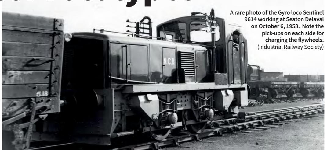
A rare photo of the Gyro loco Sentinel 9614 working at Seaton Delaval on October 6, 1958. Note the pick-ups on each side for charging the flywheels. (Industrial Railway Society)
