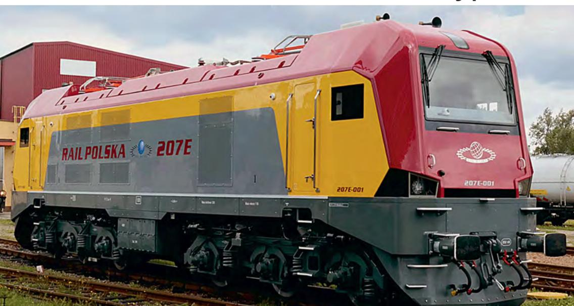
The rebuilt M62M diesel is now a Type 207E electric loco. (Rail Polska)
