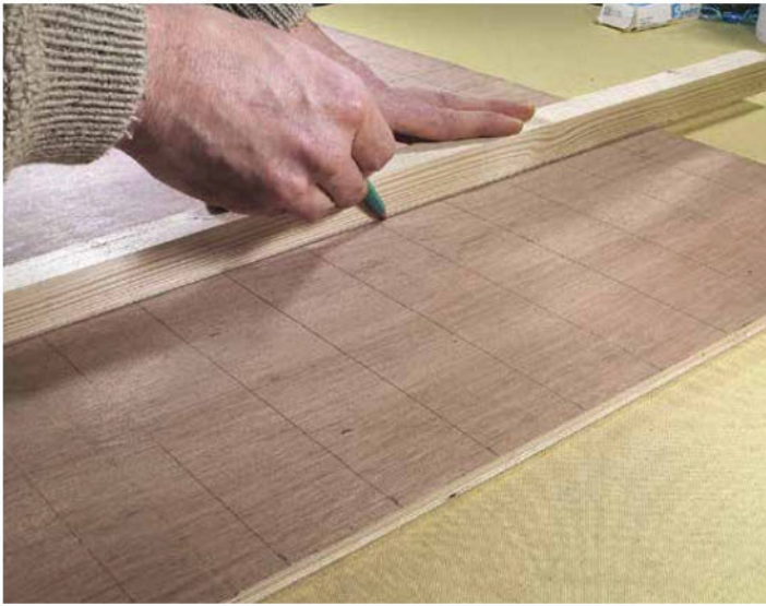
The grid helps to transfer at the right scale all the drawing lines onto the board.
