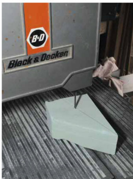
The polystyrene is cut with a saw.
