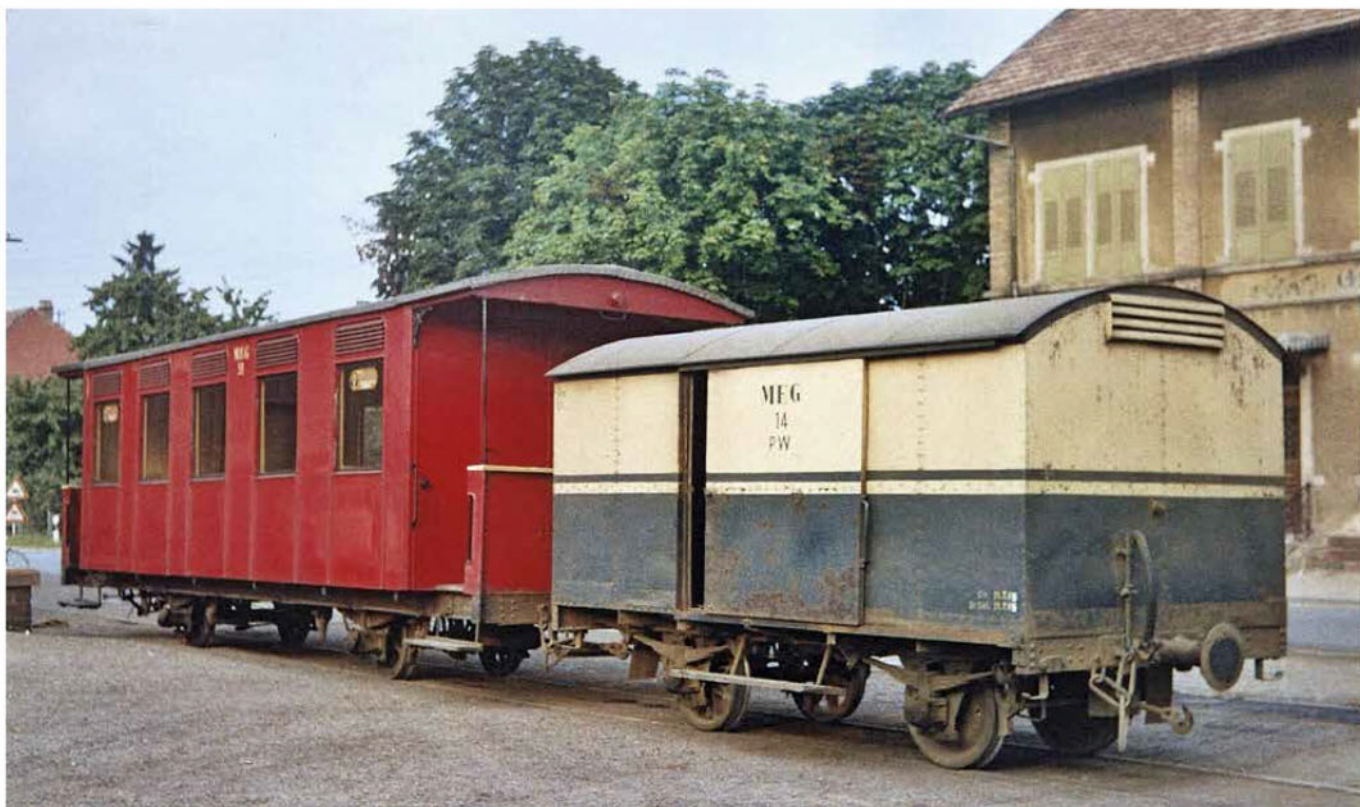
Stock awaits a railcar outside Freistett station (km 17), Ci 59 carriage built by the Compagnie des Tramways de Strasbourg 1914 and PW 14 van, built by MEG 1935. (14 August 1965, J.-L. Rochaix)
