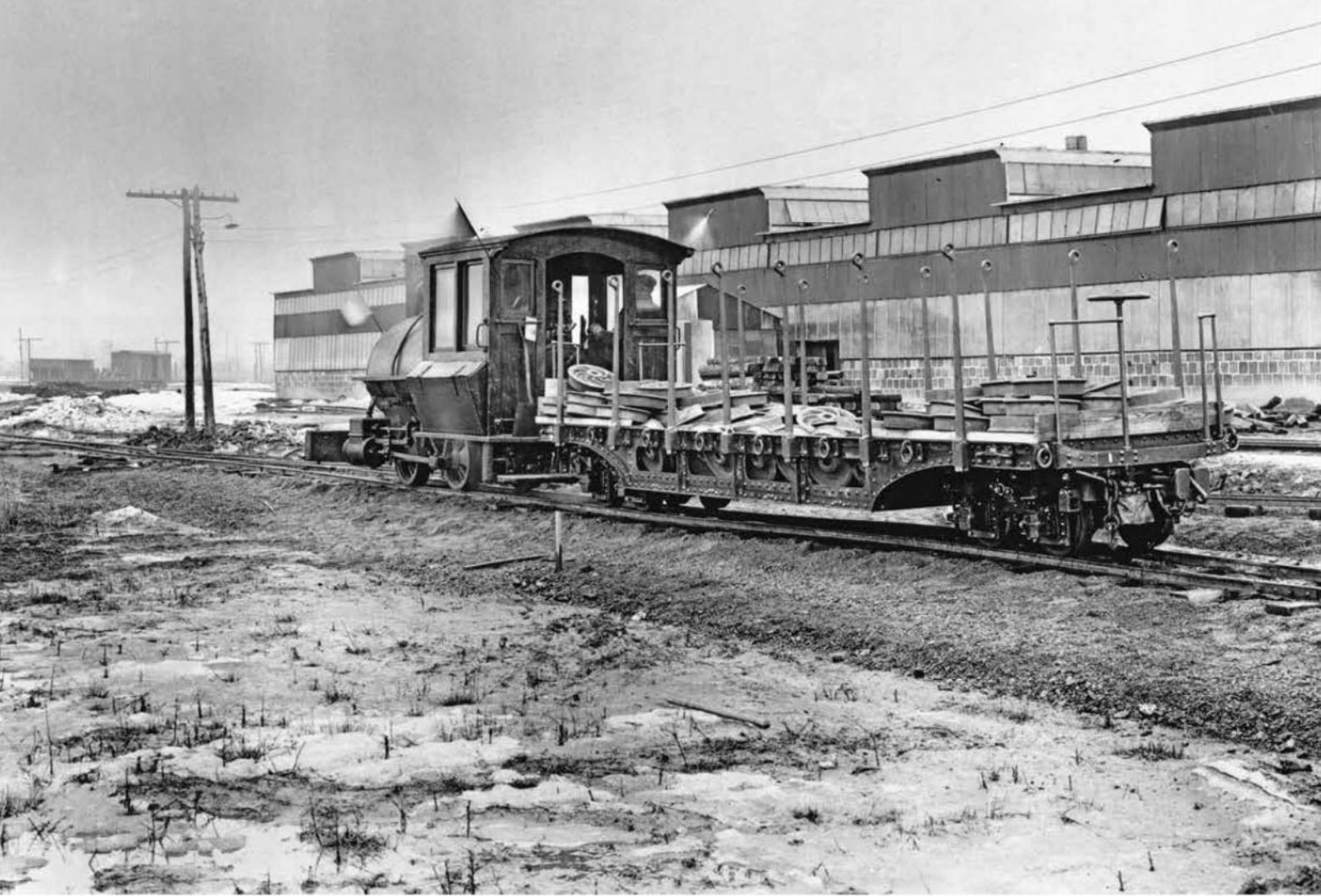
While locomotives were being built in the United States, the French army ordered a large quantity of 1888 type platforms from Canada. Hence this unusual combination of a Davenport 0-4-0 saddle tank with a Péchot wagon on the sidings of the National Steel Car company in Hamilton, Ontario. < https://www.flickr.com/photos/colinchurcher/Library and Archives Canada PA208472 >
