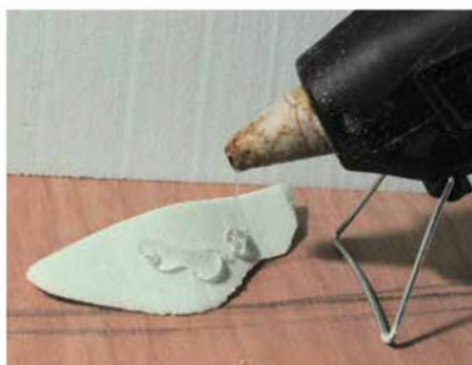
The pieces are glued together with a generous coat of hot melt adhesive.
