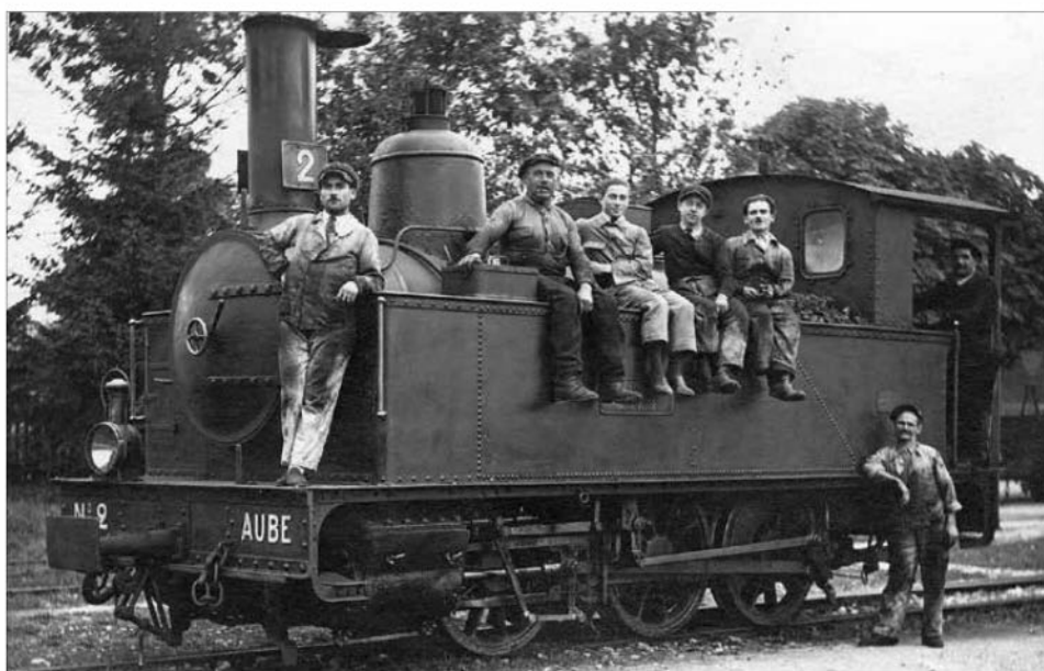
Pinguely locomotives are fairly distinctive: an angular outline, a conical shaped steam dome and a straight running plate are typical features. This one belongs to the 102 type and was supplied to the Tramways de l'Aube system (n° 103/1901). (DR/Coll. É. Mandrillon).
