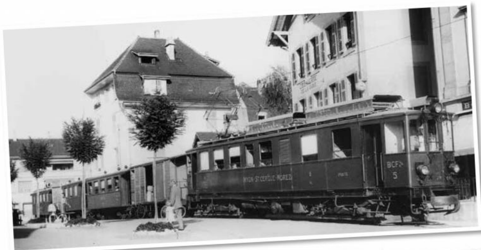
With motor-unit BCF 5/4 5 in charge, a mixed train is awaiting departure on the station square at Nyon, note the short four-wheeler carriages. The motor-unit is already on the gradient leading down under the CFF tracks. The carriages are still of the four-wheeler type. September 1948. Photo J. Chapuis.
