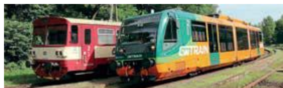
GW Train has a fleet of second-hand Duewag/Siemens-built RegioSprinter lightweight DMUs and has bought 10 more for the new contract. GW Train-liveried unit No. 654 013 is seen next to an old ČD Class 810 two-axle DMU at Krásný Jez on July 9.
