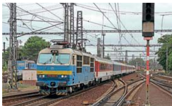
The Class 350 dual-voltage electric fleet passed to Slovakia when Czechoslovakia broke up into different countries in 1992. No. 350 004, repainted in original Czechoslovak Railways (ČSD) livery, arrives at Kolin on June 26, 2016 with a Žilina to Prague express service.
