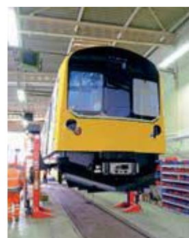
The first production Vivarail 'D-Train' No. 230002 on jacks inside the company's Long Marston workshops. Vivarail has incorporated a number of modifications to this unit, learnt from experience with the prototype. BEN JONES
