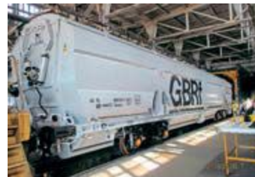
One of 50 Romanian-built high-capacity hoppers being leased by GBRf for the new Port of Tyne to Lynemouth biomass flow. GBRf
