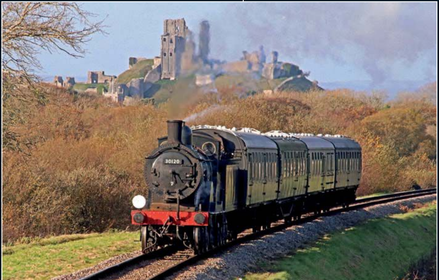
Drummond 'T9' 4-4-0 No. 30120 made a welcome return to steam on the afternoon of November 23 after cylinder repairs at the Swanage Railway. The 'Greyhound', which had not run since arriving in Dorset in July, works a loaded test train at Corfe Castle. ANDREW P M WRIGHT
