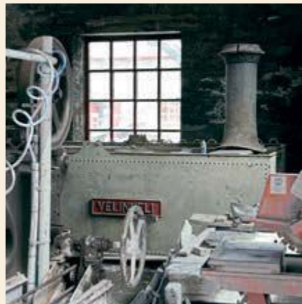
Above: The remains of the Padarn Railway's 4ft-gauge, 1895-built Hunslet 0-6-0T Velinheli . It was dismantled in 1953 for an overhaul, which was never completed, with the side tanks (one with a nameplate) and chimney being stored in the slate museum at Gilfach Ddu.
