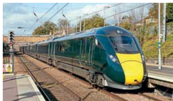
Destined for use on the GWR and running on diesel power, new nine-car Hitachi Class 802 No. 802101 bi-mode set passes Biggleswade returning to North Pole depot on November 6, having visited Hitachi's Doncaster depot. ALISAIR ANDERSON
