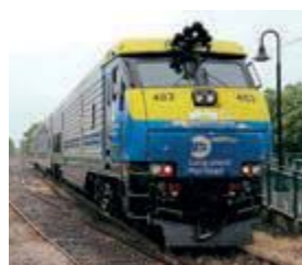
LIRR EMD-built DE30AC diesel loco No. 403 is seen at Greenport on June 16. This push-pull shuttle service connects at Ronkonkoma with the electrified line to Hicksville, which is being double tracked as part of the programme. KEITH FENDER
