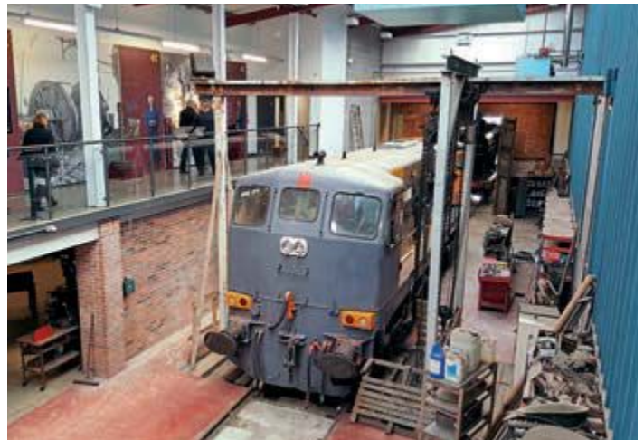
Looking down from the viewing gallery in the Dunleath Workshop as GM Class 141 No. 142 receives attention over the wheeldrop. The gallery runs through almost 180° and is complete with interpretive displays. GARY BOYD-HOPE
