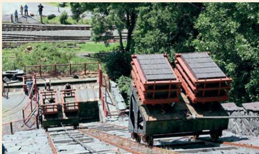
The restored V2 'tanc' incline provides an additional attraction above the throat of Llanberis Lake Railway's Gilfach Ddu station. Originally, the weight of the pair of descending loaded slate wagons would pull the pair of unloaded wagons back up, the speed being controlled by a brake on the winding drum at the top of the inclined plane. Demonstrations of how the incline worked are now handled by an electric motor (the loaded wagons have to go back up nowadays).
