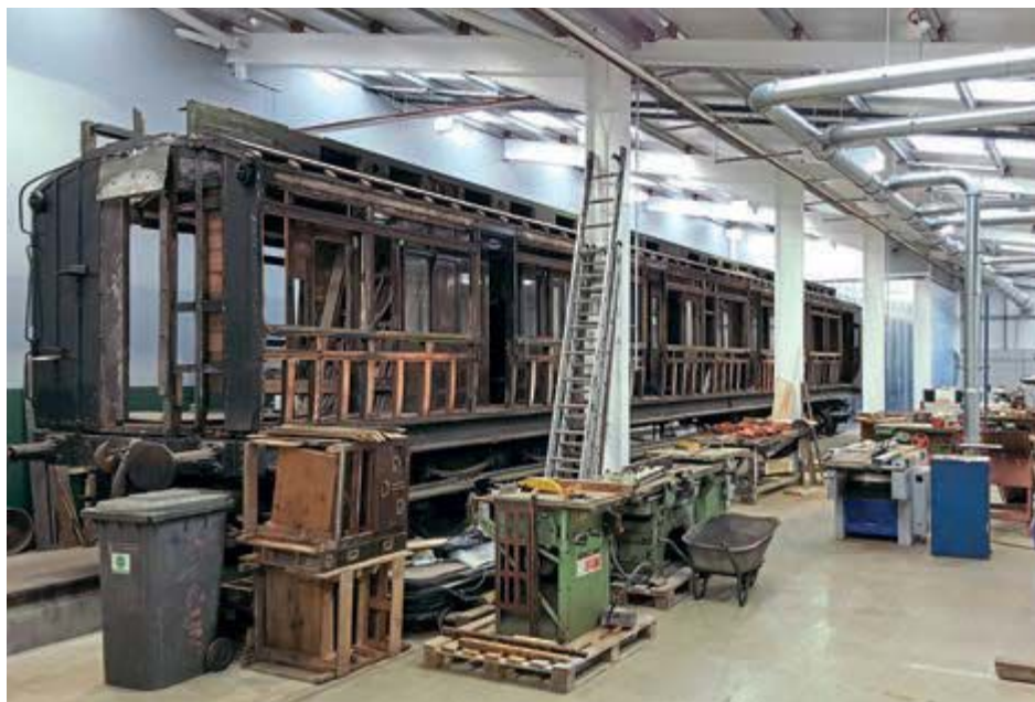
The new Carriage Shed extension incorporates a publically viewable workshop, where work is currently underway on the society's GSWR 12-wheel clerestory brake first/third No. 861. GARY BOYD-HOPE
