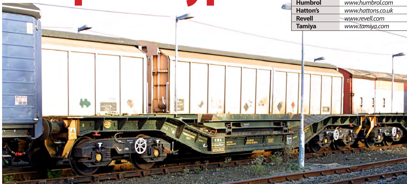
Originally built in 1942-1944, a total of 32 Warwells were refurbished with Gloucester bogies and air brakes in the mid-1970s and there was further rebuilding 20 years later. This image gives a good idea of the extended support ribs underneath the widened end decks and the relative levels of the new support cradle and the end platforms. John Turner/53A Models of Hull Collection.
