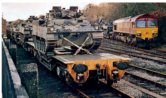
A train of Warwells being marshalled at Haverfordwest. The degree of overhang is obvious from this angle. The effect of parking a 1:76 scale Warrior on a 1:76 scale Warwell wasn't as grotesquely exaggerated as I'd feared, but you can clearly see why the cradle is necessary for the tracks to clear platform edges. R. Weatherall.
