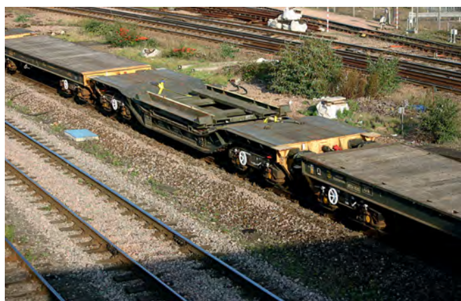
An invaluable top-down shot of MODA 95525 at Millbrook on 13 October 2011, showing sufficient detail of the structure of the support cradle to enable me to estimate dimensions and build a couple in 4mm scale. Martyn Read.
