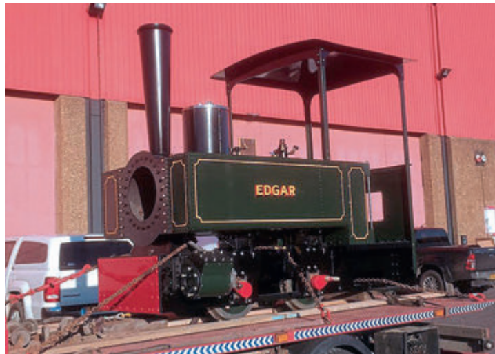
Britain's latest new-build, Decauville 0-4-0T Edgar , which was built by the engineering arm of Scarborough's North Bay Railway. WMRC
