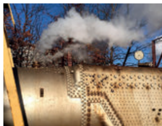
The boiler of 9F 2-10-0 No. 92134 passed its steam test on November 23. 92134
