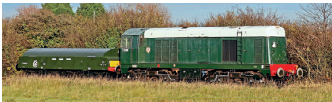
English-Electric Type 1 Bo-Bo D8098 with diesel brake tender No. B964122 built by a group of engineers from Railway Vehicle Preservations, is seen at Woodthorpe on November 19. PAUL BIGGS
