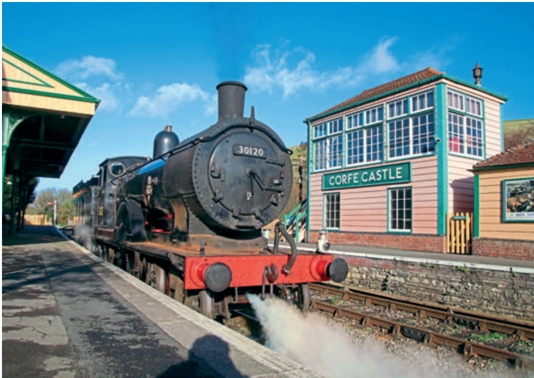
LSWR T9 'Greyhound' 4-4-0 No. 30120 lets off steam at Corfe Castle during a test run on the Swanage Railway on November 23. Extensive repairs have been carried out at Swanage to one of the 1899-built National Collection locomotive's cylinders after fears were sounded that it might not steam again. For so long based on the Bodmin & Wenford Railway, its late July move to Swanage could now last much longer than expected and could even be made permanent. ANDREW PM WRIGHT
