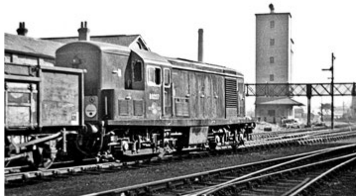
The end is near: D8227 passes the closed Halstead station in 1965, shortly before freight traffic ceased and the track was lifted. The Class 15 Bo-Bo was designed by British Thomson-Houston and built by Clayton Equipment Co in May 1960 and withdrawn in September 1968. The photographer was standing on what is now the location of the new Lidl store. The diesel is seen passing the original offices of the Colne Valley & Halstead Railway, and in the background is the chimney of a Courtauld's mill, a grain silo, and a footbridge crossing over the tracks, all now gone. R HUTLEY
