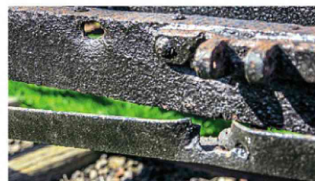
The frames of No. 2572 (before restoration) showing shrapnel damage from First World War activities. The frames have had new strengthening members added but still retain this damage on view. DAVID ENEFER
