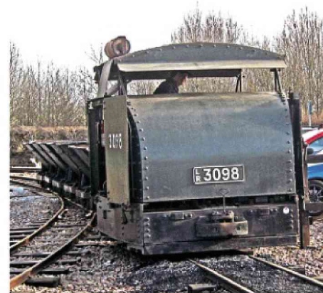
A rare working survivor of the "protected" (lightly armoured) 40hp petrol locomotives built for the War Department Light Railways, after the war, several of this type were used to haul sand trains at Leighton Buzzard, but all were scrapped by the end of the Fifties. LR3098, which was built in Bedford in 1918, worked at Knostrop sewage works, Leeds, and is owned by the National Railway Museum, York, where it returned in the summer of 2016. MERVYN LEAH
