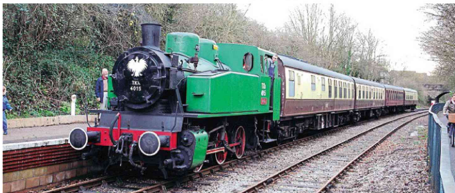
Chrzanow built in 1954 and similar in many ways to the USA S100s TKh 0-6-0T No. 4015 worked at a steelworks at Ostrowiec in the south-east of Poland until withdrawal in 1991, when it was bought by enthusiasts and imported to Britain. It steamed again in 1998 after a £60,000 overhaul. Now named Karel after the Polish Pope John Paul II, it is seen arriving at Oldland Common with a service from Bitton on the Avon Valley Railway on December 27, 2012. Several TKhs have been imported to Britain by enthusiasts for use on heritage lines, because unlike virtually all other Polish standard gauge steam locomotives, they conform to the British loading gauge. HUGH LLEWELLYN
