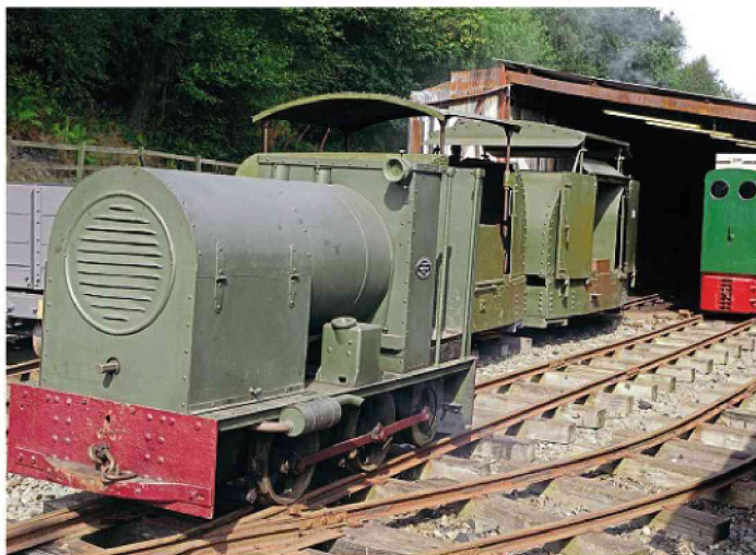
Welsh Highland Heritage Railway-based Baguley 15hp four-wheeler 0-4-0 No. 760 of 1918 was one of a type originally intended to operate close to the Front Line, but, they suffered from glowing exhausts when working hard, which made them ideal targets for enemy snipers. ROBIN JONES
