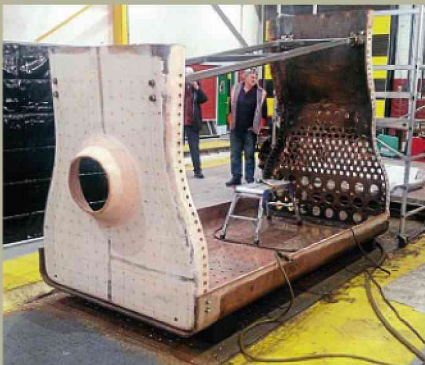
The Patriot firebox taking shape at LNWR Crewe on February 9, 2016. GAVIN SHELL/ LMS-PATRIOT PROJECT
