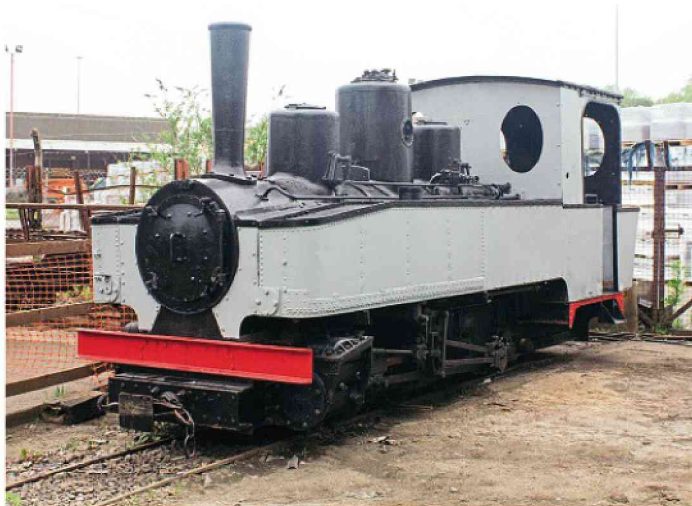
German-built Feldbahn 0-8-0T No. 2023 awaits restoration at Stonehenge Works on the Leighton Buzzard Railway, which acquired it in 2014. Built by Lokomotivfabrik Krauss as No. 7455, after the First World War, it was used on the sugar beet railway at Maizy in northern France. It moved to a sand quarry in Variscourt in 1964 before being preserved in 1970. MERVYN LEAH
