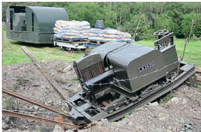
This unfortunate Motor-Rail petrol tractor had toppled over into a bomb crater, now liberally protected with barbed wire, a trademark feature of the trenches. MRT
