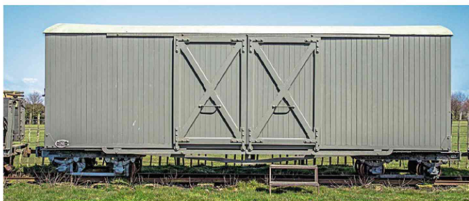
This vehicle is one of 12 First World War 2ft gauge ambulance wagons used on the Western Front trench railways, which were bought secondhand by the Nocton Estates Company in Lincolnshire, for use on its extensive system serving its potato fields, each box van having a six-ton capacity. It was later acquired by the Lincolnshire Coast Light Railway and is part of its museum collection at its current Skegness Water Park base at Ingoldmells. DAVID ENEFER
