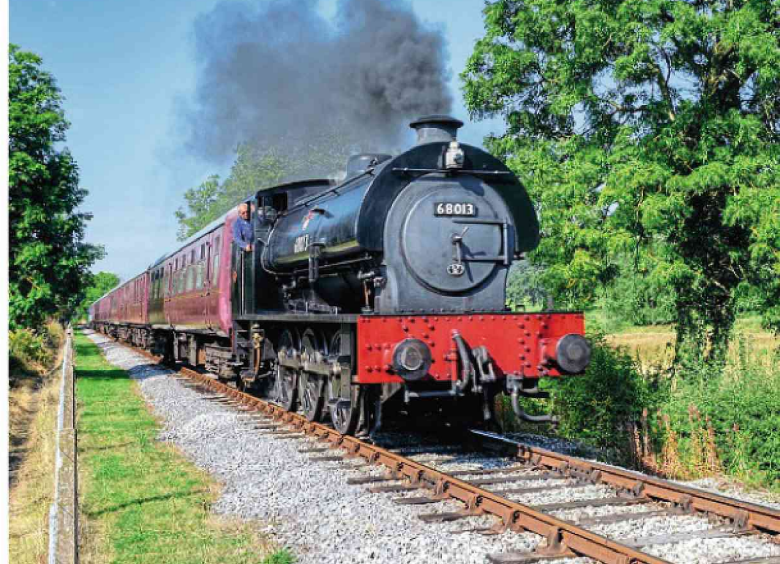
In BR black livery and carrying the mock BR number 68013, Royal Pioneer is seen in Peak Rail service in 2012. Built by Robert Stephenson & Hawthorns as No. 7136 of 1944, it became War Department No. 75186, and was the last of the type to be rebuilt by Hunslet, in 1969, when it became No. 3892. It has run in preservation as Warrington and WD150. Many heritage lines relied on industrial saddle tanks for their initial operations, and several repainted Austerity 0-6-0STs into BR liveries with fictitious numbers as an easy way of getting a 'main line' locomotive 'on the cheap'. ROB BENDALL*
