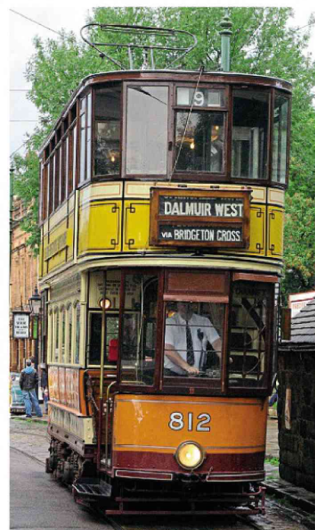
Glasgow Corporation Tramways Car 812 dates from 1900 when it was built as an open-top tram. It was given a top cover with open balconies a decade later and platform vestibules two years after that. ROBIN JONES
