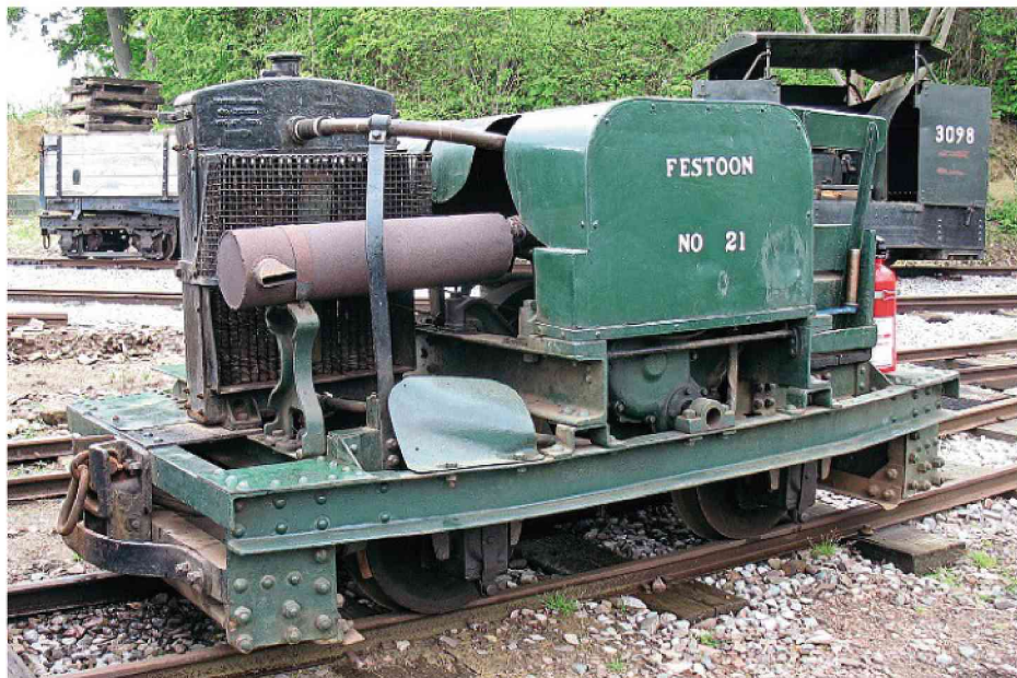
Built in 1929 to a First World War design is Motor Rail 20hp petrol-mechanical four-wheeler No.21 Festoon (works No. 4570), which may well be a rebuild of a wartime machine. Initially used on contracting work, it was sold to the George Garside quarry company in 1931, and hauled sand trains at Leighton Buzzard. It survived the arrival of newer diesels, by being converted to a self-propelled fitters' workbench, and is the oldest locomotive original to the heritage line. To mark the Simplex centenary in 2016, it went on display at the John Higgins Museum in Bedford, from mid-April. GEOFF TRIBE
