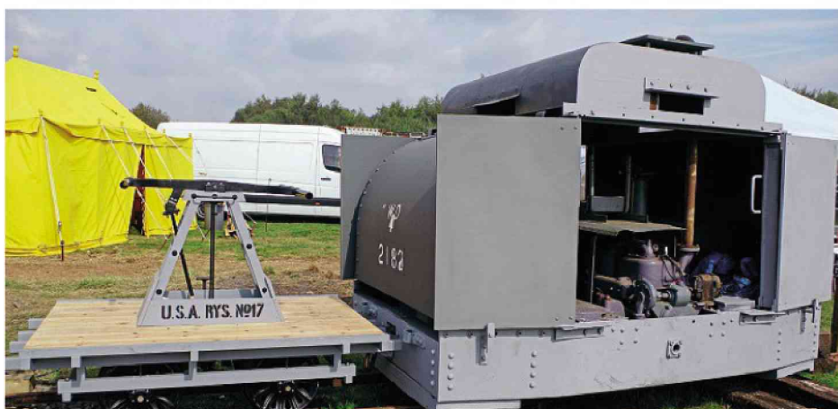
The sole-surviving (out of 34 built) 40hp armoured Motor Rail Simplex, War Department Light Railways 'Tin Turtle' No. 2182 (No. 461 of 1917) still with its original petrol engine. Now in the care of the Greensand Railway Museum Trust based at the Leighton Buzzard Railway. After the First World War, it worked at the Furness Brick & Tile Co Ltd at Askam-in-Furness, near Barrow, and was later preserved at the former Gloddfa Ganol museum in North Wales and then at the now-closed Museum of Army Transport at Beverley in Yorkshire. ROBIN JONES
