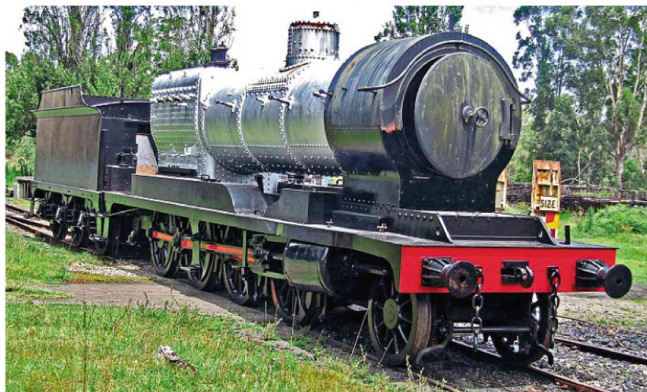
The boiler of Great Central Railway-built ROD No. 23 on its frame at Richmond Vale Railway Museum in NSW, Australia, on January 21. The 2-8-0 has been cosmetically restored. GRAHAM BLACK
