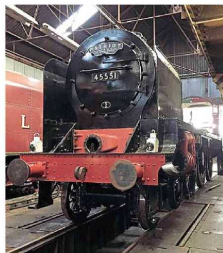
Complete with bogie, The Unknown Warrior became a 4-6-0 at Tyseley Locomotive Works for the first time on February 3, 2016. ANDY COLLINSON/LMS-PATRIOT PROJECT
