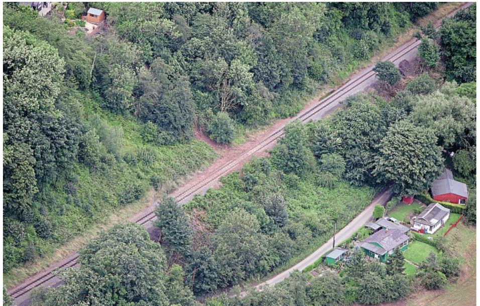
**ABOVE:** A further landslip appeared above New Stanley Cutting between Bewdley and Arley. The slippage started in the garden shed top left in the picture. Before the flood, the shed would not have been visible from this point, but mature trees have slipped down the slope towards the railway. People claimed that they had stood at this point and heard trees moving. SVR
