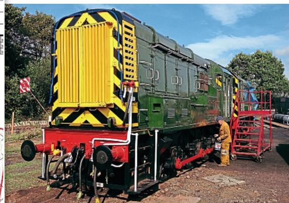
**ABOVE:** The SVR has a fleet of no fewer than seven 350hp 0-6-0 diesel electric shunters, all of which have hitherto had to be maintained in the open air. JONATHAN DUNSTER
