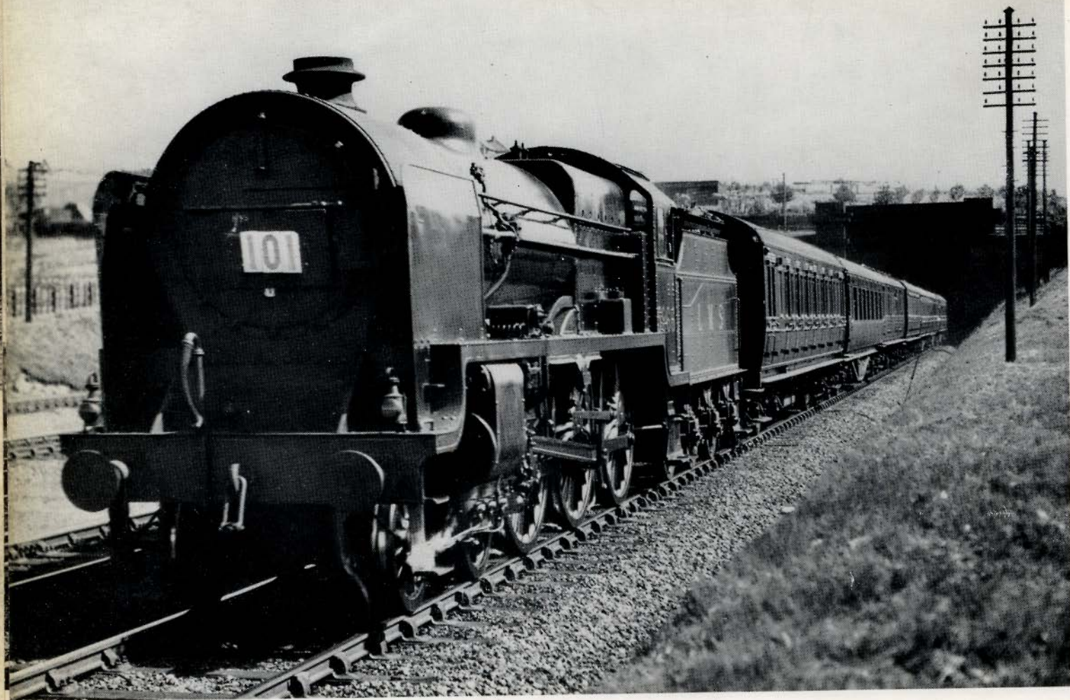
No 5966, hauling the 1.35 p.m. Euston-Aberdeen train, leaves Northchurch tunnel near Berkhamstead in 1933. This engine, later renumbered 5512, is another example of the "Baby Scot" or "Patriot" class 4-6-0's, and is recorded as a rebuild of "Claughton" class 4-6-0 No 1177 (L. & N.W. numbering). However, probably very little was incorporated from the original.
