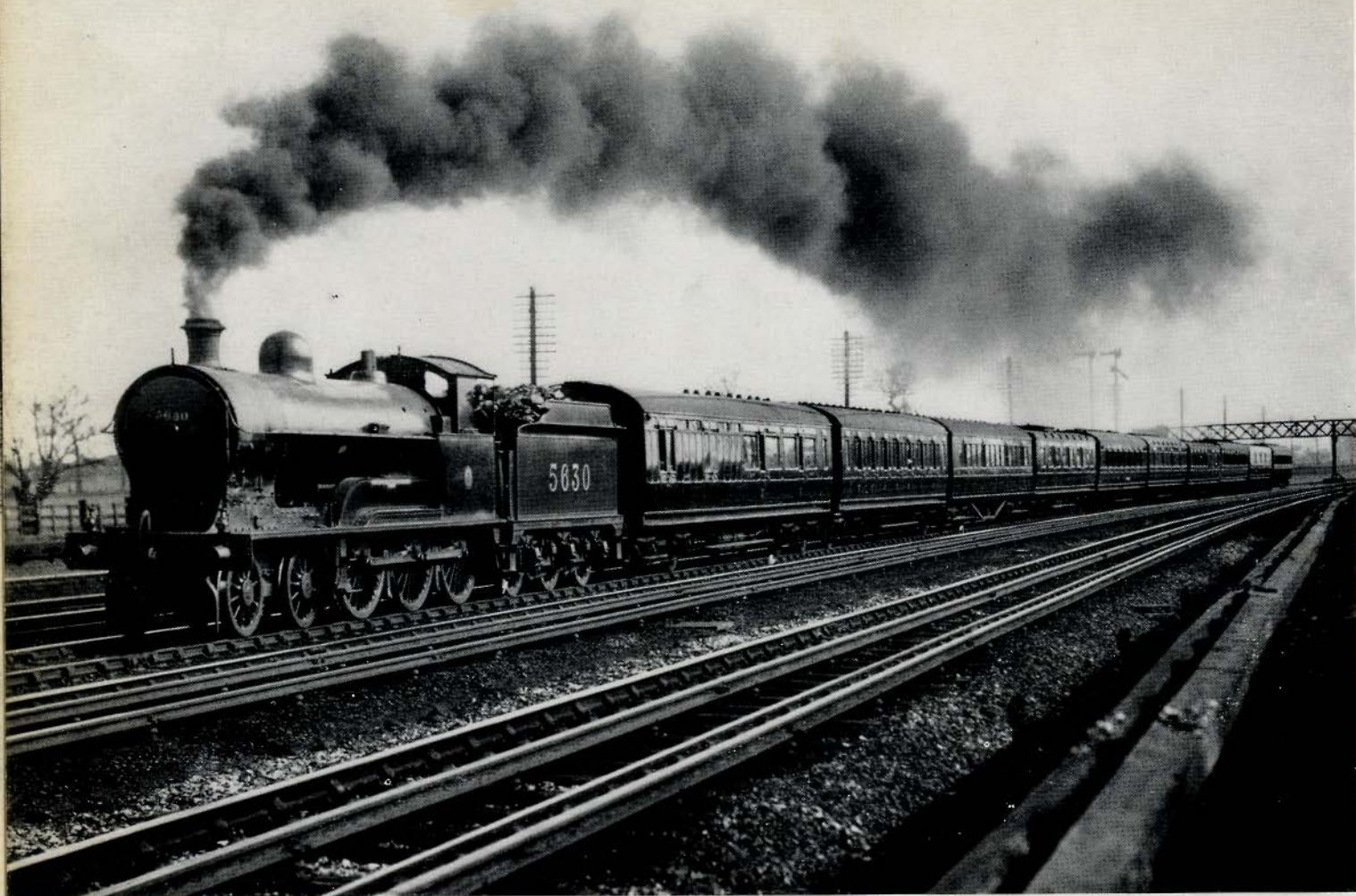
This typical L. & N.W. scene was photographed in 1928, and shows the 2.35 p.m. Euston-Liverpool express in L.M.S. livery. It is hauled by a "Prince of Wales" class 4-6-0 No 5630 (L. & N.W. No 979) WM Thackeray fitted with a tender from a ROD 2-8-0. The location is Kenton, a favourite spot for photographers even before the First World War.
