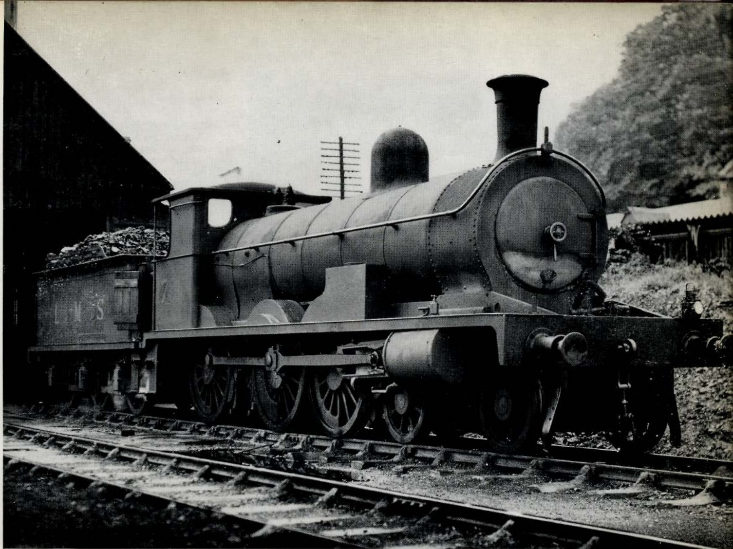
Waiting at Dingwell on a wet and misty day in 1939 is a member of a famous class of Highland Railway locomotives—a "Jones Goods" 4-6-0. The engine No 17917 (H.R. No 104), was shedded at Inverness.
