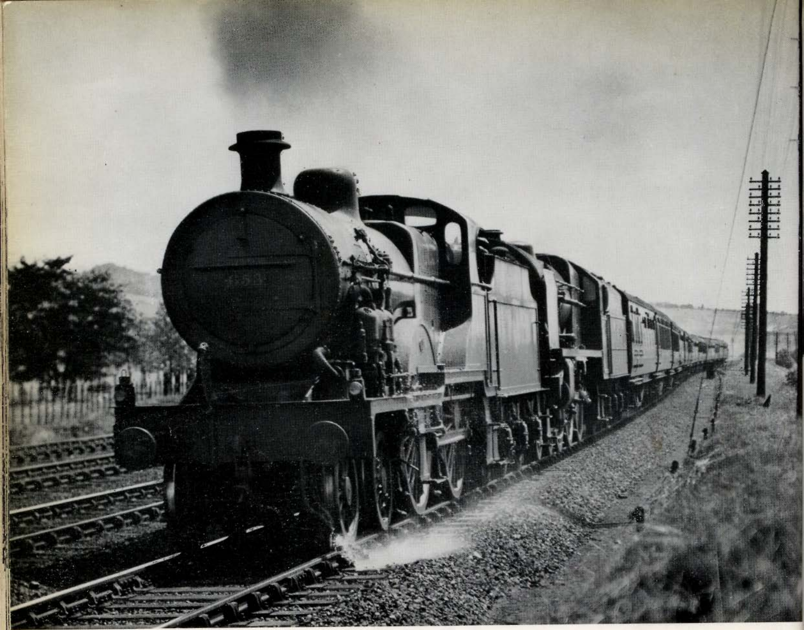
Here, the "Mancunian" is seen near Berkhamstead in 1937. The pilot engine is a Class 2 4-4-0 No 653 fitted with a Dabeg feed-water heater (which is dribbling), in front of No 6165 The Ranger —12th London Regt., a 4-6-0 "Royal Scot". At one period the "Mancunian" was a "limited load" train, which may explain the use of a pilot engine, although this particular train does not appear to be much in excess.
