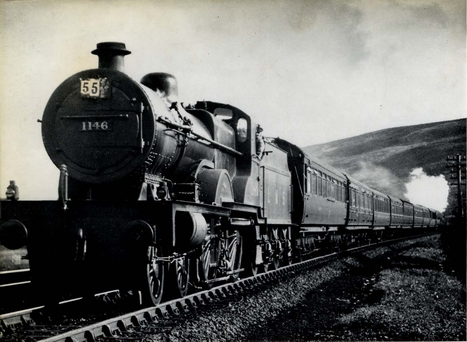
A standard 4-4-0 Compound No 1146 of Carlisle (Upperby) takes an excursion train up Beattock bank, assisted by Caledonian 0-4-4T No 15154 at the rear, in July 1936. The origin of the first coach poses a problem—it is possibly L. & Y.
