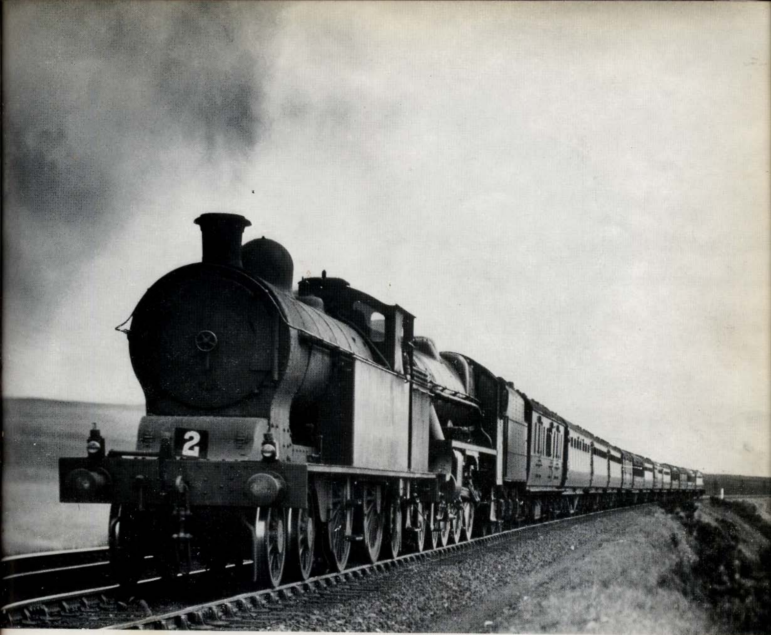
The 10.05 a.m. Euston to Aberdeen express climbing Shap in 1937. The train engine is "Jubilee" class 4-6-0 No 5671 Prince Rupert , and the pilot is an ex-L. & N.W. "Precursor" 4-4-2T No 552 (L.M.S. No 6794). Note the target number for banking duties on the buffer beam.
