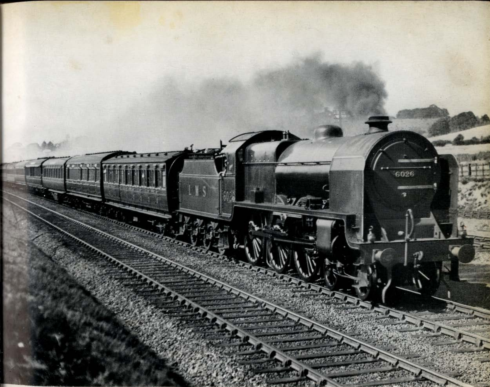
The Thirties version of the pre-1914 "Sunny South Special" passes Berkhamstead on its way to the coast in 1933. The engine, one of the "Baby Scot" or "Patriot" class, 4-6-0 No 6026 (later re-numbered 5523), and is recorded as a rebuild of L. & N.W. "Claughton" No 211. Note the splendid mixture of coaching stock: the first vehicle may possibly be an ex-Lancashire and Yorkshire, and further down the train are a couple of coaches from the Southern Railway.
