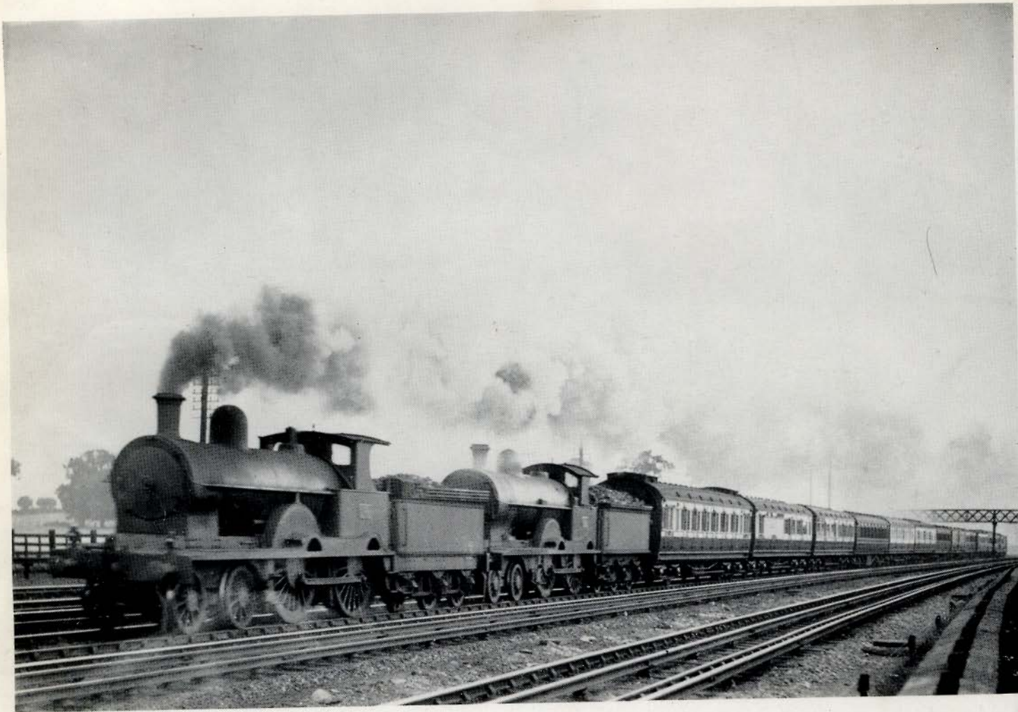
Except for two coaches in L.M.S. colours, this shows a fully representative L. & N.W. scene of past days, photographed at Kenton in 1924. 4-4-0 No 1905 Black Diamond , rebuilt from a four-cylinder Webb Compound, heads the 2.35 p.m. Euston-Liverpool express. The train engine is "Precursor" class 4-4-0 No 282 Alaric , apparently superheated and with pop safety valves, almost identical to the "George V" class. Note that the first coach resembles a double-ended slip.
