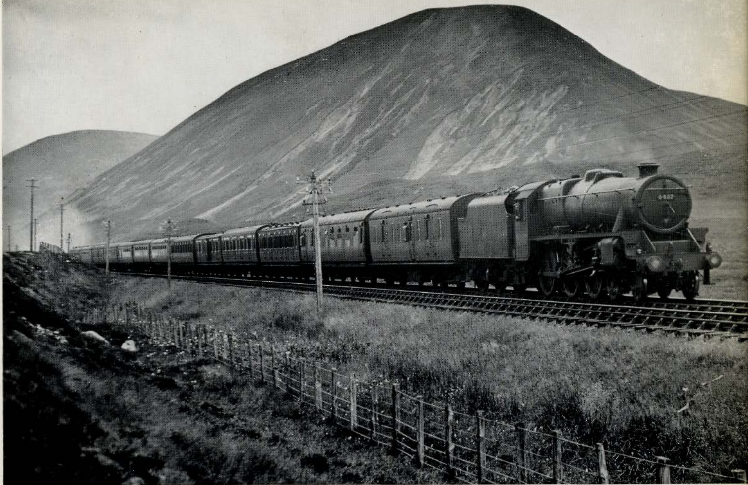
The Grampian mountains near Dalnaspidal dominate this photograph of a "Class Five" 4-6-0 No 5457 heading a fast train of well-mixed stock from Glasgow to Inverness in August 1939. The double line of telegraph poles is due to the main road running alongside the railway.
