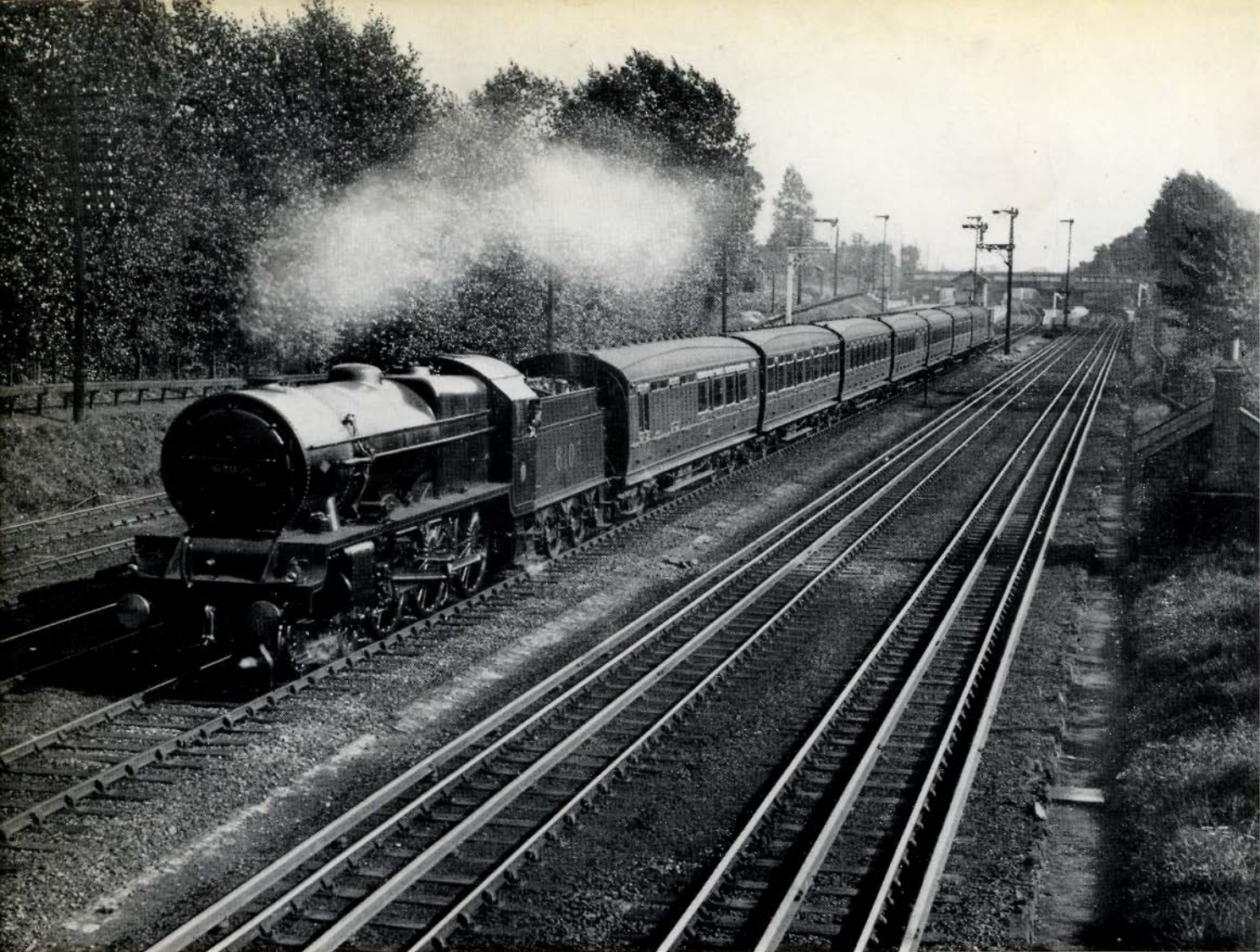
This brand new "Royal Scot" 4-6-0 was only a fortnight old when this picture was taken in September in 1927. It was a lucky shot, as the train was only seen when it was passing through the station, and the camera had to be hastily brought out of its box to record No 6105, subsequently named Cameron Highlander , on a Rugby fast from Euston passing Hatch End and Pinner.
