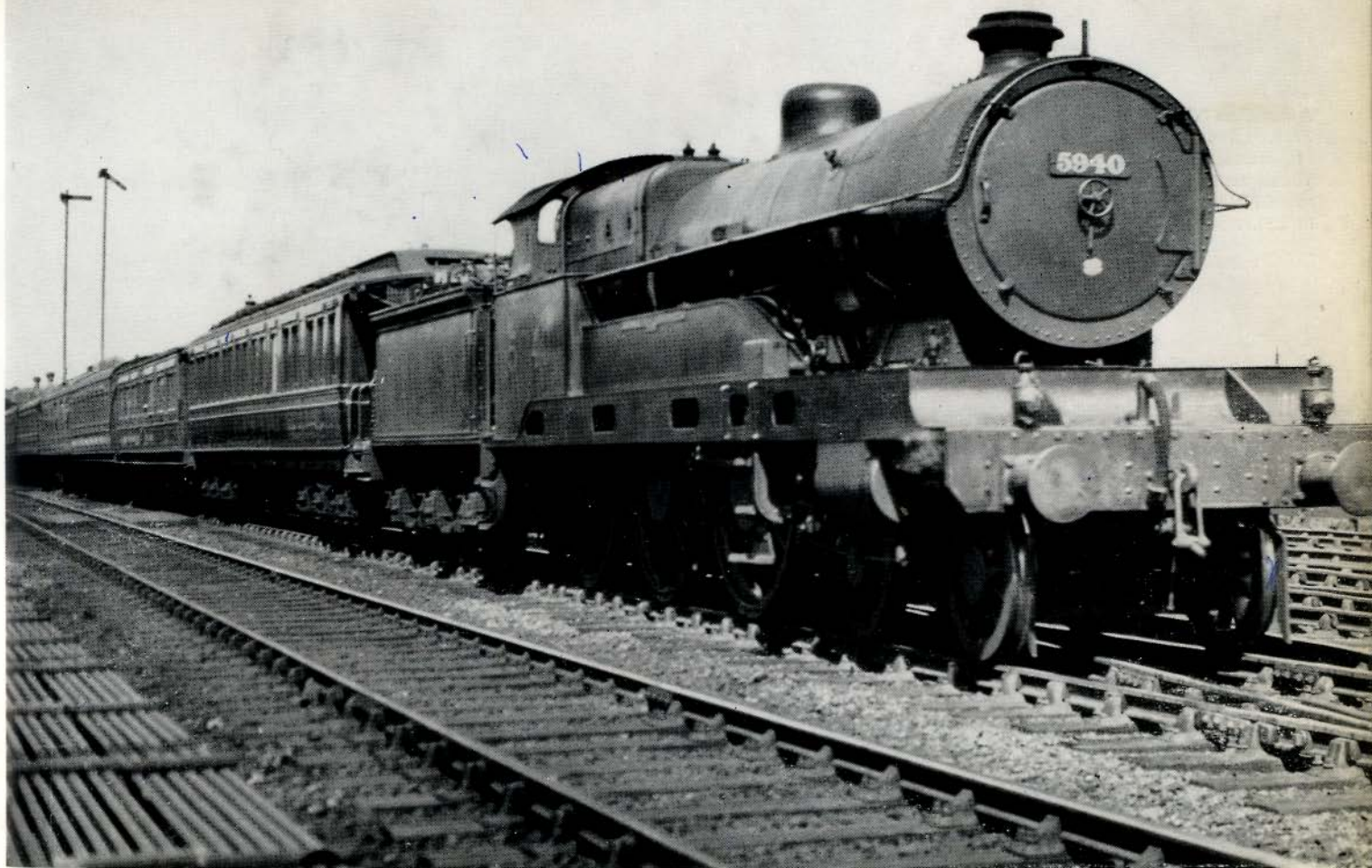
Another "Claughton" class 4-6-0, this time rebuilt with a larger boiler. No 5940 (L. & N.W. No. 1019) Columbus leaves Bletchley with the 9.05 a.m. Llandudno Junction to Euston train in 1933. Note the very tall signals at the rear of the train.
