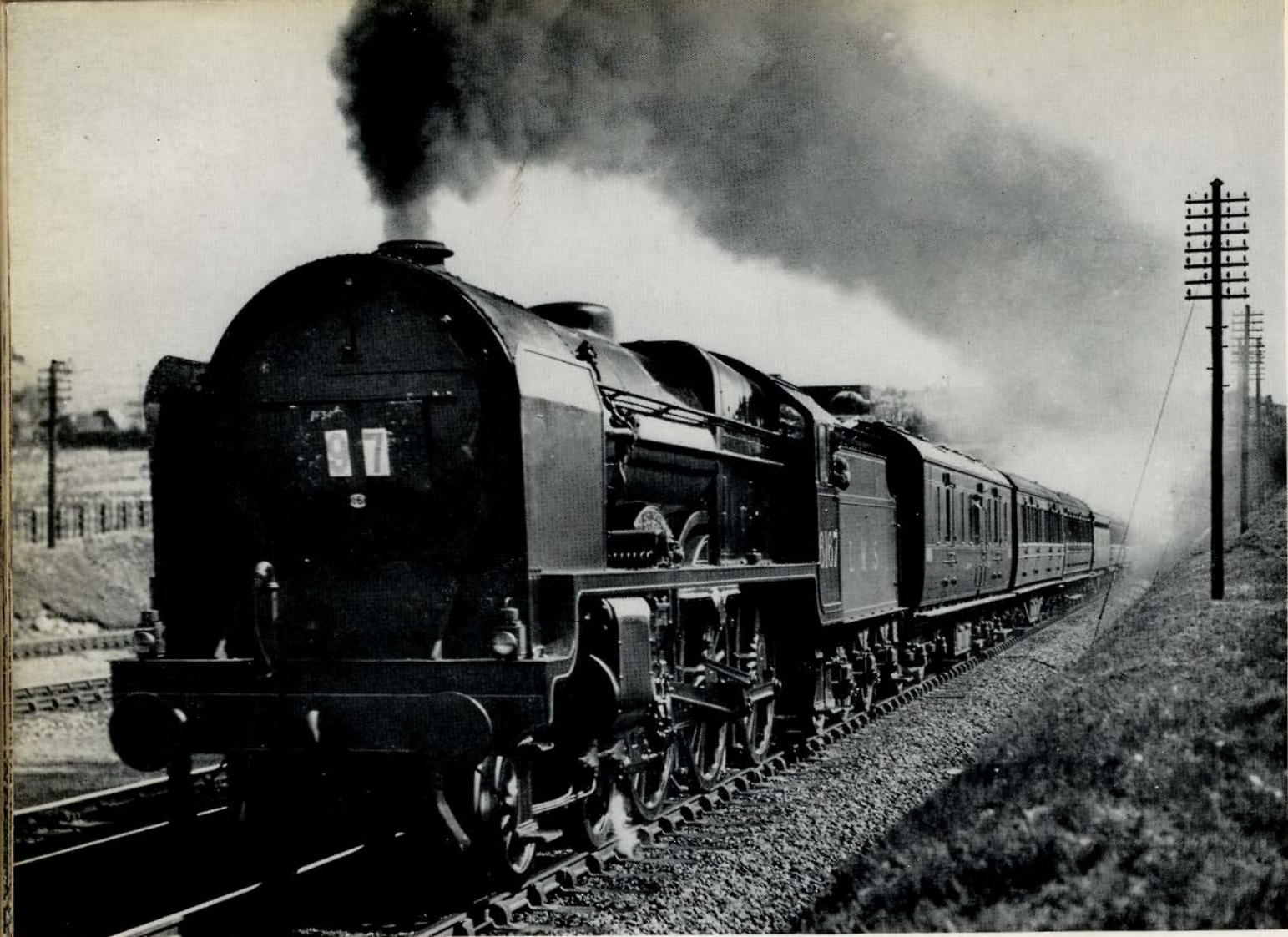
Storming out of Northchurch tunnel comes a "Royal Scot" 4-6-0 No 6167 Hertfordshire Regiment with the 1.30 Euston-Edinburgh-Glasgow train. The picture, taken in 1933, shows the engine with smoke shields and extra coal rails in the tender.
