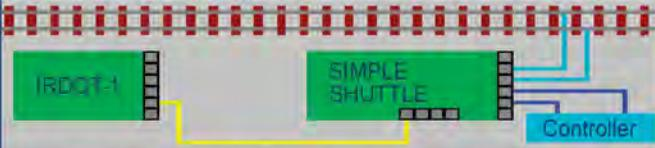
Wiring is simple. Apart from connections to a 12 to 16 volt (AC or DC) power supply the diagram shows all the wiring. The Simple Shuttle can also be used where there are sidings at one end of the line. A train arrives in one siding, the points automatically change and a different train departs after the delay. This uses a simple shuttle and an IRDOT-P at the end of every siding. Track power is obtained from a conventional controller.
