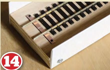
**14** To hold the rails securely in place at each end of the cassette a strip of copper-clad board is pinned to the cassette base. This is cut to length, the copper cut through on both sides in the centre (but not the central insulated core) and then pre-drilled with 1.5mm diameter holes to accept a pair of track pins. The process is repeated at the other end on the main cassettes, but not for the locomotive cassettes as these require a different method...
