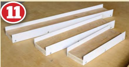
**11** Once assembled the bare cassettes will look like this. The depth of the plastic used here is just enough to catch a train should it be knocked in movement around the storage yard but not so high that it prevents access for assembling trains at the start of exhibitions and running sessions. All three cassettes shown here are locomotive cassettes of different lengths.
