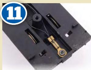
**11** With the tender weight removed two 2mm diameter holes were drilled at the front of the tender chassis to allow the wires to be routed through. Choose your location carefully to avoid conflicts with other wires. Once the holes were drilled the tender weight was reinstated.
