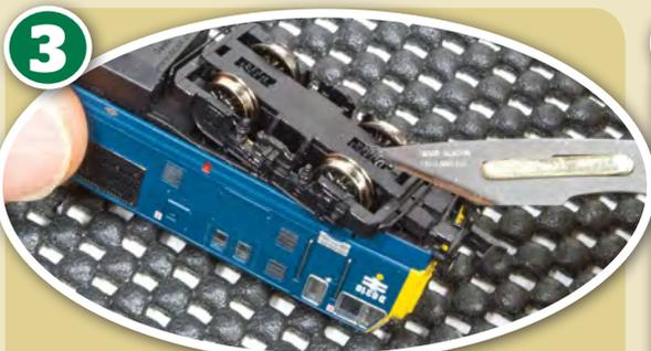
Apply lubricants sparingly using a pin or the tip of an old scalpel blade. This model has been placed on a workbench mat suitable for resting models on during maintenance work.
