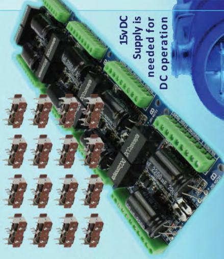
15vDC Supply is needed for DC operation
