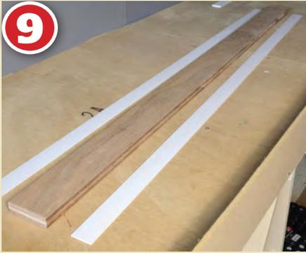
**9** With all the components cut to size the cassette is ready to assemble. The next step is to run a bead of PVA glue along the edge of the cassette base to help secure the plastic strip to it.
