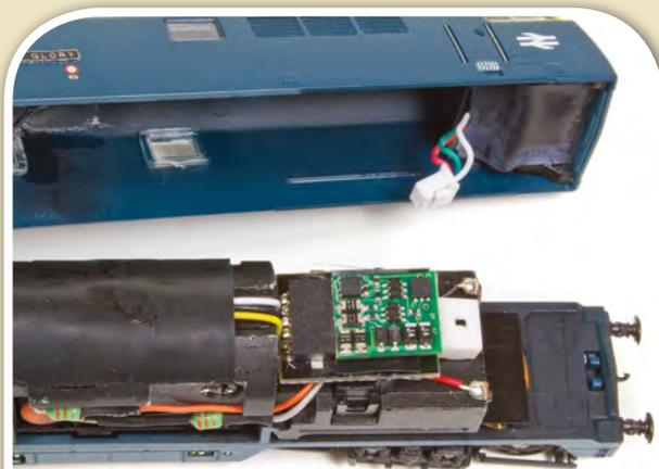
10 A 6-pin NEM-651 decoder plugs straight in its place. This is a Digitrax DZ1261N decoder.
