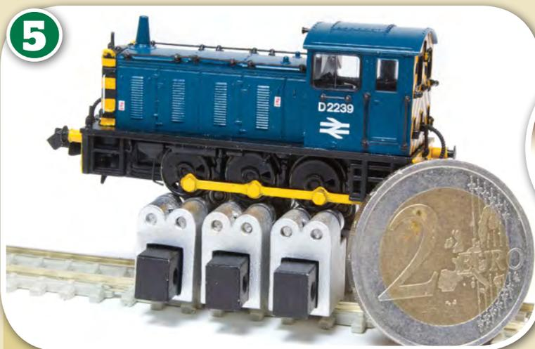
It's tight, but the Graham Farish Class 04 just manages to sit on the saddles for an hour of running in time. The real challenge with small locomotives is good current collection from something which weighs so little. A decoder has to be squeezed in that small locomotive body too.
