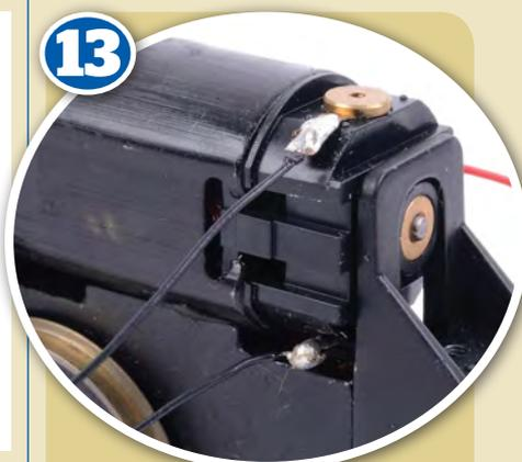
**13** New connections were then made to the motor using fine multi-core decoder wire. We used black wire throughout the installation and while this makes it more difficult to install, the end result is much neater.
