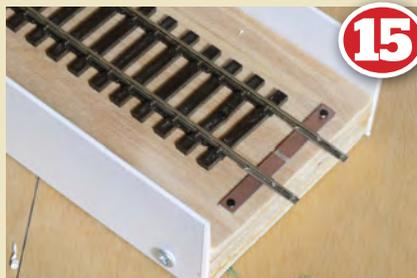
**15** To allow the locomotive cassettes to be connected to the main cassettes a pair of rail joiners is added at one end only as well as the copper-clad strip as in Step 14. This means that on arrival a locomotive can be detached from its train on a cassette, turned and reconnected to the 'landing pad' at the other end of the yard and, in turn, to another train.
