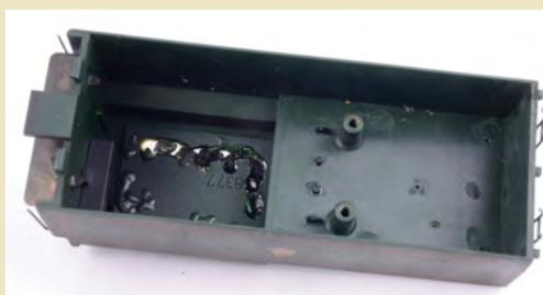
**7** However, on inspecting the tender body it appeared that I had been here before with a drill and the space below the coal is the perfect place for a speaker to be installed. What's more - a decoder can be accommodated behind the supporting lugs too.
