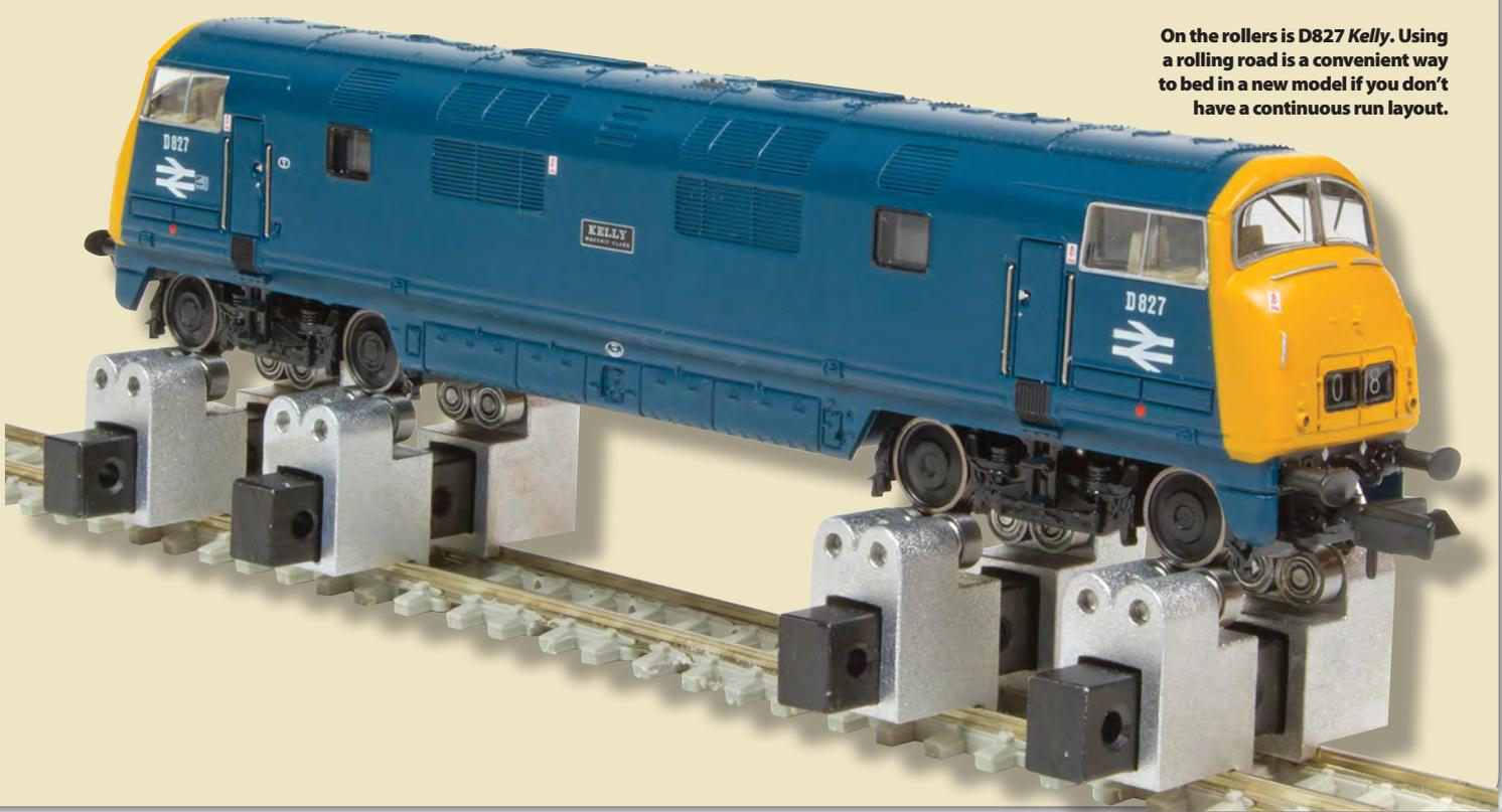
On the rollers is D827 Kelly. Using a rolling road is a convenient way to bed in a new model if you don't have a continuous run layout.
