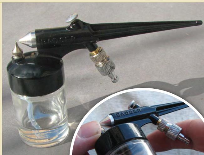
**3** This kind of airbrush is very simple in design, but a limited amount of control is still possible. Turning the paint tip clockwise as far as it will go and spraying at low pressure gives the kind of fine mist we want in weathering, although precise targeting isn't really possible. Turning it up so it's right in the air stream yields a wider, more full-blooded spray pattern that would be good for painting coach roofs, scenic work and ground cover.
