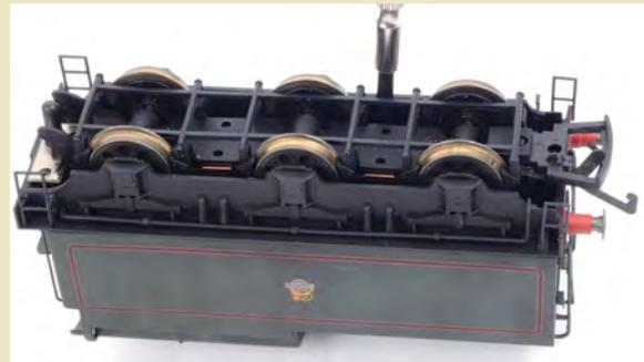
**5** Faced with a lack of space in the locomotive and no socket the best place to turn is the tender. The 'Merchant Navy' tender body is secured by two crosshead screws located behind and above the middle wheels.
