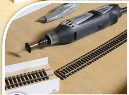
**13** At the other end of the cassette the sleeper web is cut before the track is pinned. Once laid the track can then be cut precisely to length using a mini drill with a cutting disc. Once cut slide the previous cut sleepers out from under the rails completing the track laying phase.
