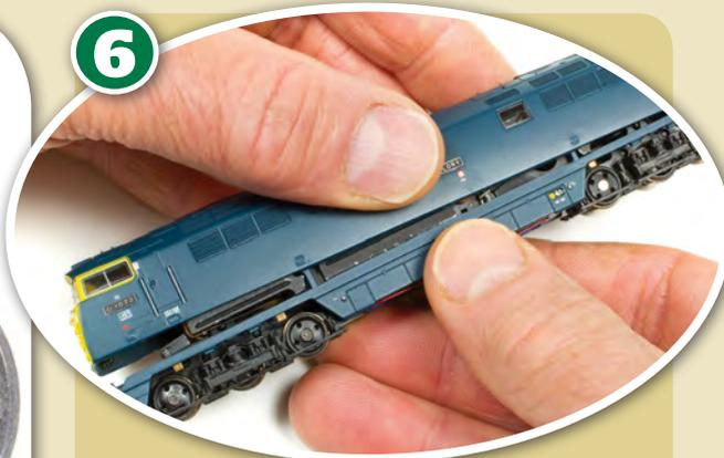
Most 'N' gauge locomotive bodies can be separated from the chassis by simply releasing small body clips with a fingernail and pulling them apart gently.
