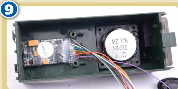
**9** The LokSound V4.0 decoder didn't quite fit between the lugs and the tender rear initially. Pairing away at the support lugs carefully opened out the space by the extra 1.5mm required to fit the decoder in. Here the decoder, still attached to its supplied 23mm speaker, and new QSI speaker are loosely positioned for testing.
