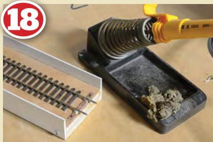
**18** At the opposite end of the locomotive cassettes rail joiners and rails are soldered to the copper-clad strip to make a firm joint. It is now just a case of building more – lots more – as in total we have 30 locomotive cassettes, 17 seven carriage cassettes, six four carriage cassettes and three eight carriage cassettes.
