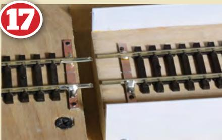
**17** Having soldered the rails to the cladding strip, pull the cassette back and the rails will stay firmly fixed in place. This fixing point makes it a simple procedure to rejoin the cassette to the 'landing pad' in operation.
