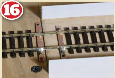
**16** Securing the rails to the cassettes means soldering them to the copper-clad strip. To do this successfully we connected each set of rails to the rail joiners on the 'landing pad' during soldering to ensure they remained in gauge and at the correct height. Make sure you don't solder the rails to the rail joiners here though.
