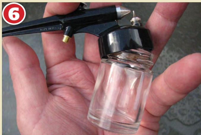
**6** Clean the airbrush thoroughly as soon as you've finished weathering. Wipe the paint jar clean, fill it with thinners and spray this out through the nozzle until the fluid runs clean. Use a second jarful of thinners if necessary, then gently run a length of 0.7mm soft brass wire through the paint tip to clear any remaining particles of paint. To get the most from it, your airbrush should be as clean as a new pin at all times. The second you start to neglect it, it will start playing up.
