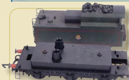
**6** With the tender body removed we are confronted with a large weight. On first glance this looks to be a problem, particularly for inclusion of a speaker, as it occupies a large amount of space.
