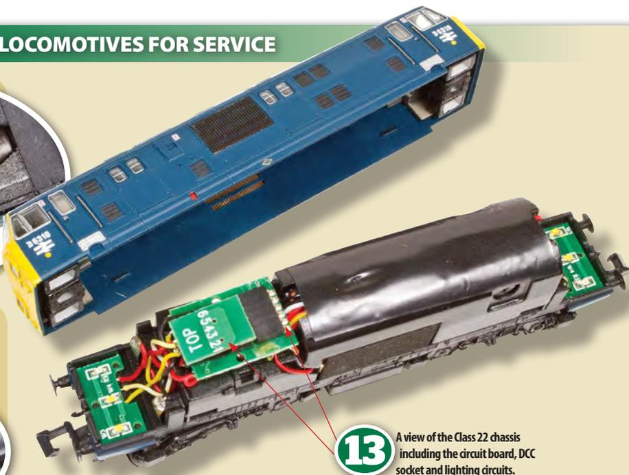
**13** A view of the Class 22 chassis including the circuit board, DCC socket and lighting circuits.
