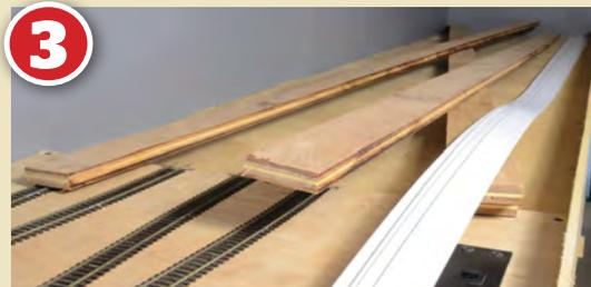
The raw materials for our cassette design consist of strips of 18mm thick plywood and 35mm x 2mm plastic strip for the sides. The wooden strips were cut by a local DIY store into 60mm widths, 8ft long and the plastic strip was sourced from an internet wholesaler site.
