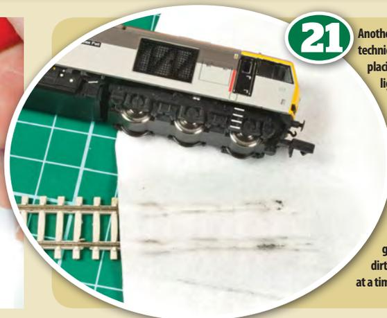
**21** Another wheel cleaning technique involves placing a paper towel lightly soaked in IPA on a piece of track. The model is held with one bogie on the towel and one on the track to collect current so the wheels rotate to gently remove the dirt from one bogie at a time.
