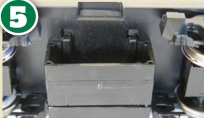
With one tank side removed the fixing method can be seen clearly. Note the rubber tab at the top of the picture which helps to retain the motor.
