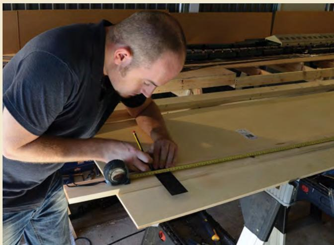
**1** Building solid top baseboards is a simple process, which can be made even easier with the right materials. Using a pre-cut piece of 9mm plywood 1,827mm x 606mm – roughly equal to 6ft x 2ft – we reduce wood cutting to a minimum for this baseboard. Four lengths of 69mm x 18mm timber are also needed to make the baseboard frame. Start by measuring two pieces for the sides of the frame. Mark a line across the width of the timber 1,827mm from the end using a tri-square for accuracy.
