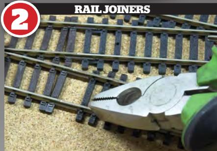
Picking the right rail joiners for your track is essential – different sizes are available for different scales and also for the different rail profiles. When fitting rail joiners always ensure that both rails are fully aligned in the joiner – use pliers to ease them into position and leave a small gap, no more than 1mm, to allow for expansion of the rails.
