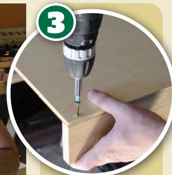
**3** With the ends of the side timbers cleaned up with sandpaper they can be fitted to the top. Using 3.5 x 35mm long screws the two sides of the frame were attached to the plywood top using an electric screwdriver for ease.
