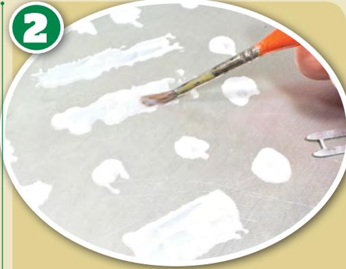
The first stage is to clip a slip of plastic sheet to the metal plate and apply randomly shaped spots of adhesive to it.
