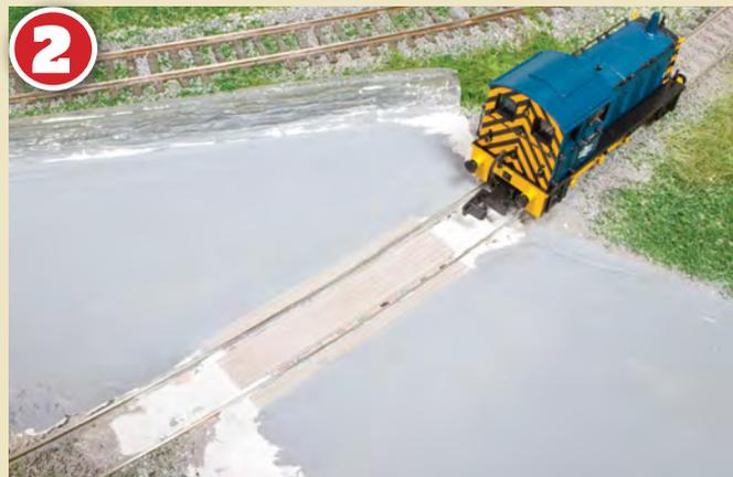
**2** The improved crossing was tested with various locomotives to ensure that they remained in contact with the rails over the full length of the wooden board insert.
