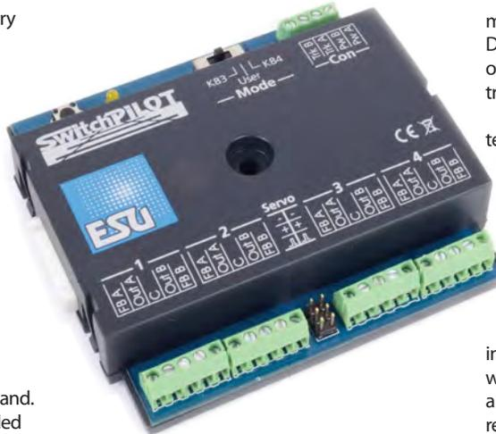
output can be modified to suit different pulse rates. Three modes are provided to suit solenoid, user defined and colour light signal operation.
