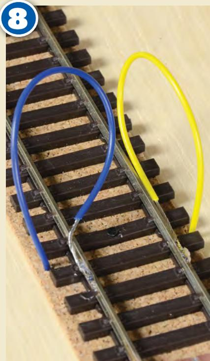
The wires can now be threaded through the 2mm diameter holes made earlier.
