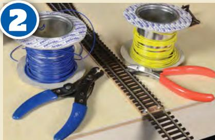
Having drilled holes for the first wires the next step is to prepare the wires for soldering to the rail sides. You will need two wire colours – we used blue for the near rail and yellow for the far rail – plus a pair of wire strippers and a set of side cutters.
