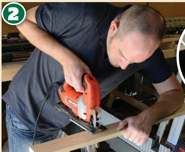
Having marked the two side pieces the redundant ends can be cut off using either a jigsaw or a handsaw. Take care when using these tools to ensure a straight cut across the timber.
