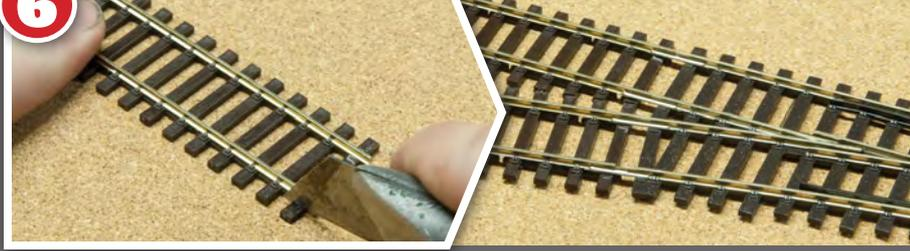
To join two lengths of flexible track to a point requires a small modification to allow the sleepers to fit together. All you have to do is cut the first three sleepers down at an angle – the first against the rail chair, the second a third of the way from the chair to the outer edge and the third two thirds of the way from the chair to the outer edge. With these three small cuts done two lengths of flexible track can comfortably be connected to large and medium radius points.
