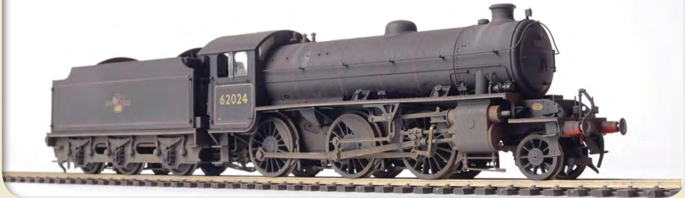
**12** The process of adding tints of colour based around black and orange is continued all around the locomotive. All the time I am referring to good, sharp colour photographs to see what happens where – tinges of rust on the cab steps, brake block dust on the tender frames, random marks and abrasions. I've rather overdone things on the cabsides but, having used enamels on top of fast drying acrylics, I can easily remove the surplus with white spirit. I don't use a barrier between coats.
