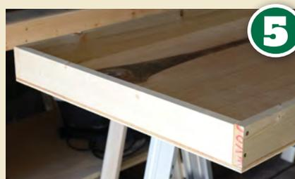
Having measured and cut the end pieces, they can be pushed into place and fixed to the outer frame timbers with screws. It will make this job easier if you drill a pilot hole through the side timber ends to accept the screws and save splitting the wood.
