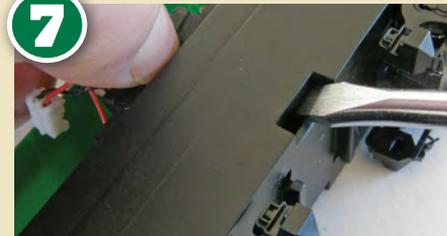
Free the lower rubber tabs from their locations in the chassis slots with a non-damaging edge. Use this to lever from below, whilst pulling from above to remove the motor.
