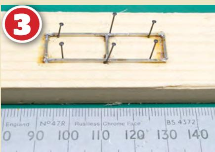
**3** In the meantime, crossing gates composed of 1mm square nickel silver rod were soldered together on a simple jig formed using a block of wood and trackpins to ensure that both gates were assembled to the same standard.
