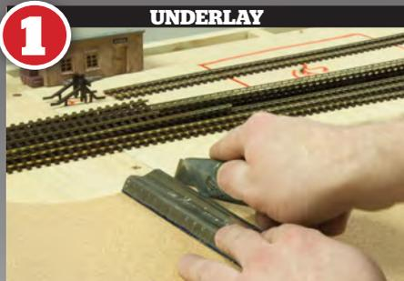
An underlay such as cork or specially designed foam products makes a big difference to the operation and appearance of a model railway. As well as providing sound deadening, underlay will also allow creation of a realistic ballast 'shoulder' should you go down the loose ballasting route. Our choice is always 1/16in cork sheet cut down to the width of the sleepers after track laying.
