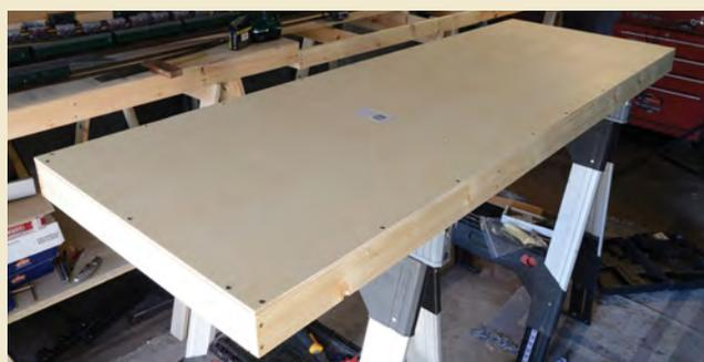
To complete the baseboard, screws were added through the baseboard surface into the end and cross braces to provide a rigid and sturdy base for the layout. This model will be supported by a pair of our standard trestles, but could equally be supported by drawers or simpler straight legs.
