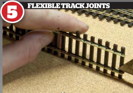
Joining lengths of flexible track takes a little more work than set track items. Rail joiners are supplied separately and in order to fit them the chairs need to be cut off the first sleeper to make a small gap for the joiner to sit in below the rail. To do this turn the track on its side and, using a craft knife with a sharp blade, carefully slice the chairs off. Rail joiners can then be slid onto the track end.
