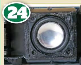
A final alternative would be to use a 23mm Hi-Bass speaker instead. More material will need to be removed from the tank for this to fit, plus it is slightly
