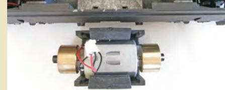
Here are the components seen from above. The open cavity which houses the motor is now exposed allowing holes for the speaker wires to be made in the chassis base.
