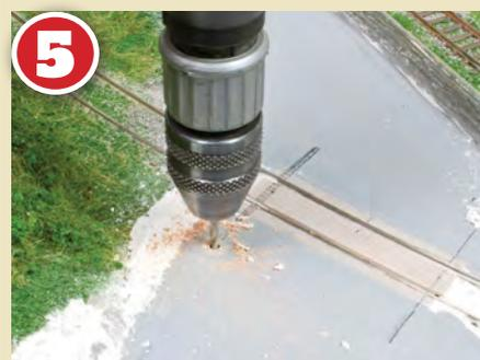
**5** Vertical pivot holes are drilled through the baseboard as carefully as possible to avoid damaging the surrounding road surface and scenery.
