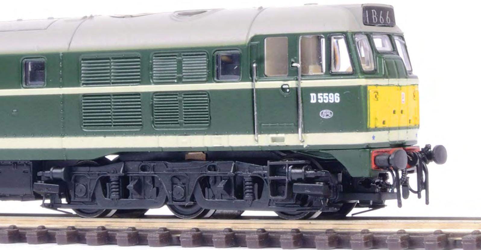
a four character route indicator box – Bachmann's '31' representing the production locomotives – which features illuminated 1B66 and 2B78 headcodes.
