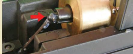
When removing the motor note the position and orientation of the cardan shafts and flywheels to aid re-fitting.
