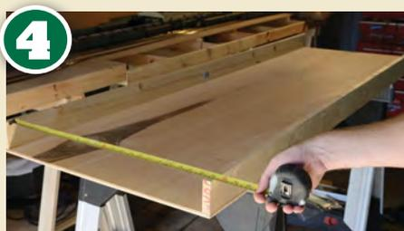
To make the end timbers for the frame, measure the space between the two outer timbers carefully at each end. We have found that the distance usually varies by a couple of millimetres from the original cutting of the plywood top.
