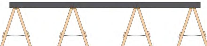
Trestles can be used in a similar manner to folding legs. One trestle will need to be positioned under each baseboard joint and at the outer ends.
