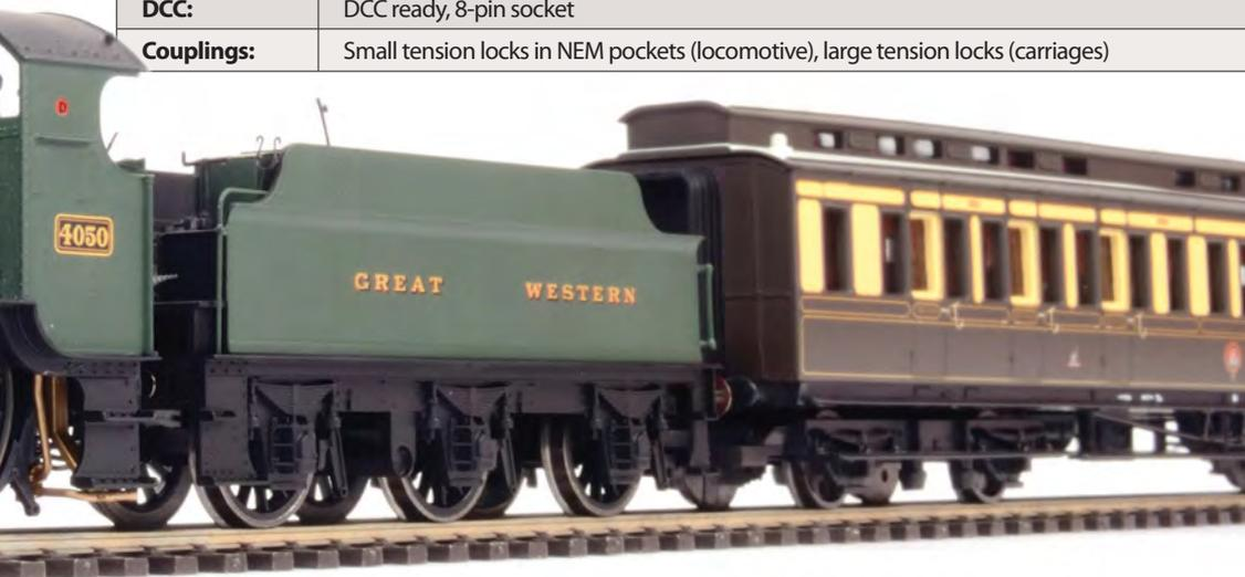
motor encased inside the detailed body. An 8-pin DCC decoder socket is provided in the tender too. Our sample did though feature a number of fingermarks from assembly which should have
