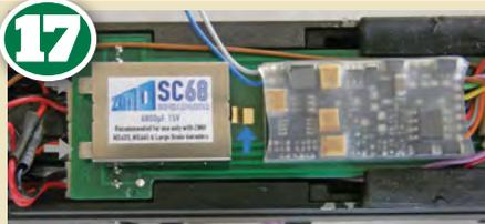
The SC68 fits neatly above the PCB without extending beyond its edge – useful if you have fitted a 'sugar cube' speaker behind the cab at this end. There are some exposed PCB connections under the SC68 which I insulated before final fitting. Solder the blue and grey wires shown to the tabs following the colour coded arrows.
