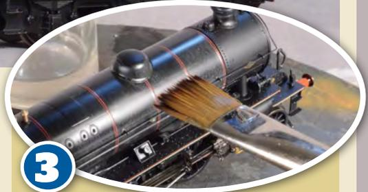
**3** Once the wash has gone on I let it harden for a few minutes and then take it off again, using a half-inch flat brush – I like the Daler-Rowney Aquafine range for their quality and durability – dipped in clean white spirit. Work with downward strokes to suggest rainwater, priming and so on running down the boiler. You will never get all the paint off, which is precisely the point. It accumulates in out of the way places and yields a most pleasing effect.
