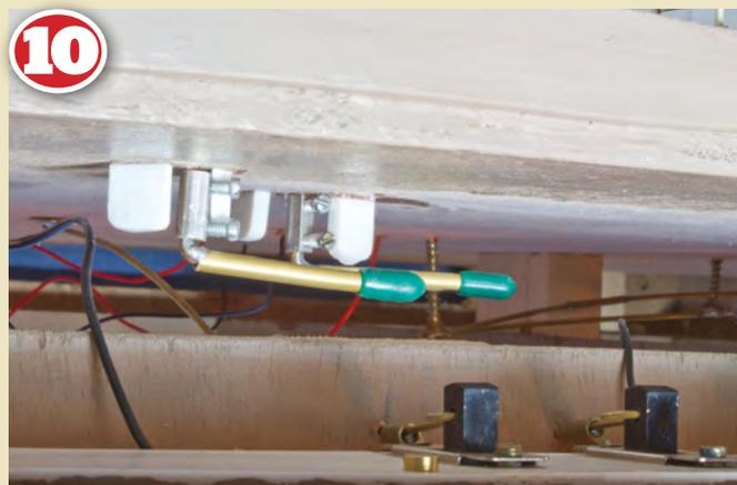
**10** A view of the underside of the layout shows the completed assembly with levers and styrene stop blocks. The levers can be reached with fingers and operated with ease to open and close the gates.
