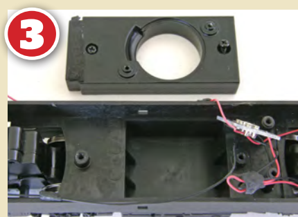
With the weight removed the fuel tank space below was revealed - an ideal location for a fully sealed speaker enclosure.
