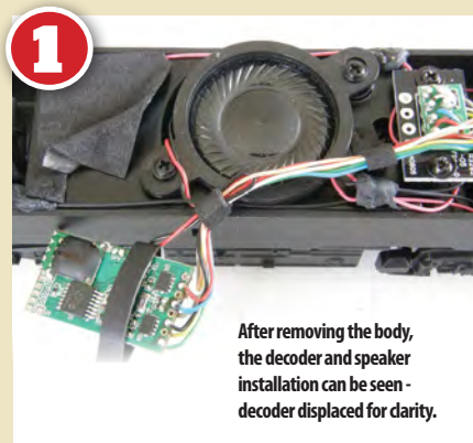
The decoder was unplugged, the speaker retaining ring removed and the insulating pad on which the decoder normally fits peeled off. Arrows indicate the weight retaining screws - these and the DCC socket screws must be released to enable the ballast weight to be removed.
