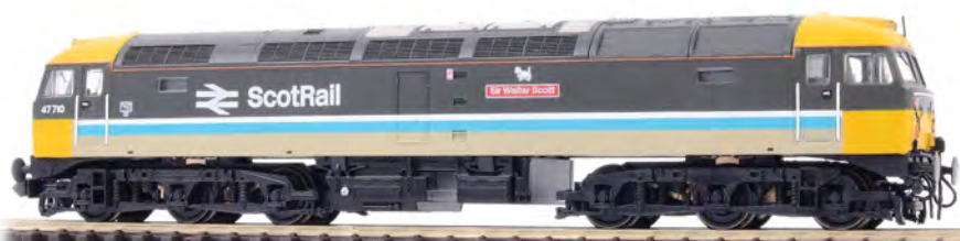
Side-on, the big diesel is impressive. The fuel tanks are a new moulding to suit the Class 47/7 while a full complement of bufferbeam detail is included for optional fitting.
