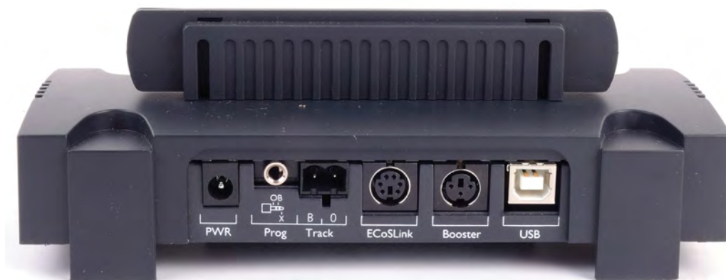
Connectivity on the base station has been enhanced with provision of a USB port and separate outputs for programming and main tracks.
