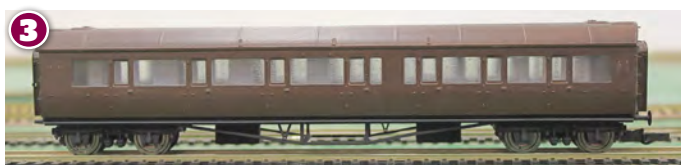
1. The compartment side of the diagram D95 Collett 'bow-ended' Corridor Composite. This is a rapid prototype of the model.
