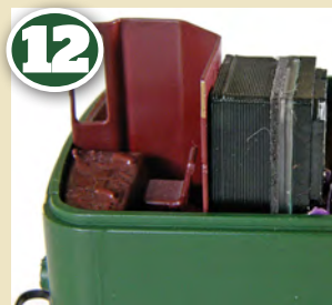
12 The only realistic speaker choice for the '00' gauge AC Cars railbus is a sugar cube. I tried out several different positions for the Zimo cube speaker. Here it is next to the driver's cab, close to a part opened window.
