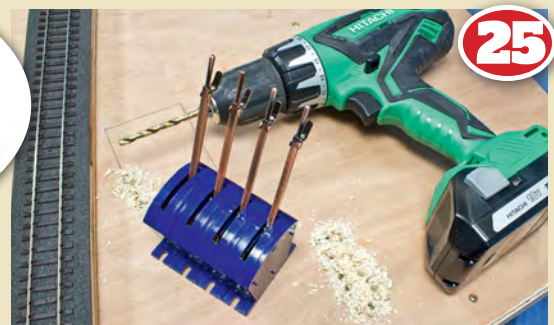
Openings large enough to accommodate four Cobalt S levers and wiring for the DCC system were cut into the top of the transfer yard baseboard. This was done by drilling a series of 6mm diameter holes around the edge of the opening then joining the holes together. The final stage was to clean the edge with files and sandpaper.
