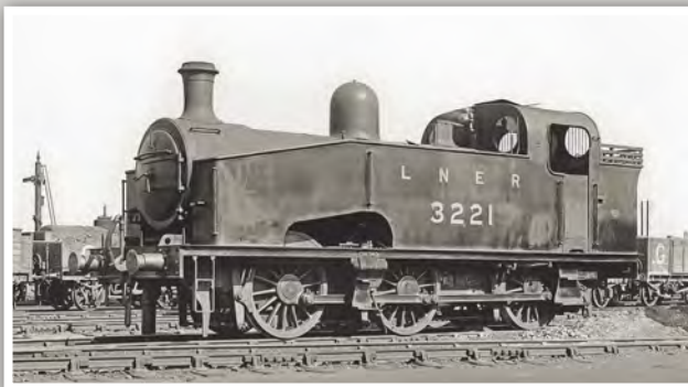
Above: The 'J50s' were powerful and purposeful tank engines designed for shunting work and short distance goods. 3221 stands at New England shed in 1926. Frank Hebron/Rail Archive Stephenson.
