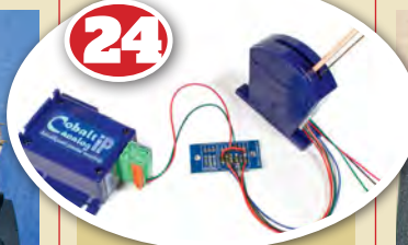
The plan included the use of DCC Concepts Cobalt S levers to switch the current to the point motors. Each lever has a momentary contact switch for solenoid motors together with two independent single-pole double-throw switches.
