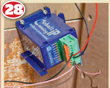
A completed Cobalt IP installation with power from the levers being fed through the pink and brown wires. The red and black wires connect to the turnout's common crossing for polarity switching.
