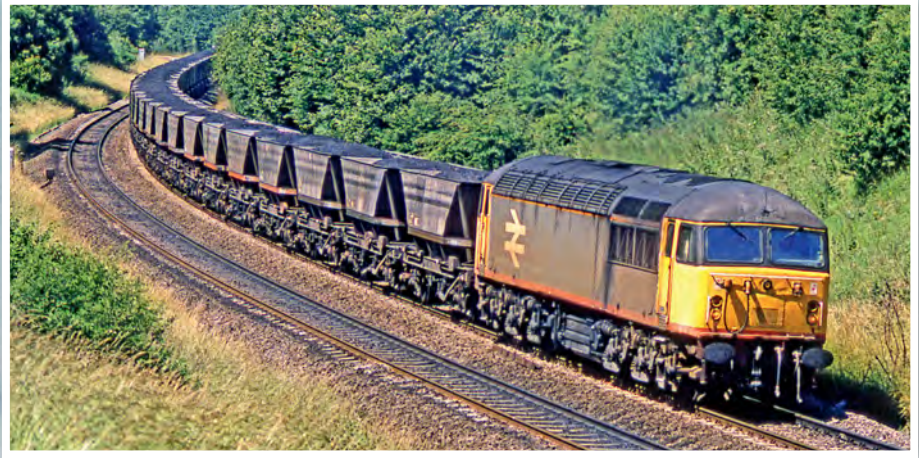
Air-brakes allowed longer and heavier trains to be handled by single locomotives such as the merry-go-round coal trains. Class 56 56011 climbs to Harbury Tunnel with 7Z65 9.42am Barrow Hill – Didcot on July 4 1989. John Chalcraft/Railphotoprints.co.uk.
