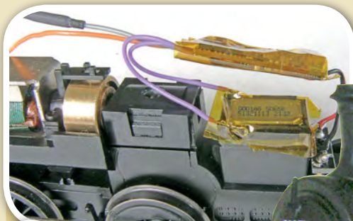
17 All the exposed metal parts of the speaker were insulated and the decoder was wrapped with kapton tape so the track pick-up wires 'appeared' at the end opposite to the normal arrangement. This helps to keep things neat and under control during reassembly.
