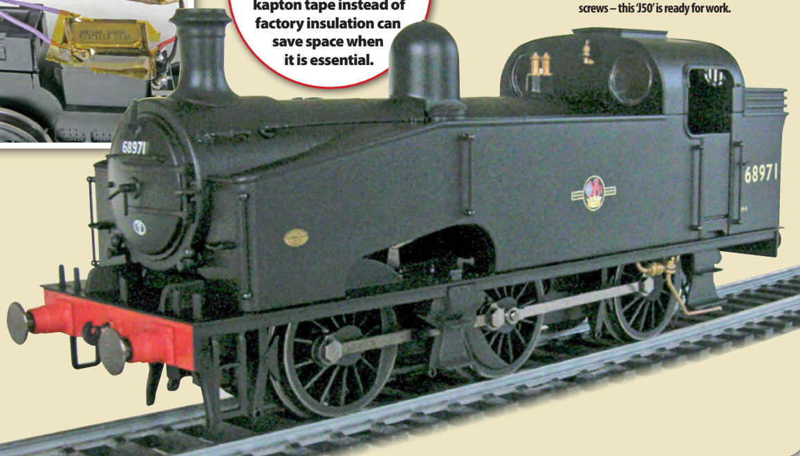
18 After refitting the body - ensuring that the sand pipe mouldings remain outboard of the coupling rods and replacing the fixing screws - this 'J50' is ready for work.
