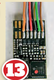
13 I removed the heatshrink insulation from the MX648 to reduce overall thickness and gain access to the soldered wires.
