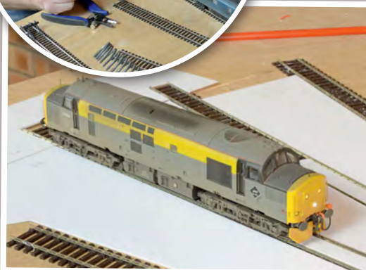
Above: Even on a quick build testing is essential – we still want everything to run smoothly when finished. A Bachmann Class 37 is used to check clearances with the new plastic inserts.
