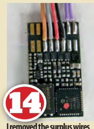
14 I removed the surplus wires from the decoder to reduce overall bulk, leaving only the track (red and black), motor (orange and grey) and speaker (purple) wires in place.
