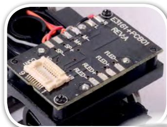
Above: The Next18 socket is compact in all dimensions. On the left is the socket with the factory blank in place while on the right is with the blank removed.
