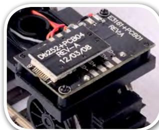
Above: The Next18 socket is compact in all dimensions. On the left is the socket with the factory blank in place while on the right is with the blank removed.
