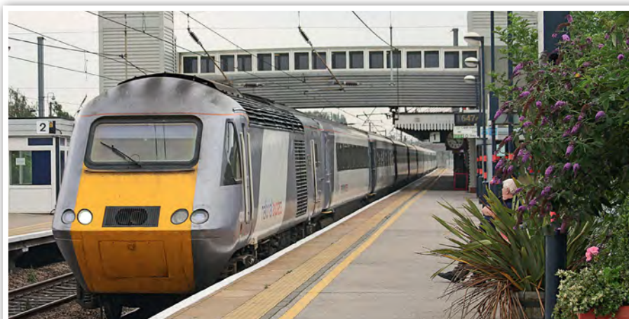
The most recent overhauls of the HST power cars have seen MTU engines installed to reduce emissions and noise. MTU powered 43310 thunders through Newark Northgate with the 2pm King's Cross-Aberdeen on July 22 2008. John Chalcraft/Railphotoprints.co.uk.
