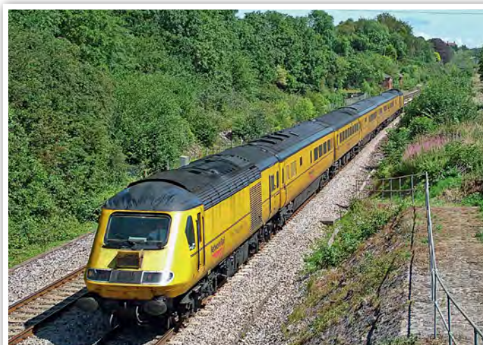
The Network Rail New Measurement Train is powered by cascaded Class 43 power cars which have been repainted in the bright yellow livery and modified with cameras on the cab fronts. Led by 43014, the New Measurement Train passes the site of Flax Bourton station as it heads west from Bristol on August 7 2004. John Chalcraft/Railphotoprints.co.uk.
