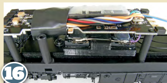
16 The speaker was fitted to the ballast weight on the floor of the chassis and the decoder end was wrapped with black tape to secure it in position and to disguise the view of the wires through the exhaust ports - not obvious until the body has been refitted.
