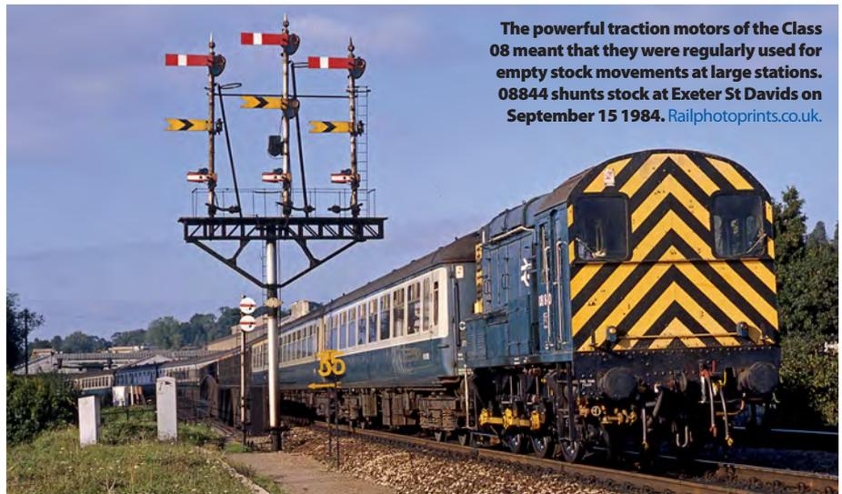
The powerful traction motors of the Class 08 meant that they were regularly used for empty stock movements at large stations. 08844 shunts stock at Exeter St Davids on September 15 1984. [Railphotoprints.co.uk](http://Railphotoprints.co.uk)
