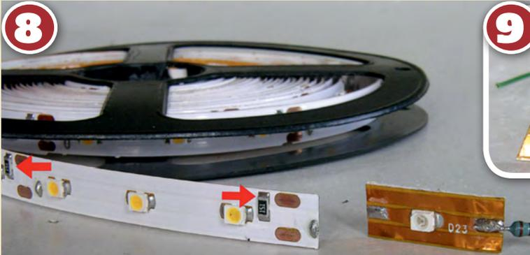
If you use LEDs regularly, rolls of 100 pre-connected LEDs are an economical way to buy them. The interconnecting copper traces make them convenient to use. Normally they have a Surface Mount Device (SMD) resistor for every three LEDs. The strips can be cut with scissors to isolate single LEDs. Make sure that there is a resistor in series with any LED used, either the fitted SMD resistor (arrowed in red) or by adding one if necessary, as shown on the right.
