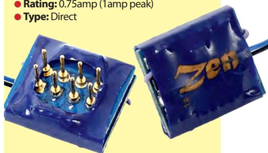
This tiny ZEN 360 direct plug decoder forms part of DCC Concepts' range of 8-pin DCC motor control decoders, designed to suit models where available space is at a premium.
