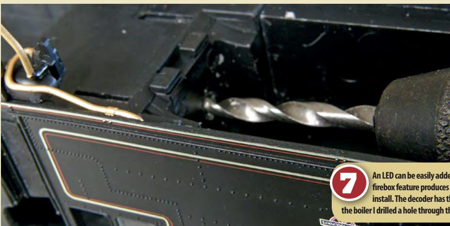
**7** An LED can be easily added. When linked to the sound of coal shovelling, a flickering firebox feature produces a pleasing effect far in excess of the cost of parts or the time to install. The decoder has this lighting effect on board, so it is as shame not to use it. From the boiler I drilled a hole through the firebox doors large enough to allow an amber LED to be fitted.
