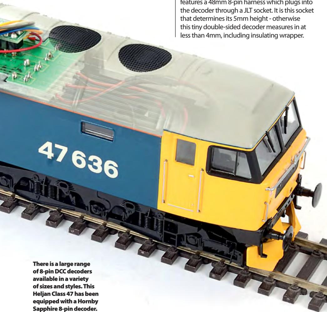
There is a large range of 8-pin DCC decoders available in a variety of sizes and styles. This Heljan Class 47 has been equipped with a Hornby Sapphire 8-pin decoder.
