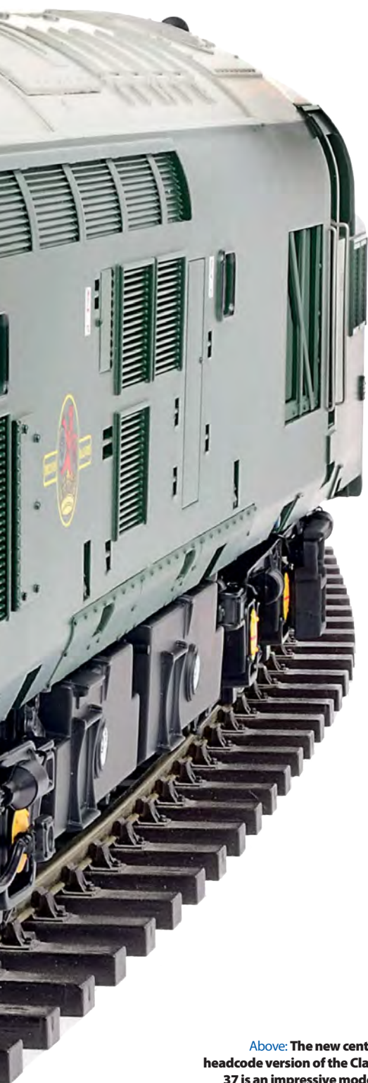
Right: The bogie side frames are neatly detailed and include separately fitted cab steps and painted axlebox covers.
