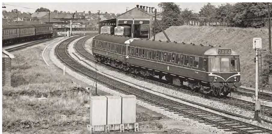
A fleet of dedicated Class 149 trailers were built to operate with the single car Class 121 and 122 units at peak periods. On July 25 1965 a Class 121 propels a 149 as it leaves Slough on a branch service to Windsor and Eton Central. Brian Stephenson.
