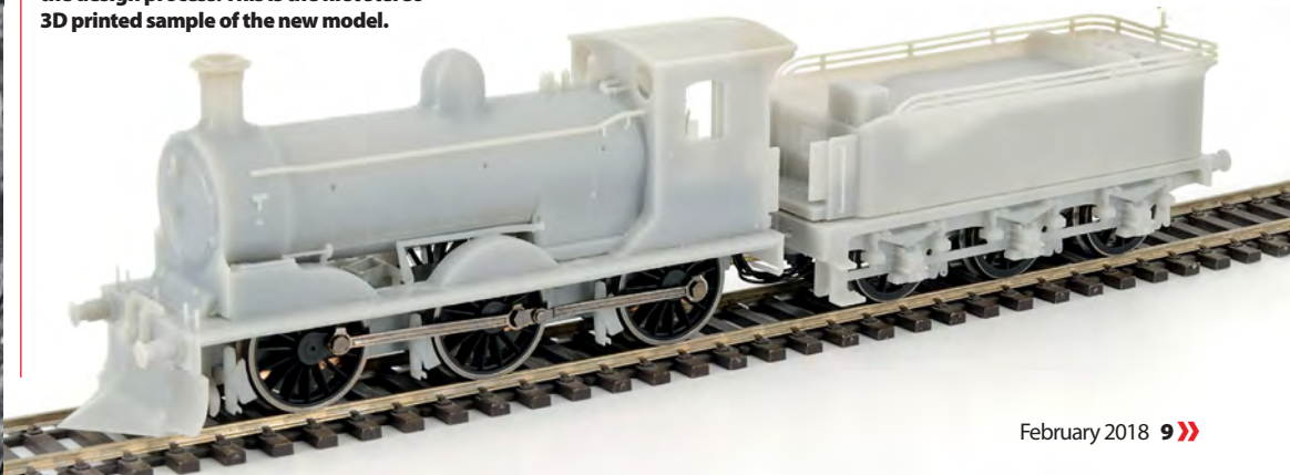
The Hornby 'J36' is progressing through the design process. This is the first stereo 3D printed sample of the new model.
