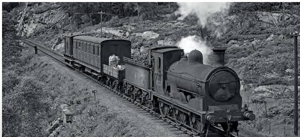
Holmes 'J36' 0-6-0 65237 heads a permanent way train on the Mallaig Extension beside Loch Nan Uamh between Arisaig and Lochailort in June 1955. These 1887 introduced 0-6-0s are being produced in 'OO' by Hornby in 2018.
