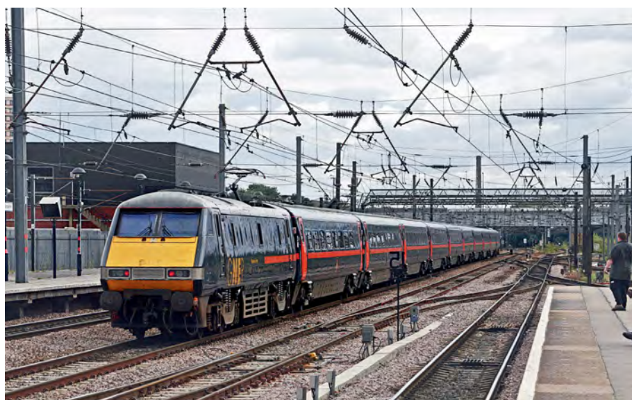
The East Coast Main Line uses a lightweight electrification design with wires used for spans in place of previous steel work. Class 91 91107 propels the 2.05pm Leeds-King's Cross service south through Doncaster on August 10 2006. Railphotoprints.uk.
