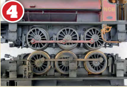
4 A wheel comparison between the DJ 'J94' and the older Hornby one. Note the difference in the depth of flanges, DJ's chassis having much finer and accurate wheel profiles.
