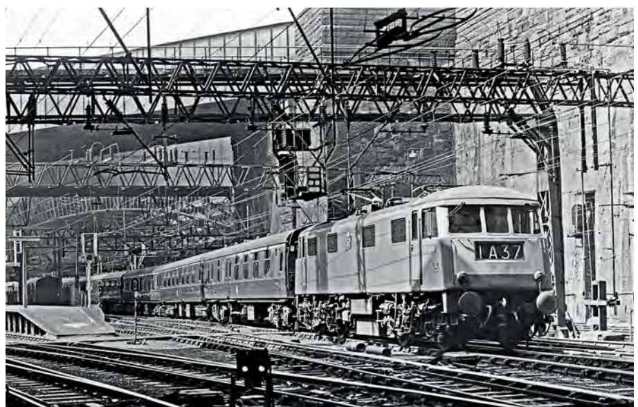
On the West Coast Main Line, English Electric built Class 83 E3099 leaves Liverpool Lime Street with 1A37 for Euston in August 1965. This area uses lattice frame gantries to support the overhead wires in the complex station throat. Colin Whitfield/Railphotoprints.uk.
