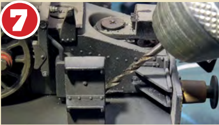
7 For ease it was decided that the connection would be at the front of the locomotive and it would arrive and depart with a brake van in tow. A hole for the lead to a miniature plug was drilled at an angle behind the front steps into the smokebox and the leads threaded through.
