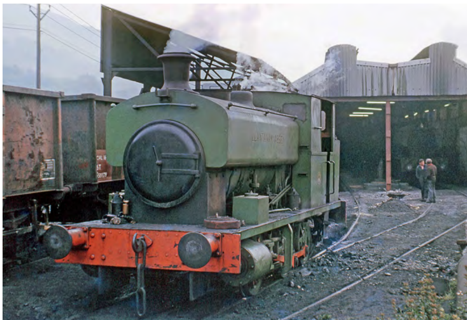
While 0-4-0STs were Andrew Barclay's best known product, larger 0-6-0STs and 0-6-0Ts were also built. NCB East Wales Area Andrew Barclay 0-6-0ST 2074, built 1939, stands outside its shed at Mountain Ash on November 1972. Railphotoprints.uk .
