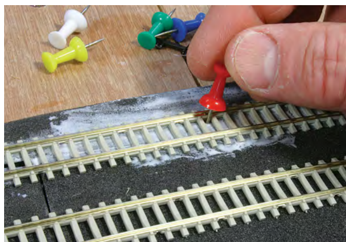
Map pins are a useful tool for holding flexible track in place whilst glue sets if it needs a little more securing to retain its formation. Do not press the pins in too hard or the track may become distorted when the foam underlay is compressed.
