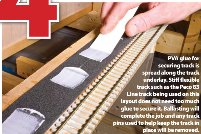
So far, so good. No rail joiners will be used at this point because the glue is holding the track well enough to keep the rail ends correctly aligned.
