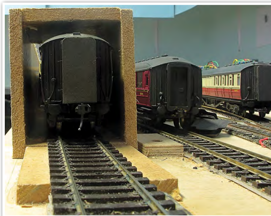
A cassette system has been developed to allow additional train formations to be stored off the layout. Each cassette can hold up to four carriages and by joining a series of stock from different cassettes together a complete train can be assembled.
