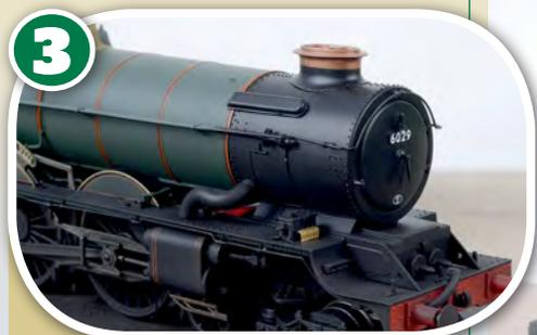
**3** The first step is to soften the colour of the underframe area. You can barely see it here, but a softly airbrushed coat of Burned Black (UA736) is enough to start toning down the factory fresh finish.
