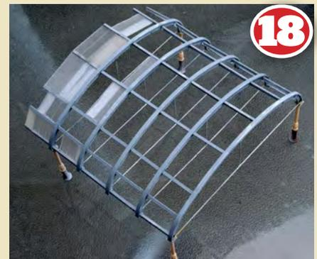
I cut up spare glazing sections using a circular saw in a mini-drill, then slotted them in place. At this stage the end roof section stands on temporary legs for support.
