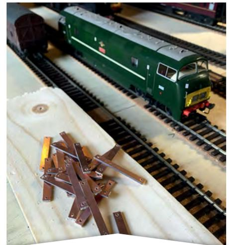
C&L Finescale copper clad strip was used for the securing sleepers. Supplied in lengths it was batch cut to length, drilled for track pins and finally the copper surface (on both sides) cut through to prevent short circuits.
