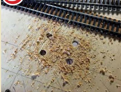
**4** Continue drilling holes with the same drill bit to fill in the gaps between the corner holes, then by angling the drill the holes can be fully connected to allow the centre to drop out.
