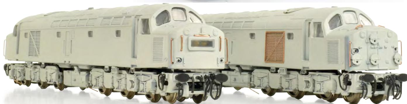
The 'N' gauge Class 40 will feature a Next18 decoder socket, provision for installation of sound and directional lighting too.
