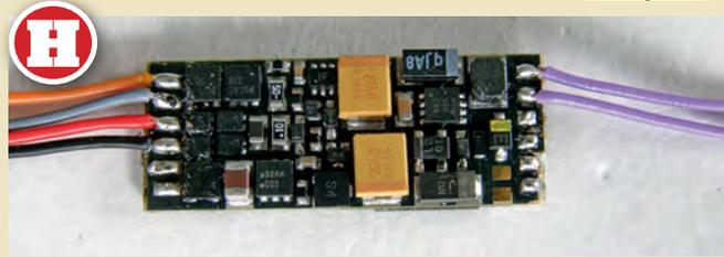
**H** I removed the unused function wires and added blue (positive) and grey (ground) to the two lower pads on the right of the picture.
