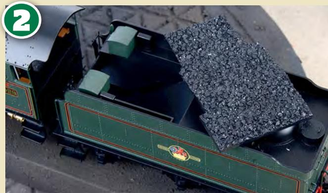
**2** A simple step, but one which is worthwhile, is removing the plastic coal load before starting. This allows weathering of the coal space. We also added the factory supplied detailing pack to the locomotive including brake pipes, brake rigging and cylinder drain cocks.
