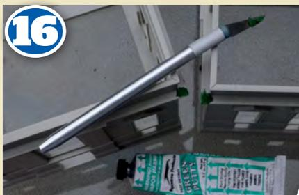
**16** There were very minor gaps at the tops of the walls, which I filled using Squadron green putty. Being flat, a blunt craft-knife blade acts like a spatula and is an ideal application tool. Once hardened off, the filler can be sanded smooth.
