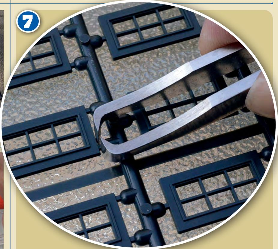
Sprue cutters, though very powerful, are more precise in action and the pincer movement means parts are unlikely to snap when being snipped off.
