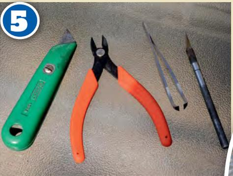
Cutting tools for working with plastic – a Stanley knife, Xuron cutters, sprue cutters (for nipping small parts from the moulding sprue) and a craft knife with an extremely sharp blade.
