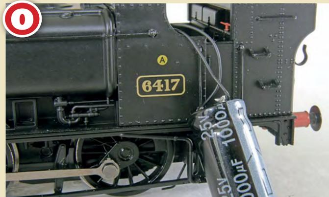
**O** After refitting the body and securing it to the chassis with the two screws removed earlier, I soldered the wires to the capacitor. I insulated with black tape which helps to disguise the capacitor's presence in the cab. Adding a crew will further hide its presence in the cab.
