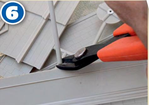
I begin assembly by using the side cutters to remove the main components. A Stanley knife does just as well but there's more risk of damaging yourself.
