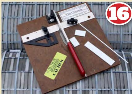
Creating the part-dismantled section at one end added individuality and was a good way of using up spare components such as roof braces and glazing panels. I made the extra girders I needed out of Evergreen styrene section cut to length using the guillotine-like Chopper from US company North West Short Line.
