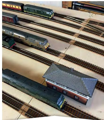
Sleepers were cut away from the track either side of each baseboard joint to make way for copperclad sleepers. The latter will secure the track ends at the baseboard joints.
