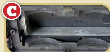
**C** The redesigned decoder socket removes the need for a cut out in the U-shaped ballast weight inside the pannier tanks. This space restriction results in the 'stay alive' capacitor being housed in the cab space.
