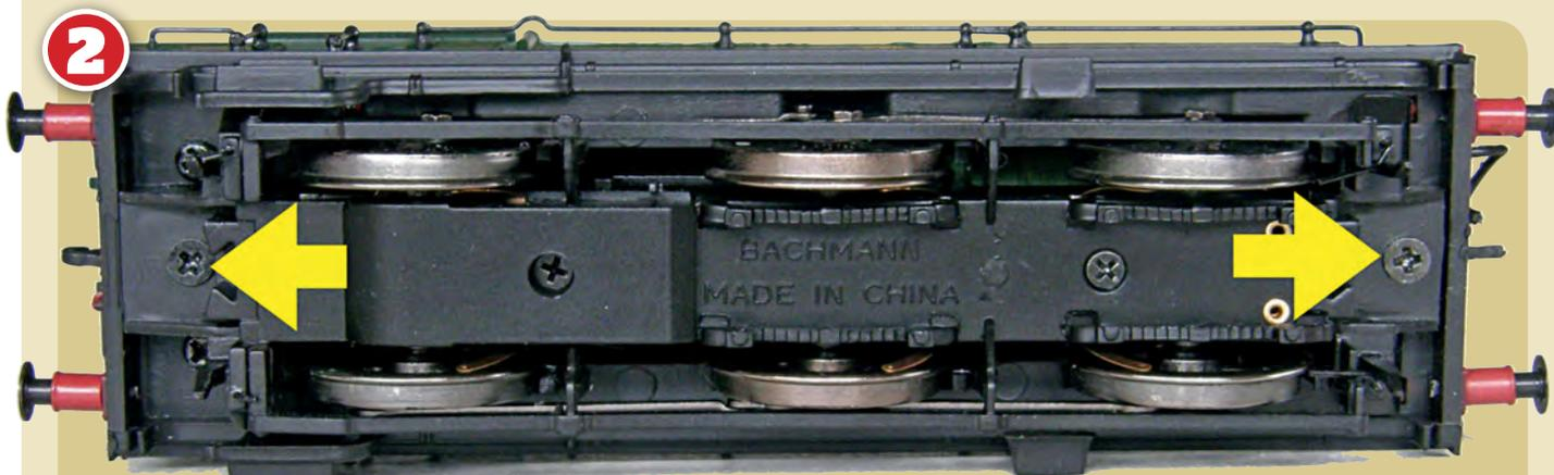
Remove the tension lock couplings for access to the body securing screws, arrowed. These should be released allowing the body to lift straight upwards and off.
