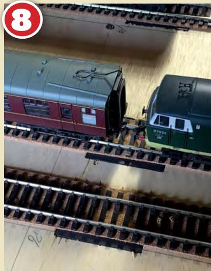
With Kadee couplings fitted to locomotive and carriage the magnets allow automatic uncoupling with the correct sequence of events. Happily, they won't uncouple trains when the couplings are under tension.
