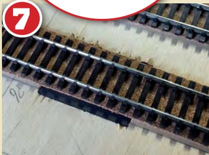
The track is then returned over the top of the magnet meaning that once ballasted the magnet below will be totally invisible.
