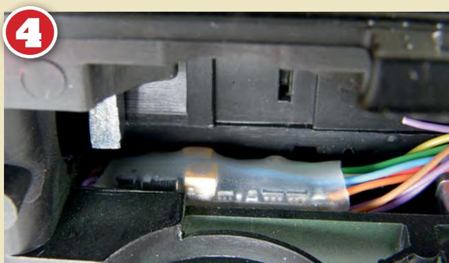
During a 'dry run' the Zimo MX649 can be seen fitting comfortably within this space even with the standard insulating sleeve in place. This sleeve will be removed to allow access to the solder pads.
