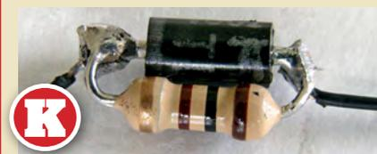
**K** The diode and resistor package was made as compact as possible to fit behind the speaker and alongside the MX649. I used black wires to connect to the capacitor as the rear ends will be passed through into the cab space. I used the convention 'long lead is the positive lead' to ensure correct polarity when connecting the capacitor later.
