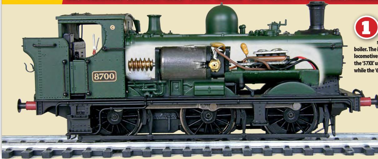
**1** The cutaway picture shows the small amount of usable space within the boiler. The internal design of both locomotives is similar, although the '57XX' uses an 8-pin socket while the '64XX' has a 6-pin socket.
