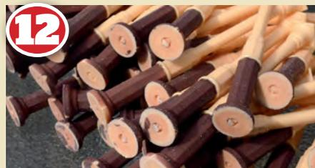
**12** The canopy supports are cut from their sprues and cleaned up as necessary. Remember to file the bases smooth, otherwise they won't sit properly.
