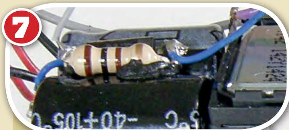
The capacitor charging control circuit consists of a series resistor and a diode, the anode of which should be connected to the positive lead on the capacitors. The anode is the end without a painted bar, in this picture the right-hand side. This is a compact package which will sit above and between the capacitors.
