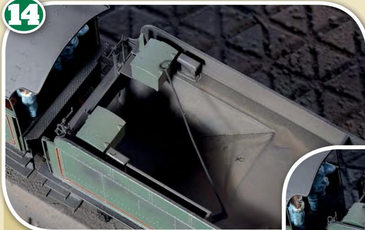
Fire irons are a small touch, but they were crucial equipment. Most are in the fire iron tunnel nearest the camera with one laying across the coal space.
