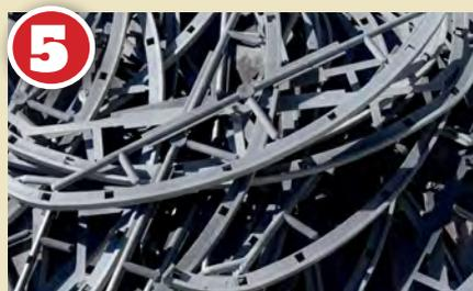
**5** The roof ribs were airbrushed light grey (Lifecolor UA603 Hellgrau again) to represent the metallic grey paint so often seen on such structures. In 4mm scale you don't need any metallic sparkle.
