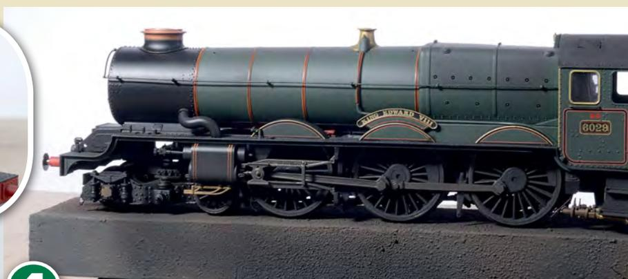
**4** The wheels, motion and front bogies are all touched up by the Burned Black together with the cab roof.
