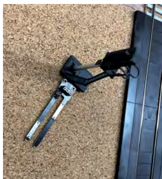
As delivered the Train-Tech sensor signals are designed to be plug and play. The two prongs slide under the rails between the sleepers to take power and position the sensor correctly alongside the track.
