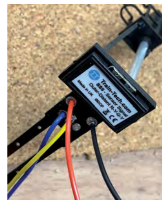
Rather than use the prongs to collect power we soldered red and black wires to the optional DCC power connections on the circuit board.
