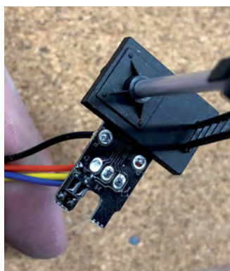
The prongs were then cut back to the markers on the legs completing modification of the wiring of the signal prior to installation.
