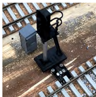
The signal was then glued in place on top of a small square of cork to make it level with the trackbed. The black and red wires were then connected back to the DCC power bus and the blue wire linked through to the next signal as per Train-Tech's instructions.
