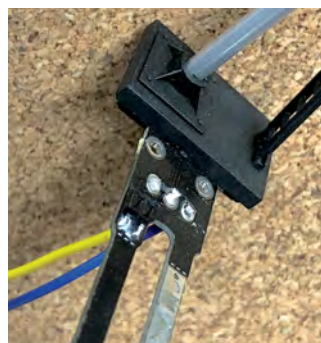
We then connected a yellow wire to the central pin (which can be used to connect to a mimic switch in the future if required) and a blue wire to the rear pin to link through to the next signal to control sequencing of the signal aspects.
