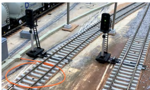
Train-Tech four-aspect colour light signals have been used for all the main line signals. Here we are testing the signals before modifying the wiring as described in the separate panel on page 15.
