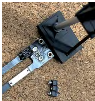
To allow the sensor wiring on our signals to pass underneath the baseboard we unsoldered the three-pin plug from each signal's circuit board. This needs to be done carefully to avoid any damage to surrounding tracks on the board.
