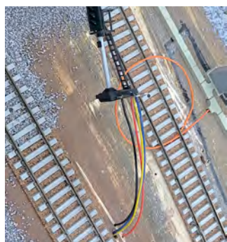
Two 2mm holes were drilled for the red and black wires and a pair of 2.5mm holes were joined together for the blue and yellow wires to pass through the baseboard. The orange wire here is cosmetic.
