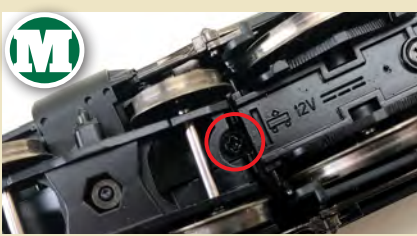
At the front of the air-smoothed model you need to remove the front bogie first to gain access to the front body fixing screw. Remove the single crosshead screw which holds the bogie in place.
