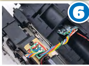
As before, we plug the decoder into the socket by aligning the orange wire with Pin 1 on the circuit board and the decoder can be tucked into the smokebox for a neat installation.
