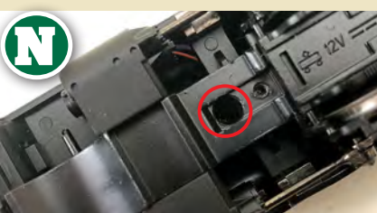
The front body fixing screw is located just behind the cylinders in a recess. It is a crosshead of the same pattern as the rear fixing screw.
