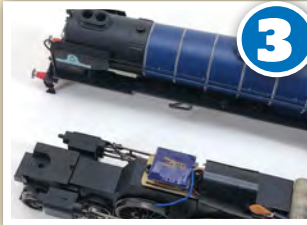
Both the Gaugemaster DCC29 and DCC Concepts Zen direct decoders fit comfortably inside the 'A1' boiler and provide a very neat decoder installation.
