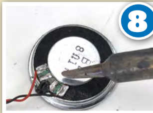
Disconnect the black and red wires from the factory fitted speaker by heating the connection points with a soldering iron briefly until the solder melts and the wires can be pulled away.
