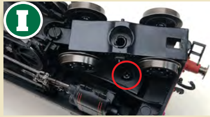
Locomotive body removal is optional for decoder installation. The body fixing screw is located under the front bogie on the rebuilt 'MN'. Turn the bogie to one side for access to the crosshead screw.
