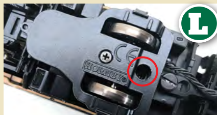
While the tender fixing points are identical on both the air-smoothed and rebuilt locomotives, the locomotive body fixing screws are in different positions on the new 2017 released air-smoothed models. The first screw is located at the rear of the trailing truck, buried into the casting.
