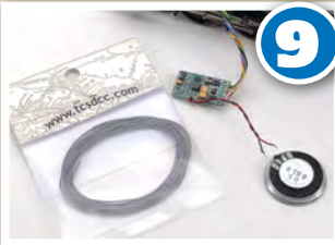
We are using TCS decoder wire from www.digitrains.co.uk to extend the speaker cables. Polarity isn't important and we recommend black wire for a neat installation without the need to paint the cables.
