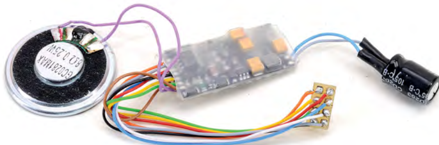
The Zimo decoder brand includes the MX645R (left) 8-pin decoder and the MX644D 21-pin decoders. These are supplied without speakers, leaving the customer to make their own choice to suit the installation. This MX645R has been connected to a 28mm round speaker and a 'stay alive' capacitor.
