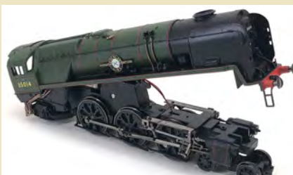
The body lifts up from the front until the rear lugs disengage. If you have already fitted your model with front steps and brake rigging, take care handling these areas as it is easy to knock these parts off.
