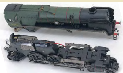
With the decoder socket now located in the tender, the locomotive only contains the motor and gearbox as well as a pair of connections to the track pick ups.
