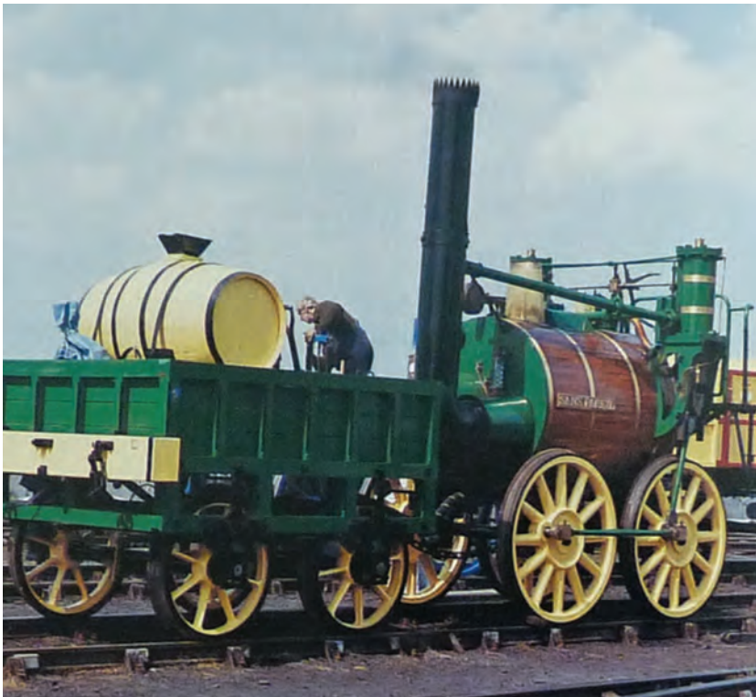
Sanspareil replica , built by Shildon Works apprentices for the 1979 re-enactment of the Rainhill Trials (picture courtesy Jane Hackworth-Young).
