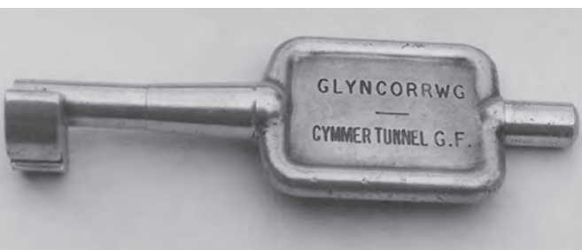
The Token for the section between Cymmer Tunnel Ground frame and Glyncorrwg. Once released, this precluded any unauthorised movement between Caerau and Cymmer. (Stuart Davies)
