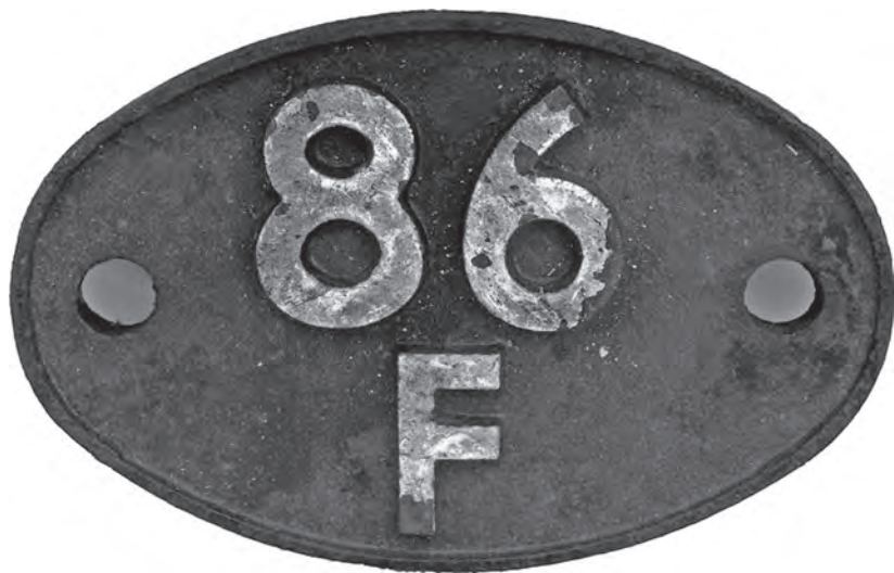
The GWR shedcode for Tondy was TDU. The practice was to stencil this on the footplate side frame immediately behind the front buffer beam or on the top of the front step plate. In 1950 the former LMS system was used whereby a cast iron plate was affixed to the bottom of the smokebox door. Tondy became 86F, the 8 denoting Western Region and the 6, a Newport District shed. Reorganisation from 1 January 1961 saw the transfer of Tondy Depot to the Cardiff Valleys District and Tondy now became 88H.
