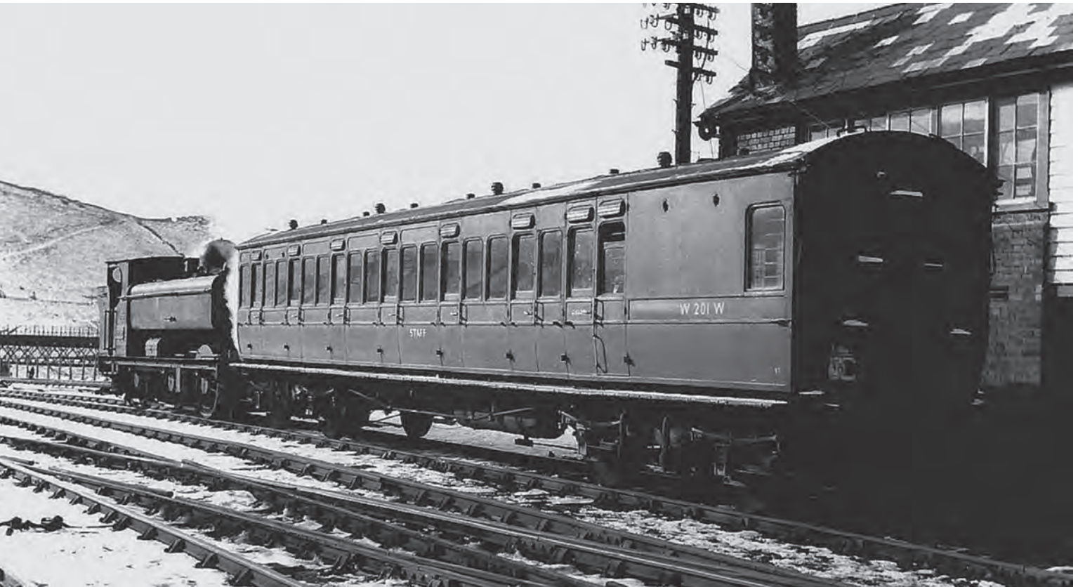
A miners' service to Duffryn Rhondda Colliery, a short distance south of Cymmer on the R&SB line, departs on a snowy day '21 February 1955' with engine 5789 of Duffryn Yard and former Taff Vale railway 331, an 8-wheel Brake Third built at Cathays in 1903, here renumbered as W201. It was converted by the TVR to an Auto Brake Third in December 1910, the GW re-converted it to a Brake Third in 1924 as 2488 and then downgraded it to Workmen's Brake Third in October 1949. It was renumbered W201 in October 1950 and remained in service until August 1959. (Ian L. Wright)
