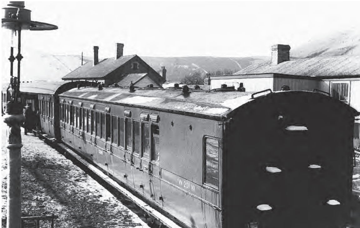
A miners' service to Duffryn Rhondda Colliery, a short distance south of Cymmer on the R&SB line, departs on a snowy day '21 February 1955' with engine 5789 of Duffryn Yard and former Taff Vale railway 331, an 8-wheel Brake Third built at Cathays in 1903, here renumbered as W201. It was converted by the TVR to an Auto Brake Third in December 1910, the GW re-converted it to a Brake Third in 1924 as 2488 and then downgraded it to Workmen's Brake Third in October 1949. It was renumbered W201 in October 1950 and remained in service until August 1959. (Ian L. Wright)
