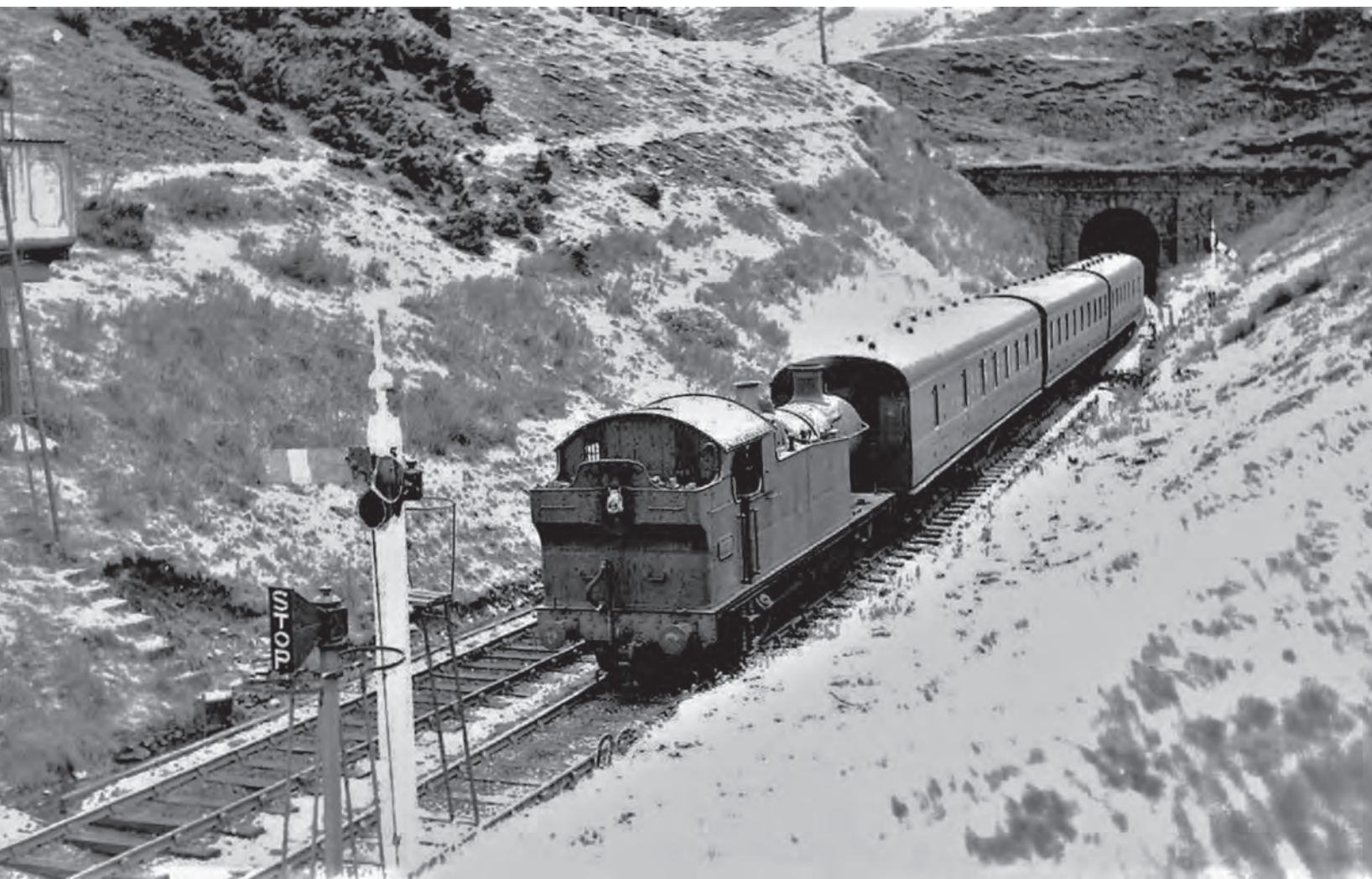
A three-coach Treherbert to Swansea service leaves the tunnel behind 6680. The engine will have shut off steam to run through the tunnel, hence no residue behind the train.
