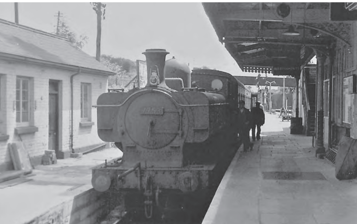
The gradient from Cymmer to Blaengwynfi was easier than to Abergwynfi and enabled the replacement of 4575 small Prairie tanks with the less powerful though also Auto-fitted 64XX Pannier Tanks. Auto fitted 5555 is seen at Bridgend in August 1960 one month before all the 4575s left Tondy for the last time. She is standing on the back road alongside the Valleys platform road. The yard below was used by a company for car repairs and the street along the top was Llynfi Street. (D.K. Jones Collection)
