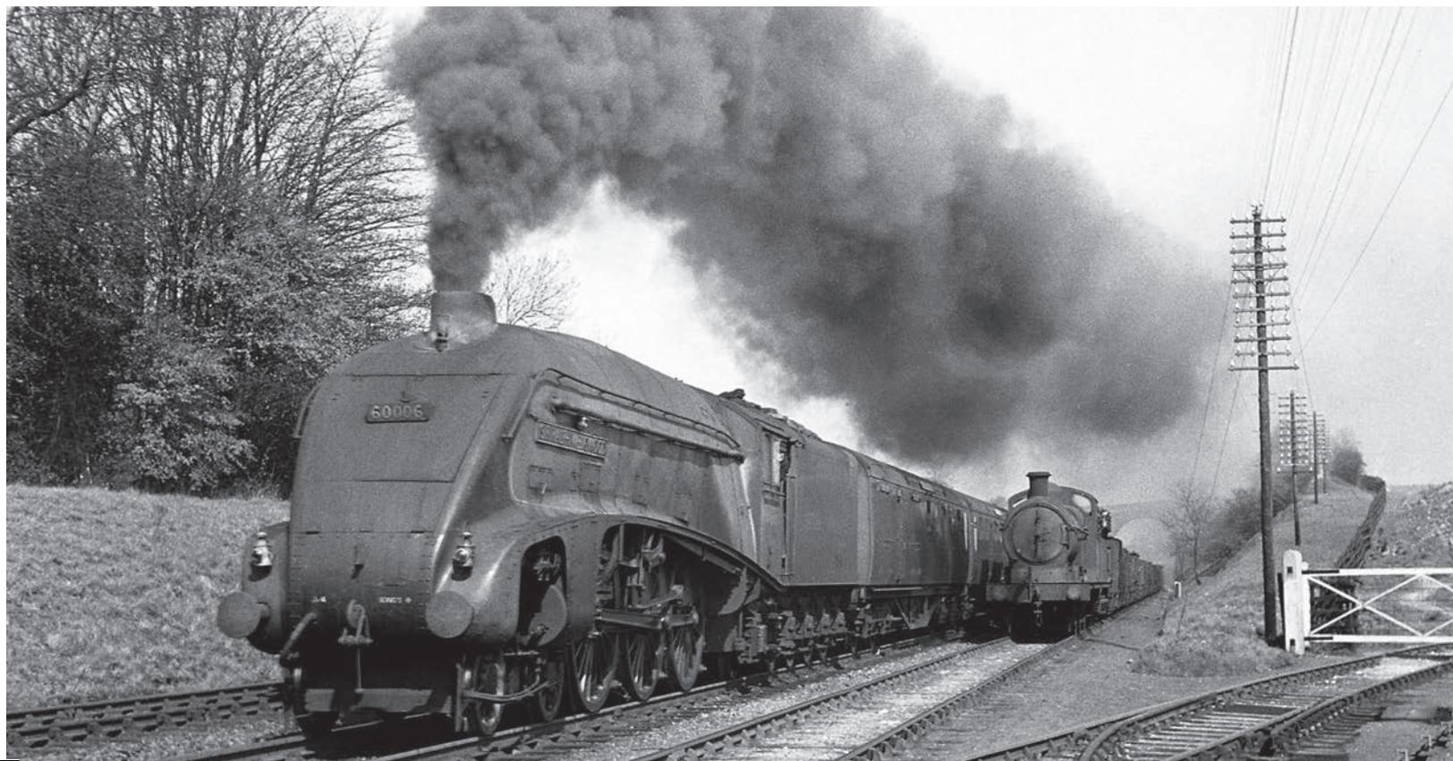
**60008 DWIGHT D. EISENHOWER** (LNER 4496, 8 – 1946 number) built at Doncaster Works, Order No 341 – Works No 1861. Entered traffic in September 1937 named **GOLDEN SHUTTLE**, renamed September 1945. Withdrawn by BR in July 1963 and saved for preservation. **P** Normally based at the National Railroad Museum of USA.
