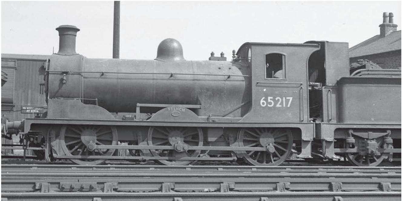
This view of BR No 65217 French shows the addition of a tender cab to good effect. The relatively open aspect of the 'J36' cabs afforded the locomotive crews limited protection from the elements. Many of the class were attached to snow ploughs and of those were fitted with tender cabs thus giving the crews much more protection. *Norman Preedy Archive*
