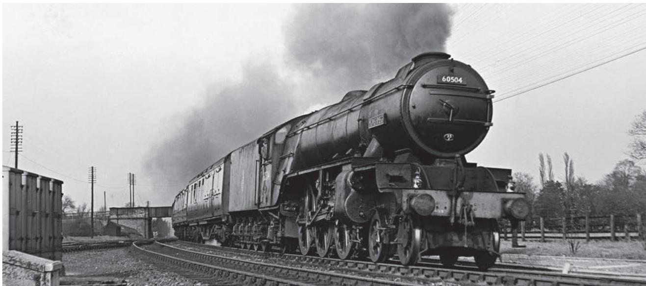
Thompson A2/2 Pacific BR No 60504 MONS MEG is seen passing Chaloners Wynn Junction near York on 11 April 1953. A Kylchap exhaust arrangement was fitted with lipped chimney, as well as small wing-type smoke lifters. The locomotive carries BR Green livery with an early crest on the tender. *Norman Preedy Collection*
