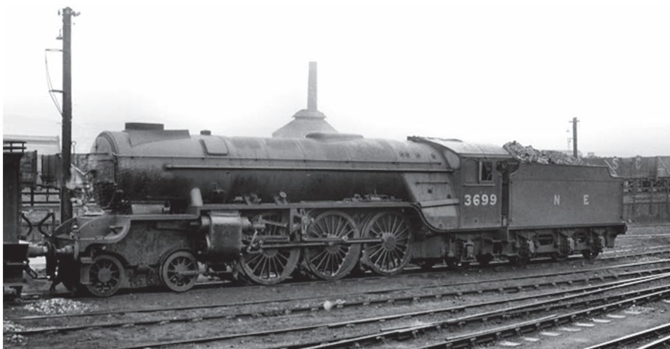
Thompson 'A2/1' class Pacific LNER No 3699 (BR 60510) is pictured adjacent to the ash pits at Edinburgh Haymarket depot in early 1945. Note the wing type smoke deflectors and ex-North Eastern 4,200 gallon 6-wheel tender. The locomotive was then un-named and seen before the completion of electric lighting installation. *Mike Morant Collection*
