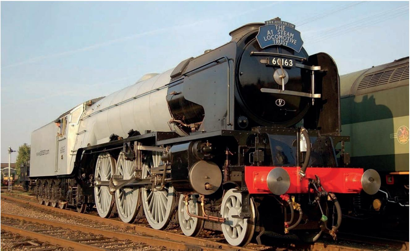
TORNADO is seen posed at the Great Central Railway in October 2008. Note the lipped double chimney and also the lighting generator located behind the right-hand smoke deflector. *Clive Hanley*
