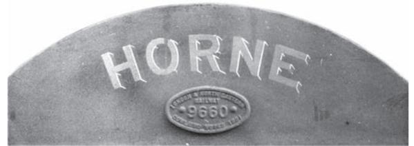
**LNER locomotive 'J36' class 0-6-0 BR No 65236 HORNE seen with the name painted on to the centre wheel splasher with a cast maker's plate mounted below. This Cowlairs Works built locomotive was one of 123 engines of this class introduced un-named between 1888 and 1900, which later came into BR stock. After the end of World War I some of the class received military associated names.**
