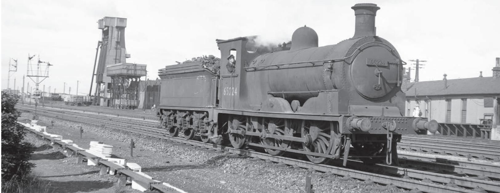
LNER 'J36' class BR No 65224 MONS is again seen at Haymarket. Note the impressive coaling plant, water tank and arrays of lattice work signal posts. In this 1956 image the locomotive is not fitted with a tender cab, but still has the connecting canvas sheet attached to the engine cab in place. *David Anderson*
