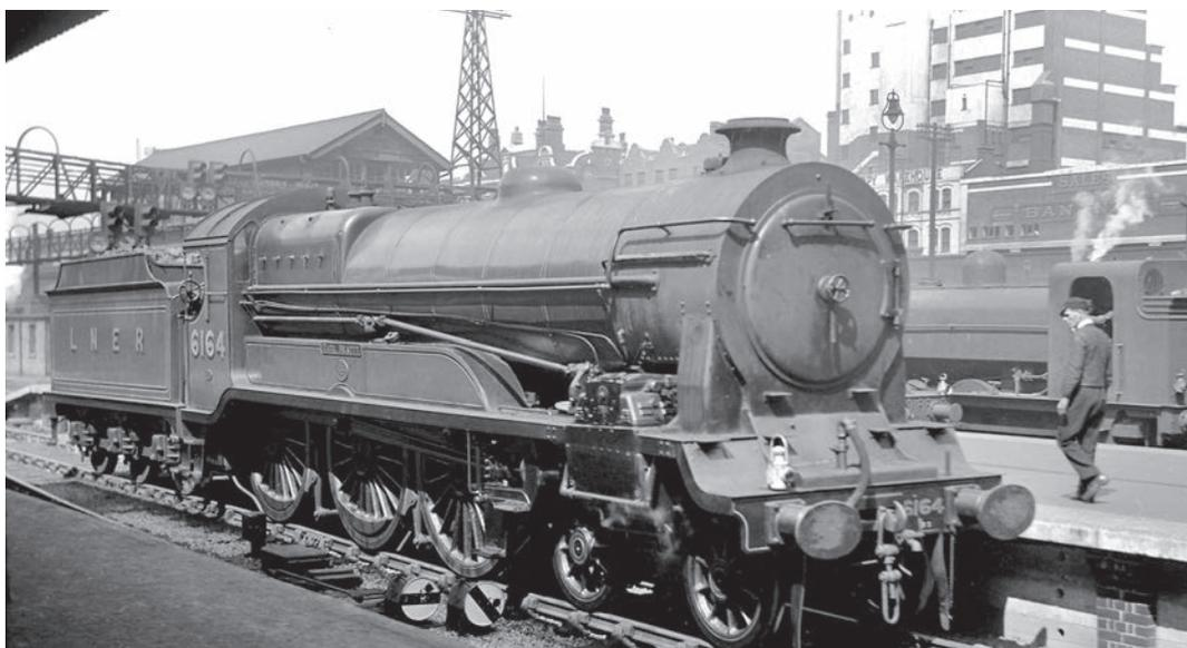
LNER 'B3/2' class LNER No 6164 EARL BEATTY is seen at Kings Cross station in August 1939 shortly after being converted to a Caprotti valve gear locomotive. Note the Ex-Great North Railway 'J52' class 0-6-0ST standing at the adjacent platform whilst on station pilot duties. *Rail Photoprints Collection*
