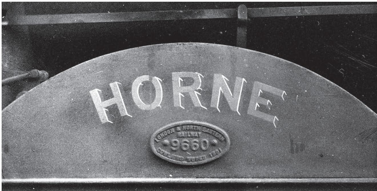
The centre wheel splasher of BR No 65236 HORNE with the stencilled locomotive name and Cowlairs Works makers plate. *Norman Preedy Archive*
