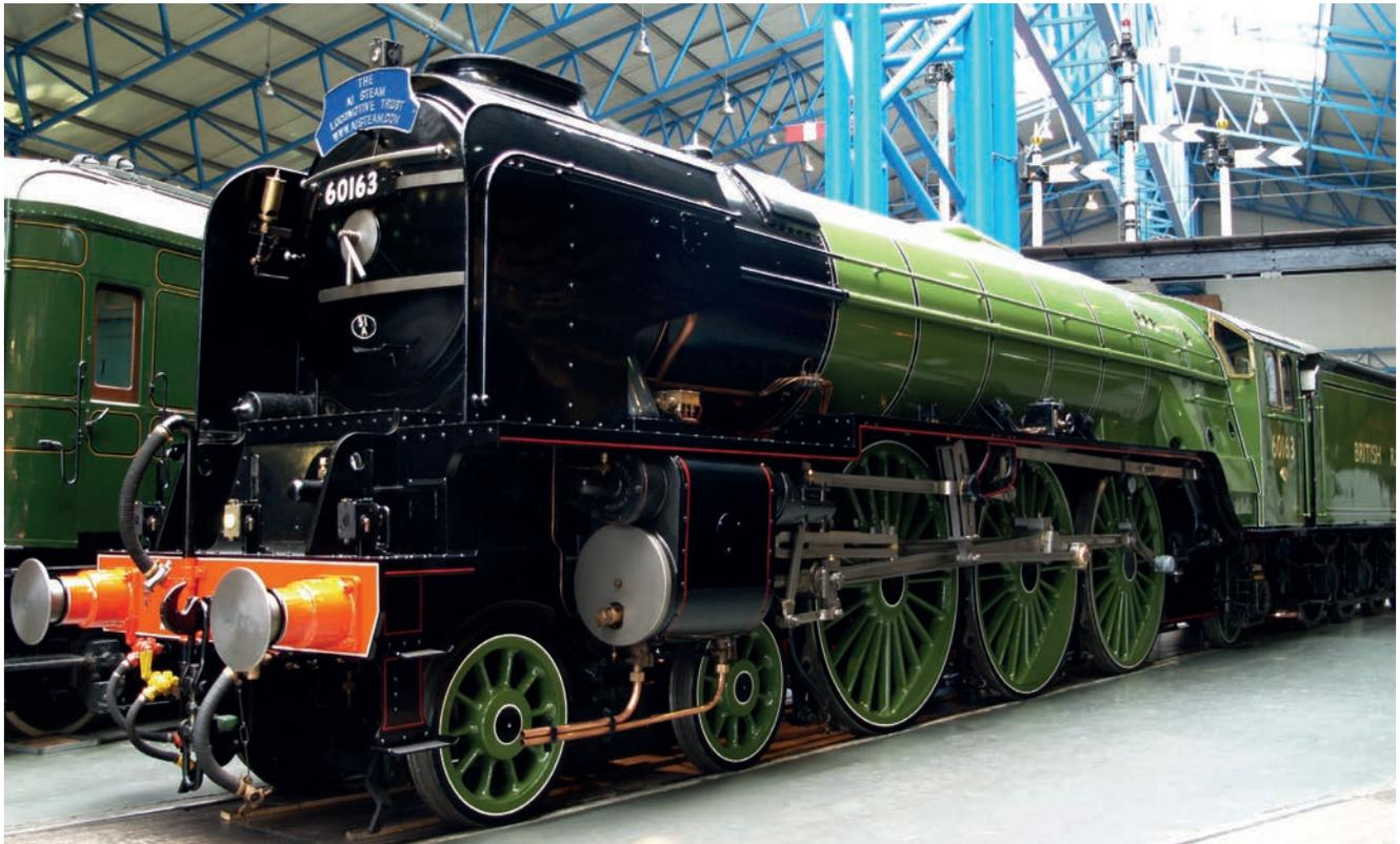
The new 3-cylinder A1 Trust Pacific with a lipped double chimney makes a fine sight as it stands in the display area main hall of the National Railway Museum having been given an LNER Apple Green livery on 1 January 2009, and prior to being named. The chime whistle and lighting generator can both be seen located inside the right-hand smoke deflector. Note the 51A Darlington shedplate. *Phil Brown*
