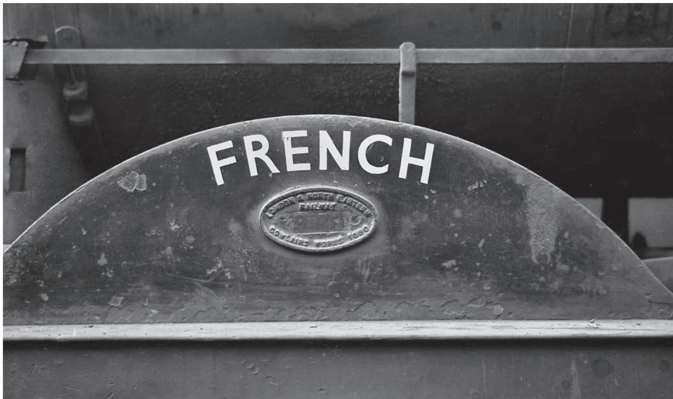
The name of locomotive BR No 65217 together with a Cowlairs Works LNER era makers plate can be seen in this image of the engines centre wheel splasher. *Keith Langston Collection*
