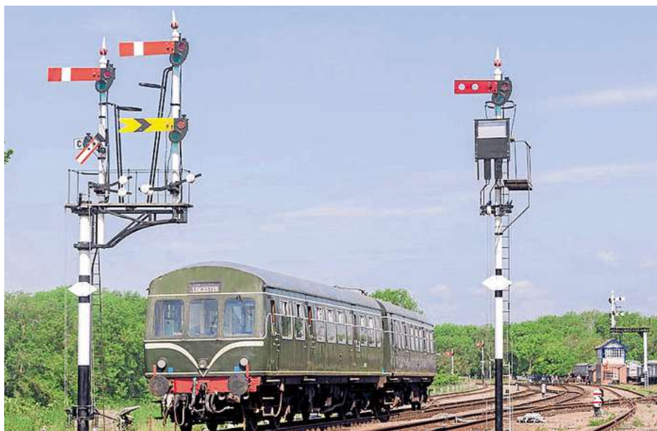
The GCR's resident Class 101 DMU was used to test the signalling at Swithland before commissioning on May 30, 2012. It is seen entering the Down loop using a 'calling on arm' on the Down home bracket. STEVE TAYLOR
