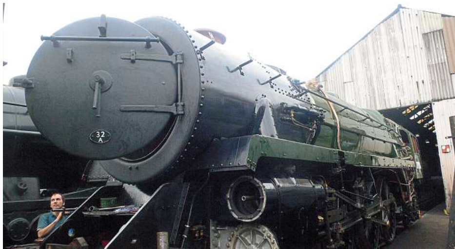
Out in the Loughborough sunshine for the first time since its repaint, Oliver Cromwell , minus its smoke deflectors, has its valves reset in late April 2008.
