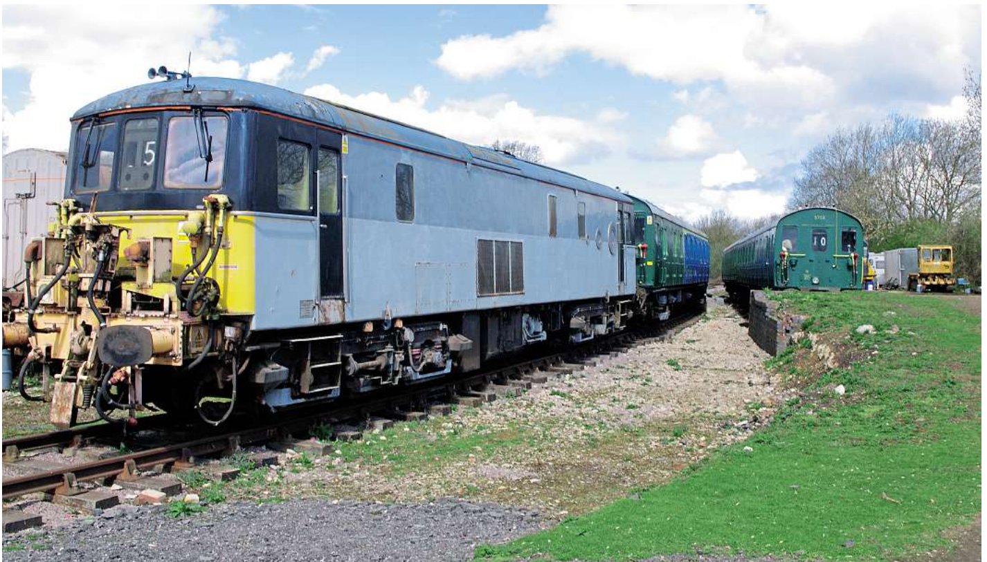
Class 73 electro diesel No. 73130 at Fimmere, still fitted with additional coupling equipment for hauling Eurostar units. ROBIN JONES
