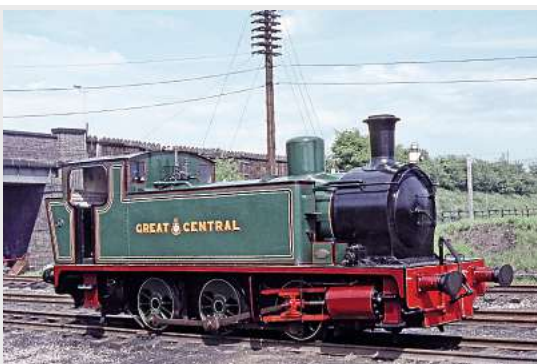
RSH 0-6-0ST No. 39 (6988), converted to a side tank in GCR livery, is seen at Loughborough on May 27, 1979. Industrial types were still in service on the line at this time. BRIAN SHARPE
