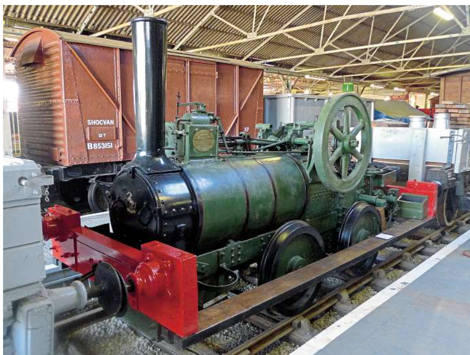
Great Central it ain't: Aveling & Porter flywheel-driven 0-4-0 No. 807, seen on static display inside the Quainton Road museum building, was one of a pair which worked on the Wotton Tramway, later known as the Brill branch. Supplied in January 1872, it had a maximum speed of 4mph. Both were withdrawn in 1894 and replaced by two Manning Wardle K-Class saddle tanks. No. 807 then worked at the Nether Heyford Brickworks in Northamptonshire, which closed in 1940. After being bought by the Industrial Locomotive Society, in 1951 London Transport agreed to store it at Neasden Depot. In 1957 it was officially handed over to the British Transport Commission for display at the former Museum of British Transport, Clapham, and in 1980 arrived at the London Transport Museum in Covent Garden. ROBIN JONES
