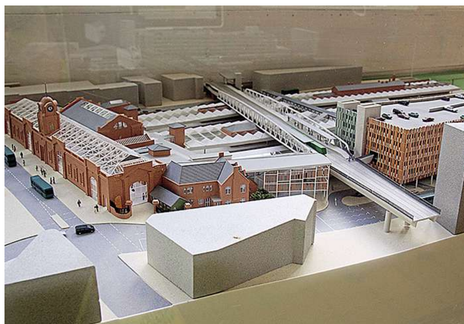
A model of the new bridge taking the tramlines across the top of Nottingham station. NET
