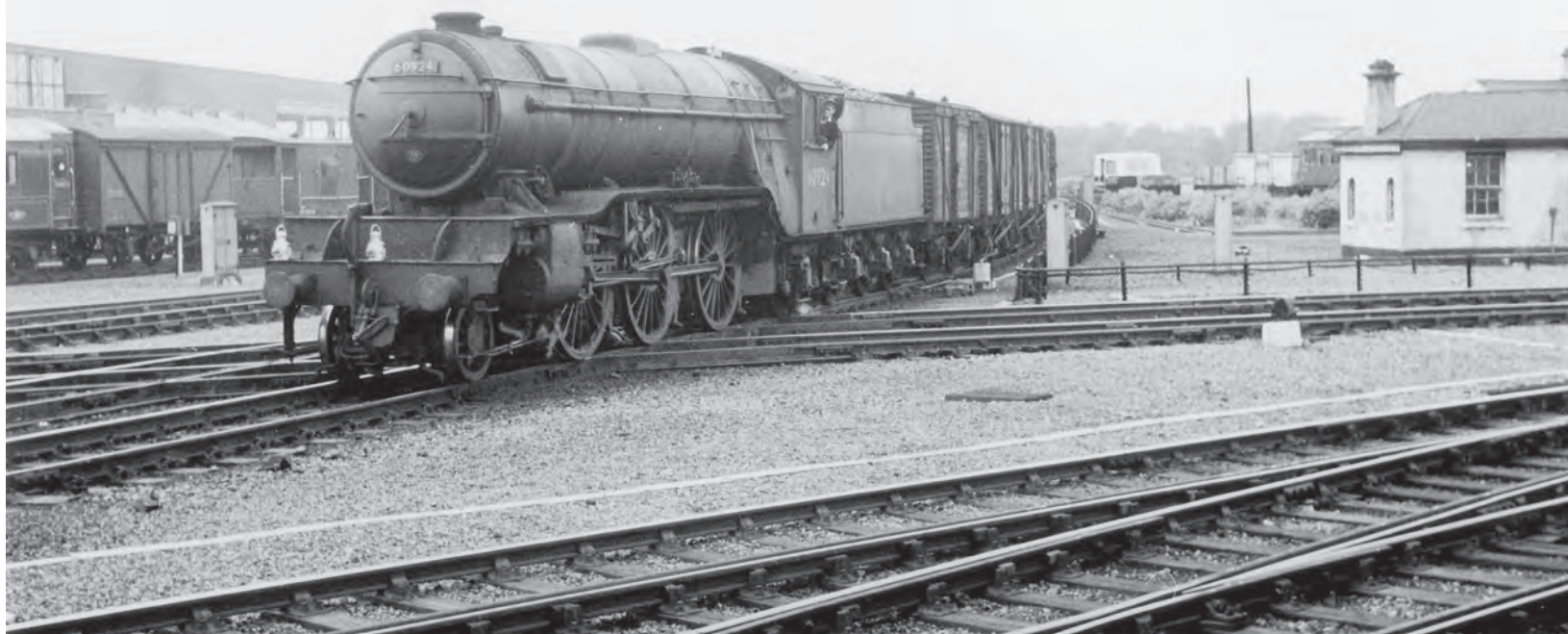
A southbound fast freight is about to thread its way through York station, headed by Gresley 'V2' 2-6-2 60924, a Doncaster resident. It is astride Waterworks Junction where the East Coast Main Line meets the line to Scarborough, disappearing to the right of the picture. 7 August 1962.
