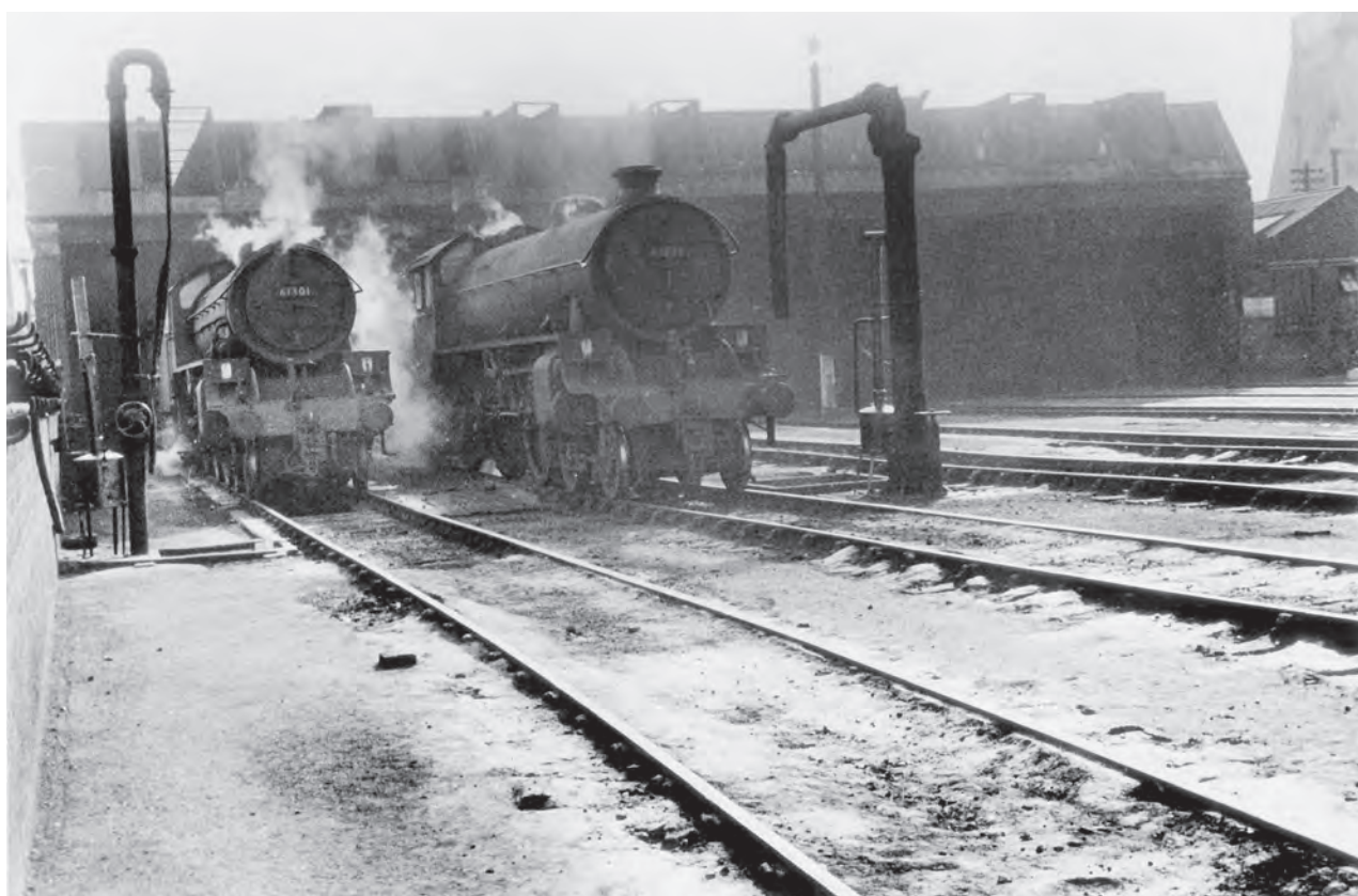
'K1' 2-6-0 62040 has emerged to have its tender replenished, with a crew member watching the water level rise.
