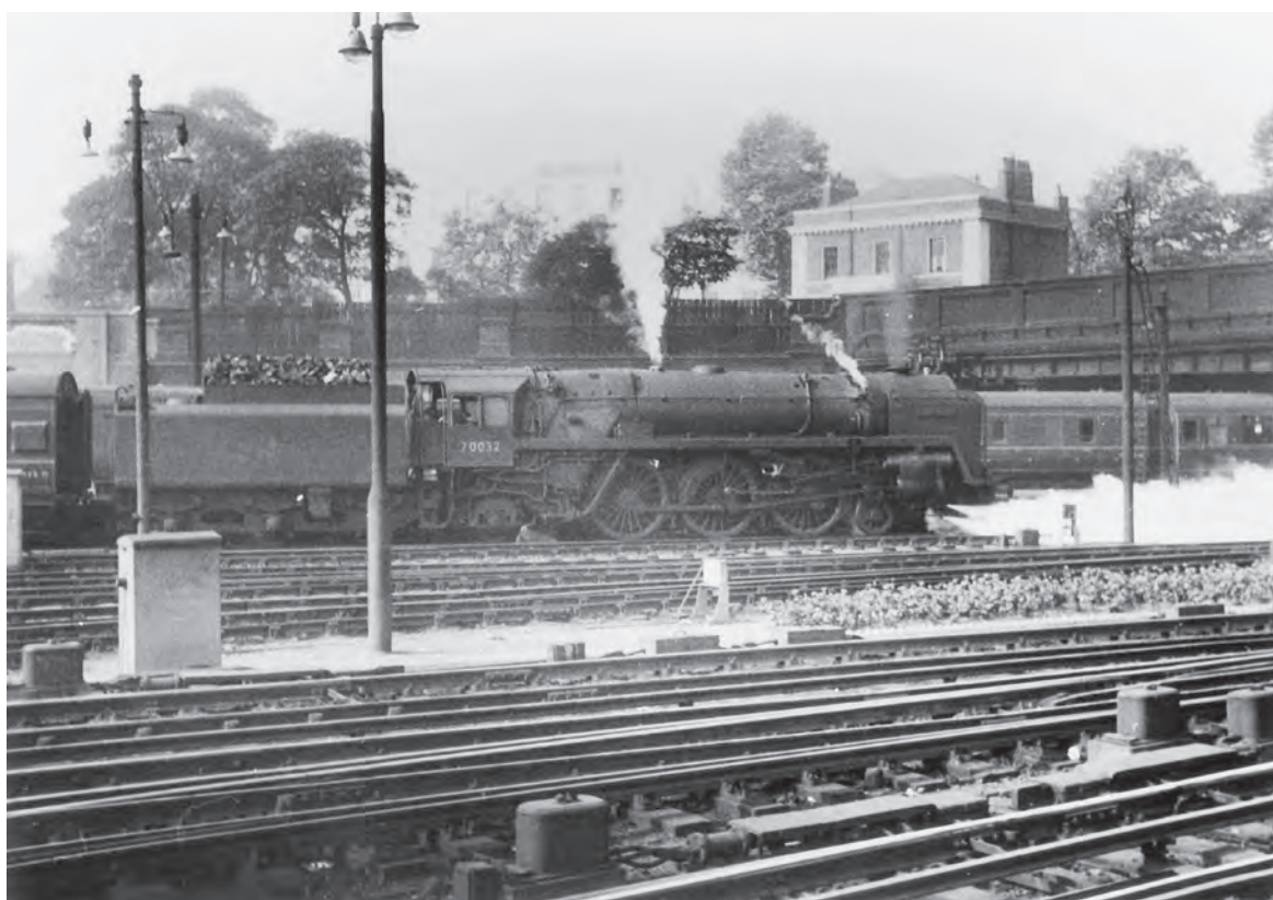
Longsight based 'Britannia' pacific 70032 Tennyson is about to leave Euston with an express for Manchester. The steam cocks have been opened and steam pressure is on the red line. Behind the tender is an ex-LMS brake vehicle. The electric lines for the Watford suburban trains are in the foreground. 12 September 1959.
