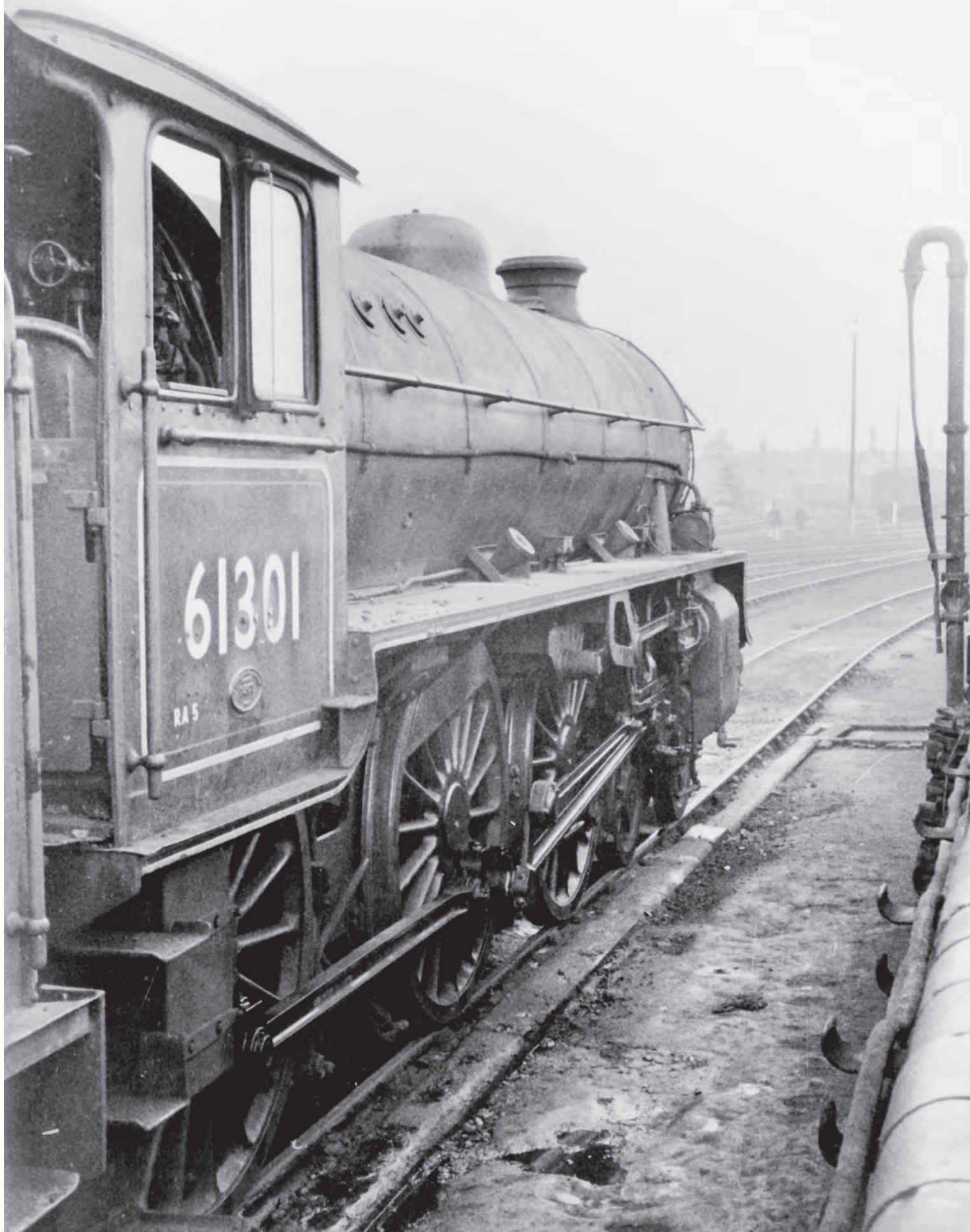
Resident 'B1' 4-6-0 61301 is at rest by the wall dividing the platform from the running shed.
