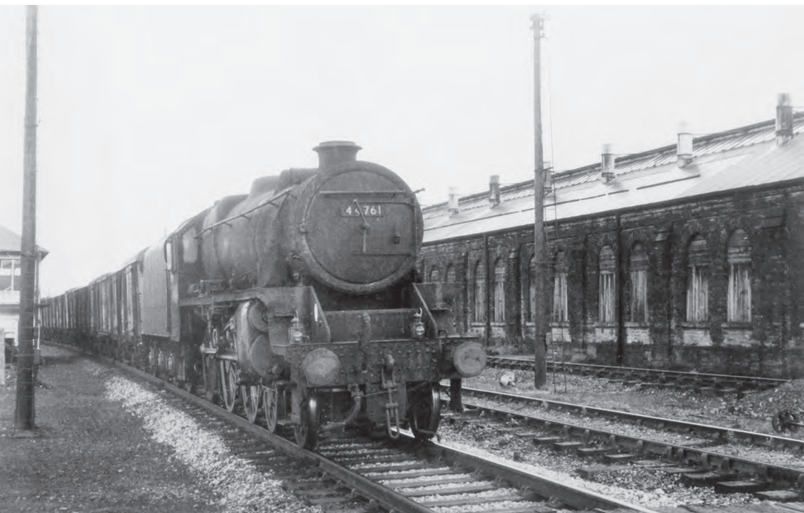
Stanier '5MT' 4-6-0 44761, from Springs Branch shed, is bringing its southbound freight to a halt at Hellifield, passing the closed locomotive shed in the process.
