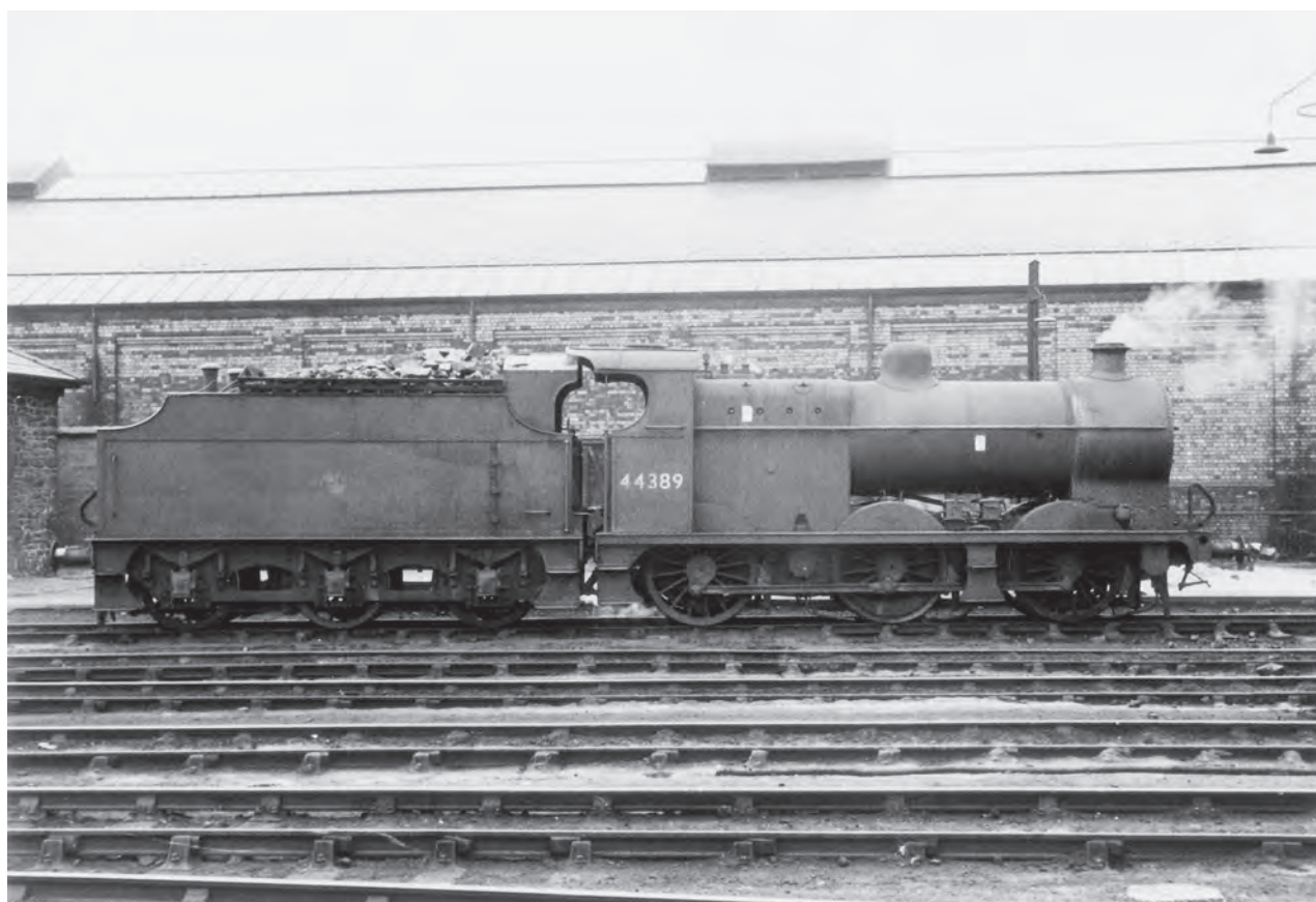
Outside the shed, '4F' 0-6-0 44389 is in steam awaiting its next turn. The tender is well filled with coal and note the tender cab to give the crew protection for tender first working. 8 June 1964.
