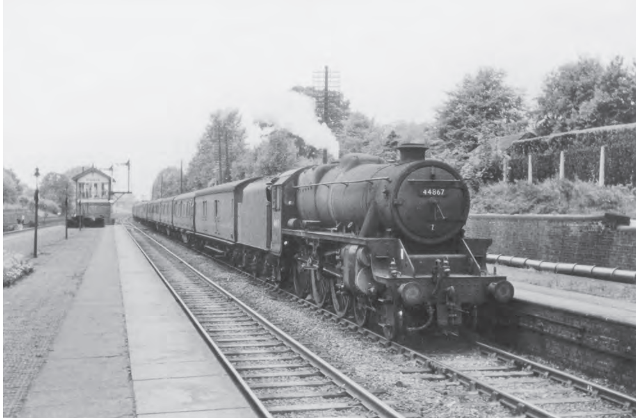
Rugby shed's Stanier '5MT' 4-6-0 44867 is heading a lengthy parcels and van train through Hatch End's up slow line platform. The locomotive is taking it easy in a queue of up trains. Note the bull head rail.
