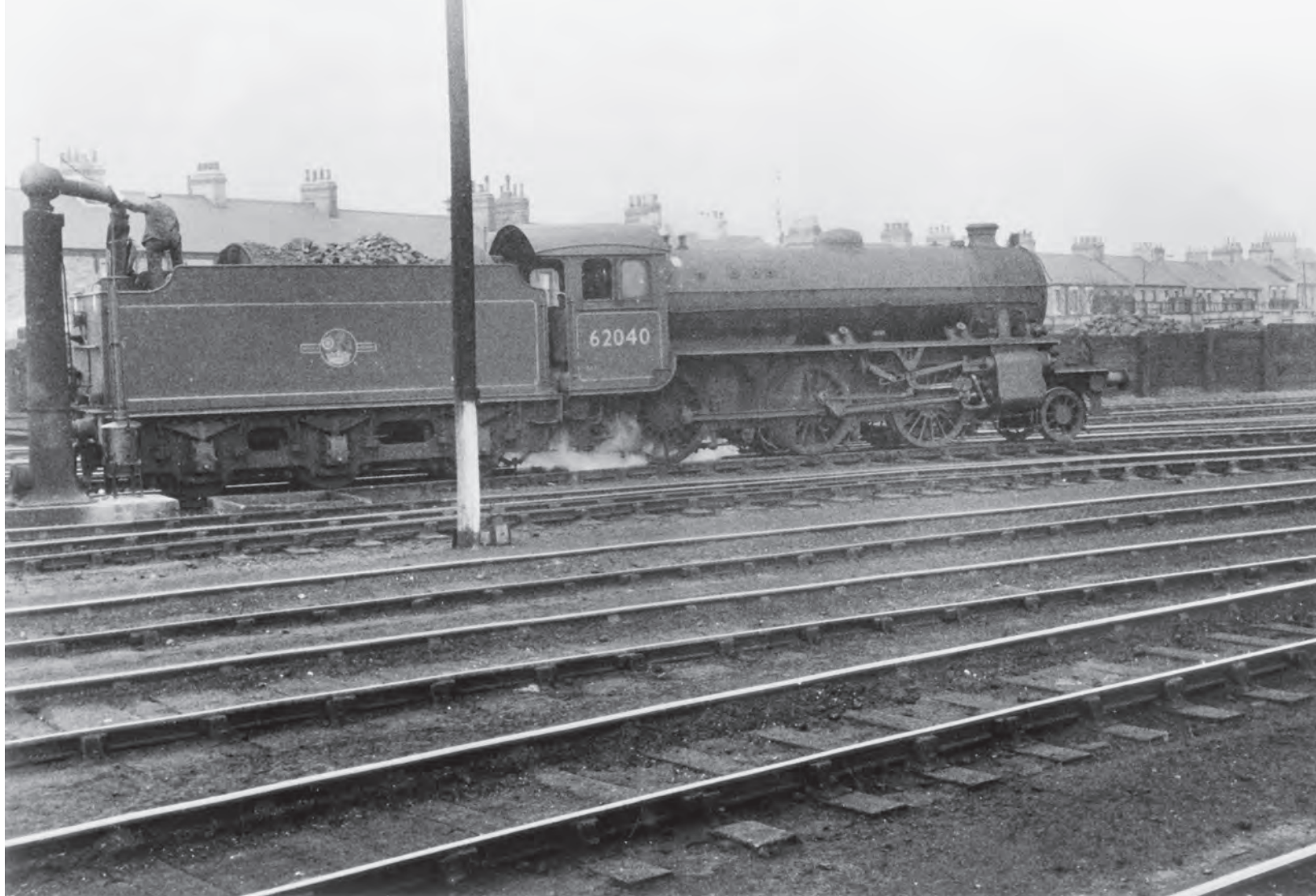
'K1' 2-6-0 62040 has emerged to have its tender replenished, with a crew member watching the water level rise.
