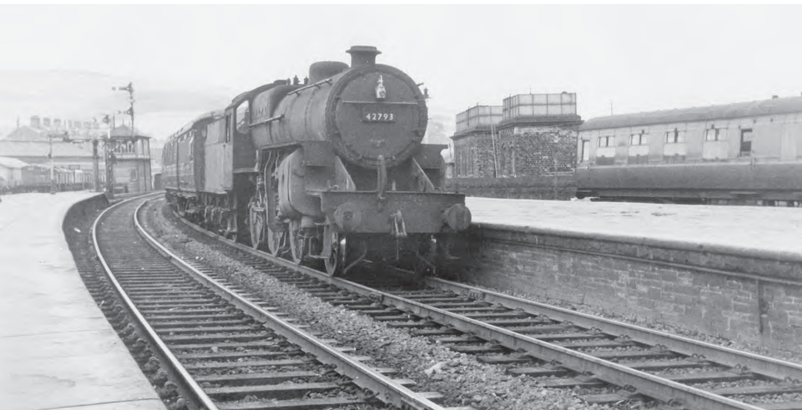
'Crab' 2-6-0 42793 is slowing for Skipton station with a northbound local service. The front coach is a Gresley brake vehicle. Skipton's south signal box is to the left and two water tanks are evident to the right of the locomotive. An ex-LMS brake awaits further work. 6 August 1962.
