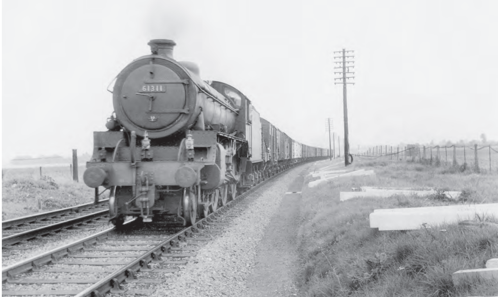
Now moving east of Chelmsford to an occupation crossing in the vicinity of Boreham on 22 August 1960, we find a useful cycle location for photographing trains in action. Modernisation was in the air, but steam still had work to do. Looking east, Colchester's 'B1' 4-6-0 61311 is at the head of a westbound van train. Note the oil lamps above the electric lights on the bufferbeam.
