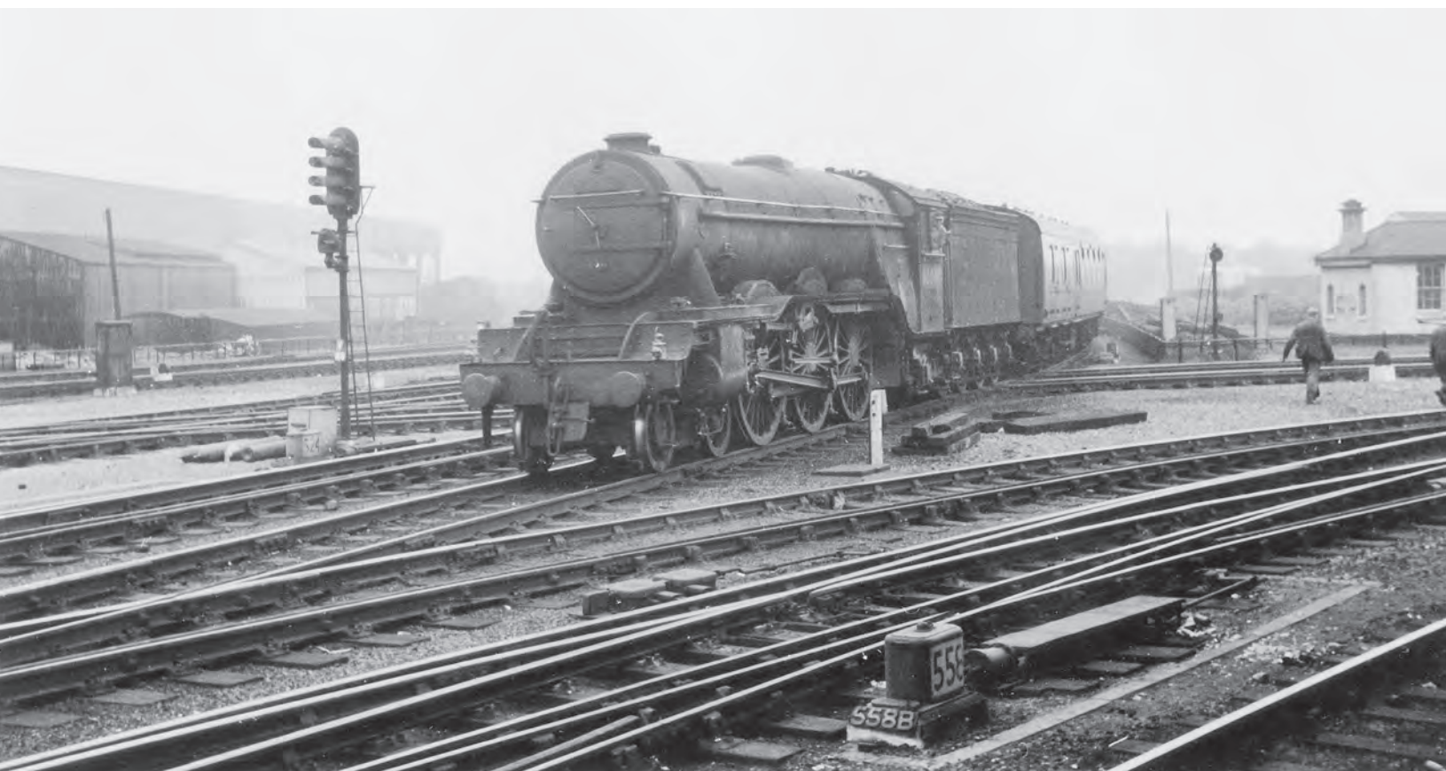
Dull weather persists and the locomotive is dirty, but Gateshead's single chimney 'A3' 4-6-2 60040 Cameronian is arriving with an express from the North. To the left of the picture, locomotives rest outside the shed. 6 August 1959.
