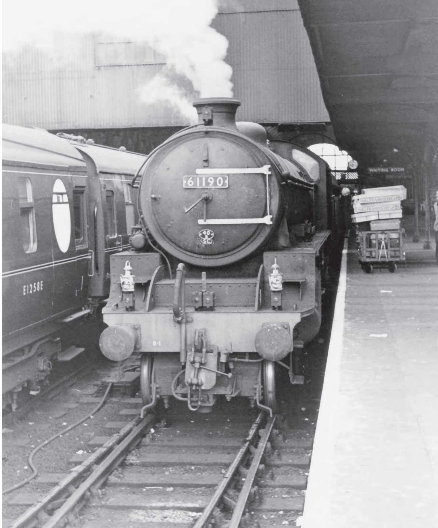
Thompson 'B1' 4-6-0 61190 of Immingham shed is awaiting departure with an afternoon Cleethorpes service. The driver is leaning from the cab to see all is well, whilst flower boxes rest on a platform trolley. The locomotive has electric lighting supplemented by oil lamps. The design of coach on the adjacent track complements the locomotive. 7 August 1961.
