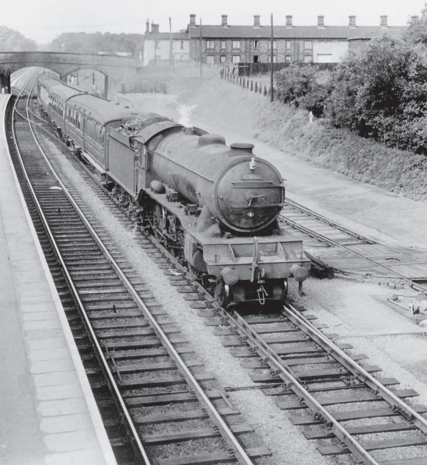
'K3' 2-6-0 61862 enters Audley End main line station, heading for the staggered platform for up trains, where it will connect with the railbus service. The Gresley brake is prominent at the front of this train. Note the wagon turntable to the right of 61862.
