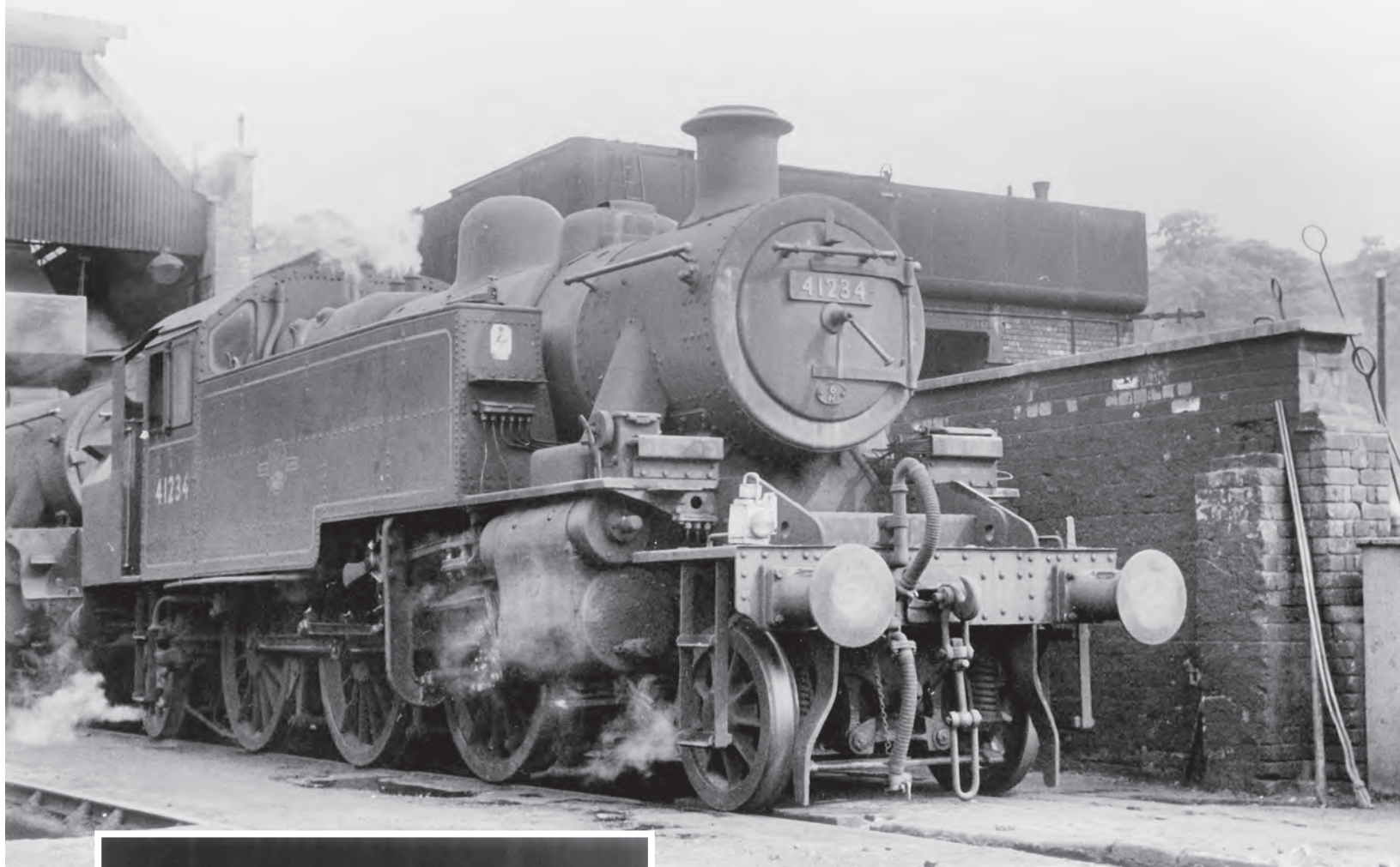
Bangor resident Ivatt '2MT' 2-6-2T 41234 is ready for duty, which may well be the freight on the Amlwch branch. Bangor shed closed to steam in October 1966. 7 June 1964.
