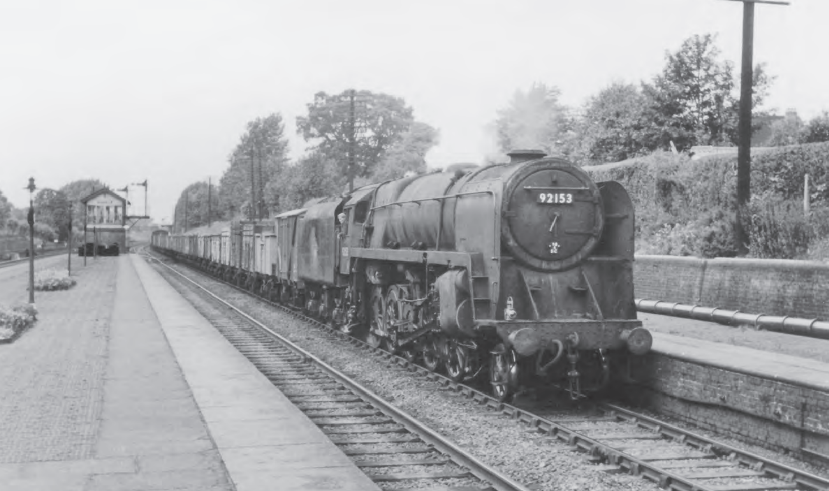
BR '9F' 2-10-0 92153, still carrying a single chimney, is slowly dragging a rake of wagons towards London. Its gentle progress gives the fireman a chance to survey the scene. 92153 is from Toton shed. Note the tidy flowerbeds to the left of the picture.
