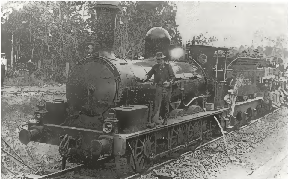
A number of contractors were used on the construction of the North Coast Railway. The well-known contractor Smith & Timms obtained a locomotive from the Railways in 1909 and used it on such duty in the area for about 12 years. The locomotive was A class, 0-6-0 tender engine No.193 (Henry Vale, 1882, B/N 18). Whilst used on railway construction, the name 'Gloucester' was painted on the sides of the six-wheel tender. It reverted to railway ownership at the completion of work and was renumbered 1010, finally being scrapped in 1937. In this photo (c.1912), 'Gloucester' is shown on a construction train near Dungog.
