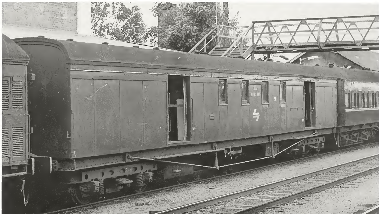
KP845 in the consist of the South Mail at Junee in 1981. While most KP vans had been refurbished, KP845 still retains the deep letter board sides and standard windows and is fitted with 2AN style bogies. KP754 (below) basks in the morning sun at Sydney Terminal in the early 1970s, displaying some of its mail sorting interior. The deep letter board sides have been replaced by thick Masonite panelling. The side windows have been shortened in height and the van is fitted with 2AH bogies, which were reworked from the unique Dean bogies.
