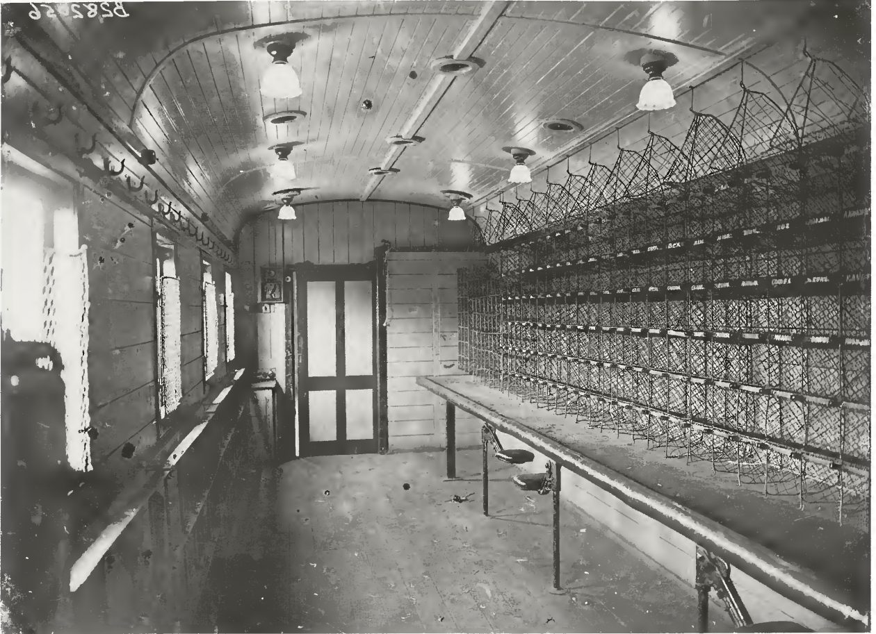
Interior view of a KP showing pigeon holes labelled for various destinations, the Sydney suburbs of Bondi and Coogee being prominent in this photo.
