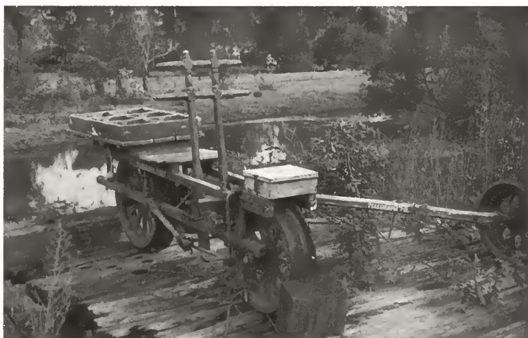
A station tricycle. These simple, hand-powered 'one-man horrors' were used for a variety of tasks. The prime purpose of this particular machine was to be a means of replacing the lamps in station signals; the rack for holding six lamps is shown fixed behind the seat. Apart from their intended uses, station 'trikes' could be used for transport to the local Watson Taylor Lake for a day's fishing, if needed.
