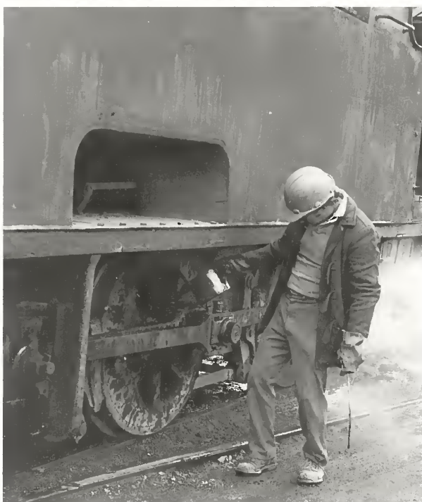
All locomotives require maintenance, particularly steam locomotives. In the last years of operation, the Portland engines were manned by a driver who performed all manner of duties from driving, through firing, to coaling and watering the engine. He was assisted in these chores by a shunter on most occasions. A job that was always carried out by the driver was the one depicted here - that of oiling the motion. All operational staff (and visiting photographers) were required to wear hard hats within the works. R.D. Love
