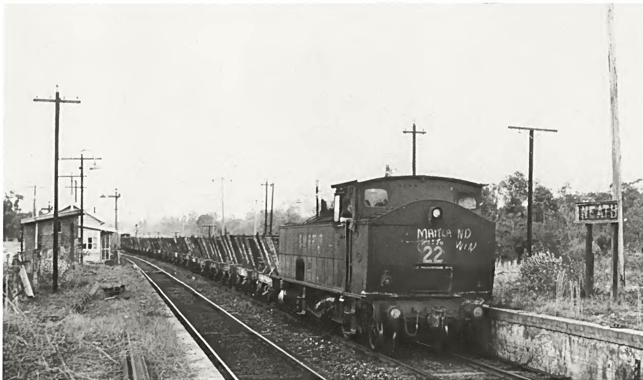
Above: Two lengthy side platforms were provided at Neath, each capable of accommodating quite respectable trains. In an era long after their need had passed, 2-8-2 tank No.22, leads a line of empty non-air coal hoppers through the station as the train makes its way from East Greta Junction to the mines. The signal box is situated at the far end of the left hand platform.
