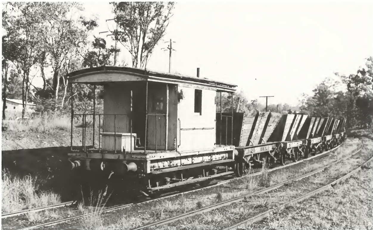
These three photographs show standard coal train rolling stock on the South Maitland Railways for over seven decades. There were the black Beyer, Peacock 2-8-2 tanks, such as No.22; red non-air coal hoppers of which this pair is typical; and, to bringing up the rear, the Company's version of a CHG van, a grey livery distinguishing it from its Government cousins.
