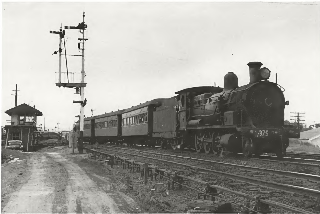
5375 reverses a three-car train past the signal box into the carriage sidings at Wollongong in the early 1960s. The main line signals in the vicinity of Wollongong at this time were of the upper quadrant type. The example shown here has a wooden main post.
