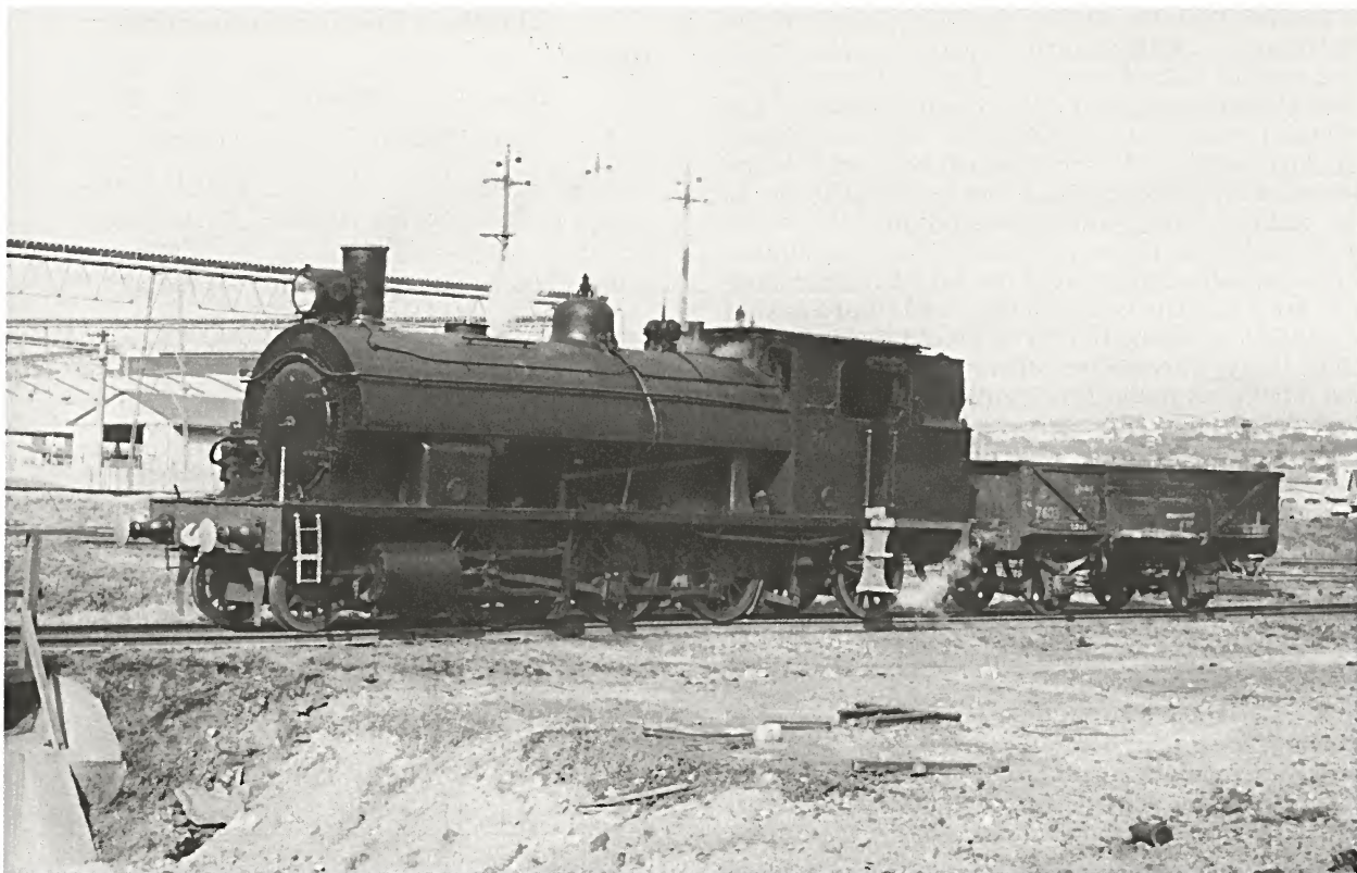
The 26 class 2-6-2 saddle tank engines were specially built to work short-haul mineral trains. Some of the class were placed immediately on Illawarra coal and blue metal trains when introduced into service in 1892. They disappeared from the Illawarra when Thirroul replaced their former depot at Waterfall in 1917. However, the 26s were to return in force in 1949, but were confined to shunting duties in the Port Kembla industrial network. By then most at Port Kembla had acquired an electric headlight plus a steam turbo-generator to provide the necessary current. 2609 fortunately escaped the disfigurement of automatic couplings and needed an S truck as a match wagon for coupling to non-buffered trucks.
