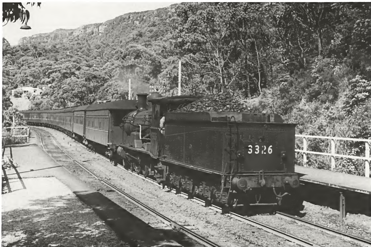
The running of tender engines on the local trains to Scarborough and Coalcliff required some tender-first working in the absence of a turntable at either of these termini. This example shows 3326 arriving at Wombarra with a ten-car train from Port Kembla on 19 December 1963. R.K. Booth
