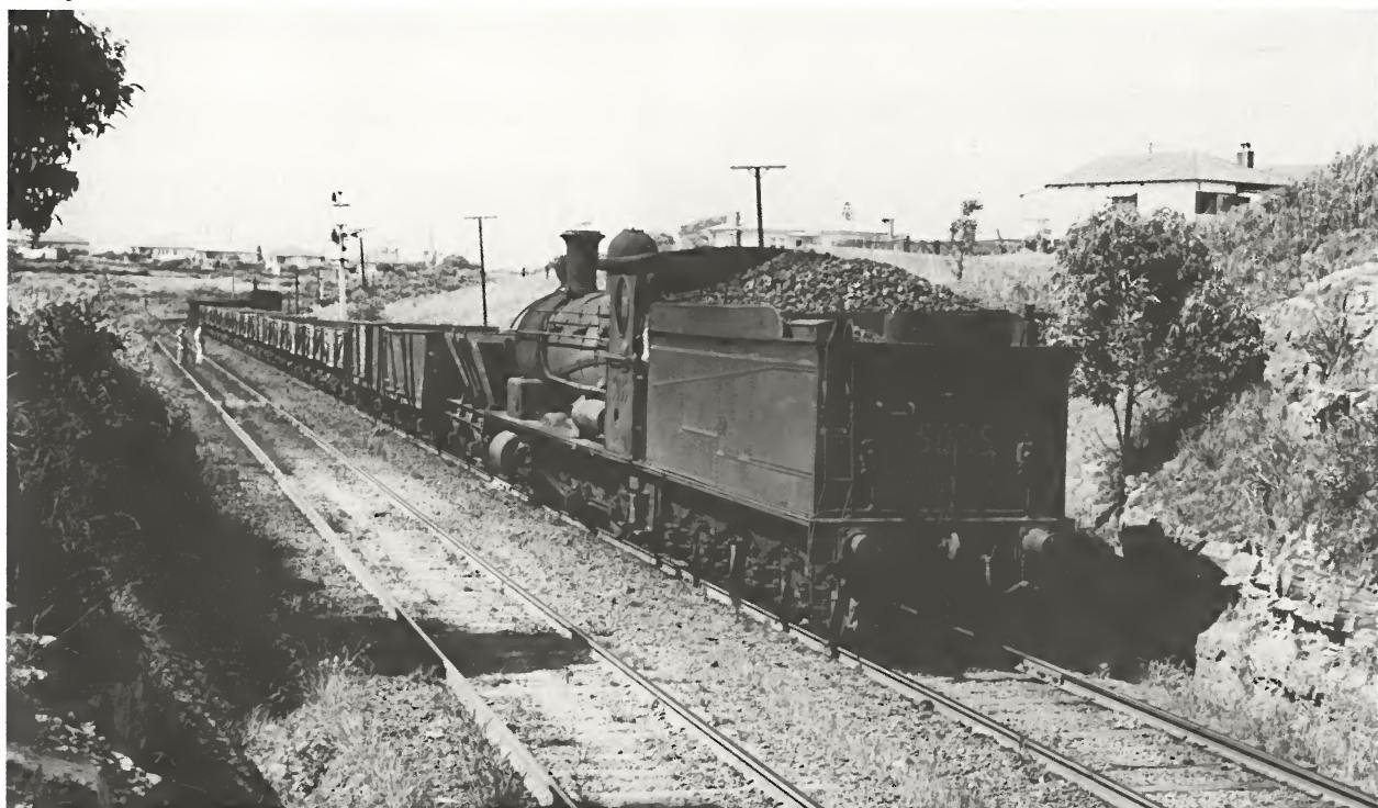
Locos on local goods trains between Thirroul and Port Kembla usually worked chimney-first on the down and tender-first on the up. 5035 has an assortment of four-wheel wagons in tow as it approaches Thirroul on 5 February 1960. Even by this date, 50 class engines still fitted with original style tenders were becoming a rarity.
