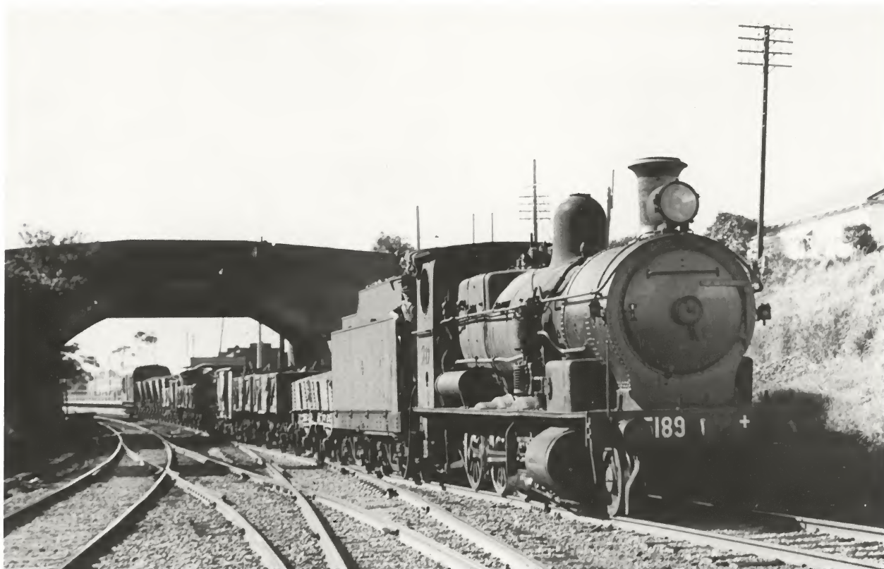
5189 takes the Port Kembla branch at Coniston with a train from Thirroul in 1958. The leading truck is a wooden D wagon with a load of ashes from Thirroul loco. A mixture of S and K wagons leads five LCH coal hoppers and a brakevan, comprising a typical goods train of the period.
