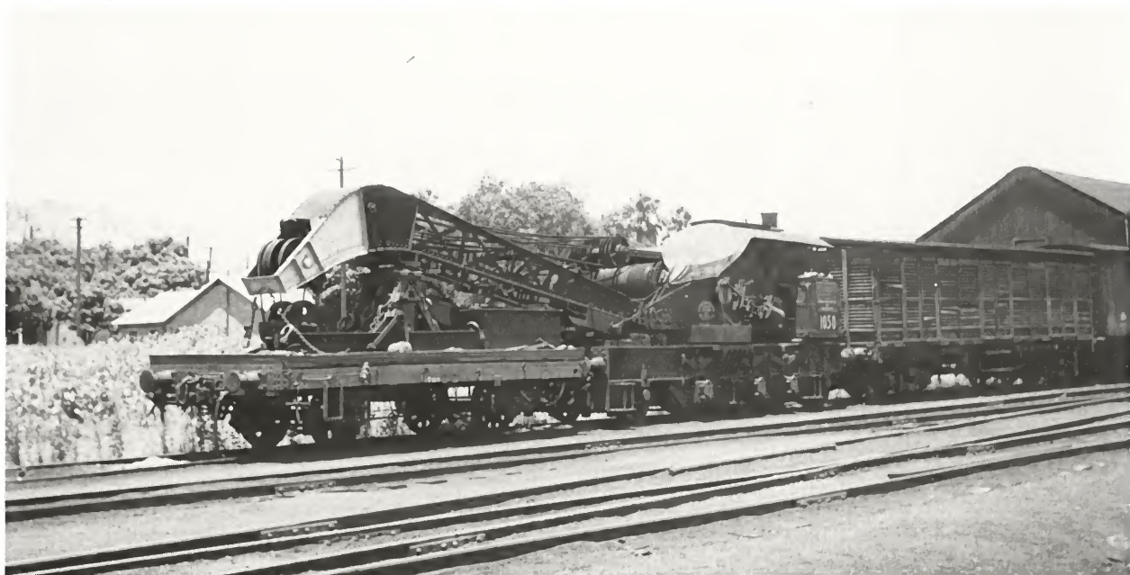
Below: Werris Creek depot's 30-ton accident crane 1050, its jib support vehicle and the accident vans stand in a siding at Werris Creek loco on Saturday, 30 December 1961.
