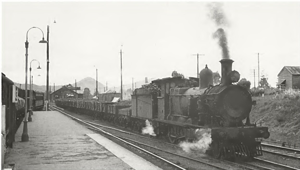
Superheated 3142, complete with cowcatcher at the front and Eveleigh Works builder's plate fitted to the cab side, shunts Mudjee yards. Taken from the Sydney end of Mudjee station, this photograph shows the dock platform at left and Mudjee loco in the distance. The peak of Mt. Frome is in the distant background. Wednesday, 27 December 1961.
