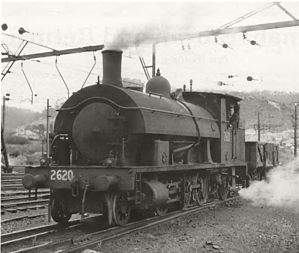
In steam days, it was always a pleasure while at Lithgow to watch the 26 class 2-6-2 saddle tank engines shunting the yards. Here, on Tuesday, 26 December 1961, 2620 with its S match-truck goes about its work.
