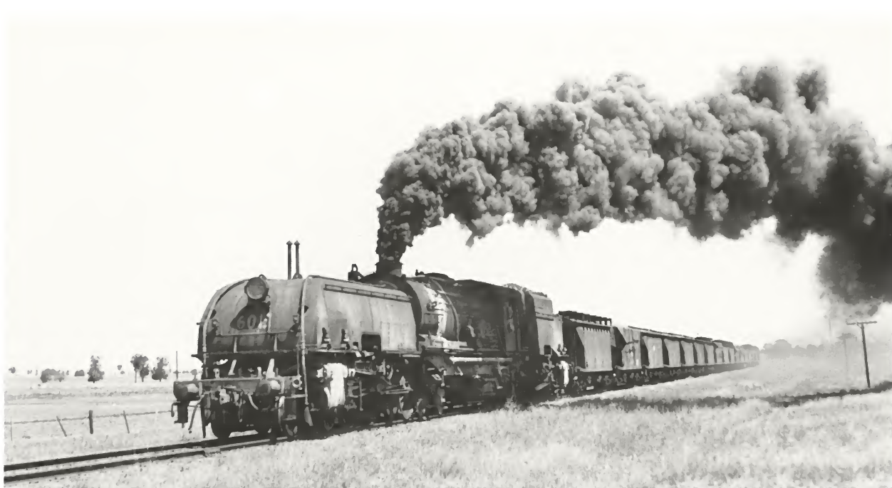
The full load for a Garratt in the Peak Hill - Narromine section was 1500 tons. 6015 is having no trouble with 16 BWHs and sheeted BCHs plus a van (1000 tons gross) as it steams along near Narwonah, south of Narromine on 5 January 1967.
