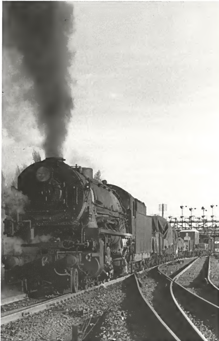
Exerting maximum tractive effort, 5717 stutters noisily out of Junee with No.56 Goulburn mixed trailing out of the yard in the background. Assorted steam leaks around the Mountain's front end are drowned by the blast from the three cylinders as the train attacks the bottom of the three mile, 1 in 66/70 grade out of town. The important branchline to the south-west can be seen diverging into the bottom right corner of the photograph.
