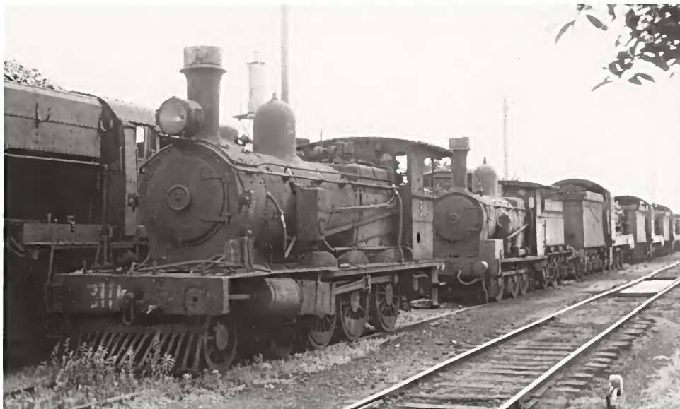
It is the end of the road for a long line of stored locomotives at Broadmeadow depot, photographed next to several out-of-steam 60 class engines on Sunday, 31 December 1961. At the front of the line is former Werris Creek engine 3111, still retaining its cow-catcher. Behind 3111 are 1939 and several 35 class engines. Metal caps, such as that on the funnel of 3111, were used at Broadmeadow on stored engines to exclude rain.
