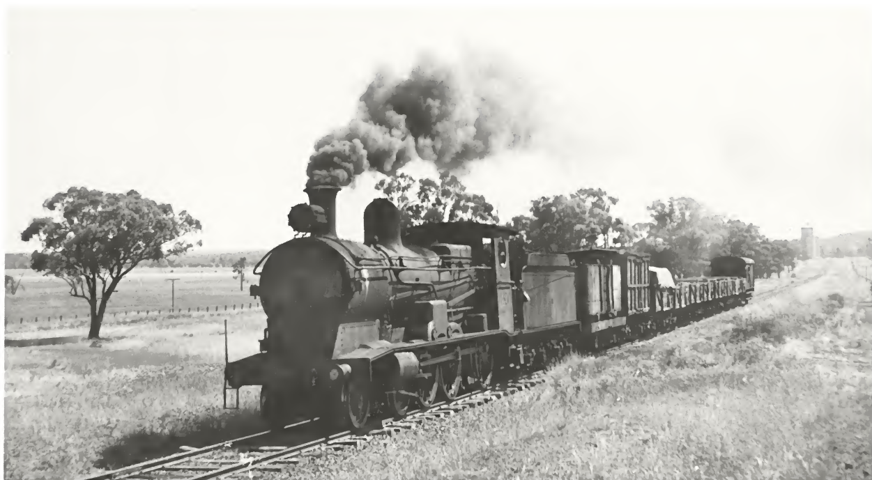
With the Muronbung wheat silo in the distance to the right, 3326 and its load of four wheel water gin, CV and 10 S trucks of new railway sleepers plus a PHG van, head for Dubbo and home. Engine 3326 was fitted with a 'Sunbeam' type headlight in days gone by, the number of the locomotive visible in a panel on the sides of the light. This engine was also fitted with steam heating controls, having spent many years at Goulburn on the Cooma line duties prior to working in the Dubbo area.
