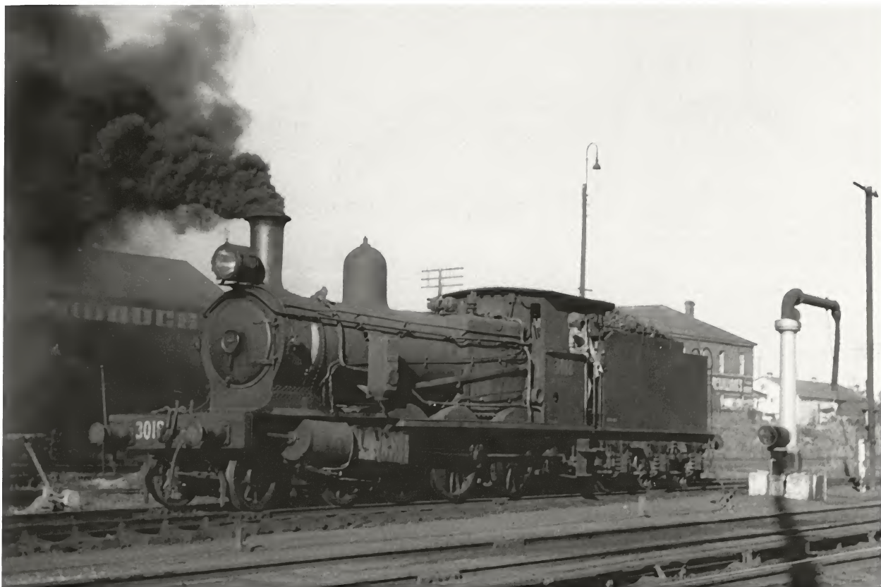
The fireman has been busy attending to the fire of 3018 as it reverses past the water column near the coal stage while shunting in Dubbo yard. The yard shunters at Dubbo were usually 30T class engines and they typically faced the west. Thursday, 28 December 1961.
