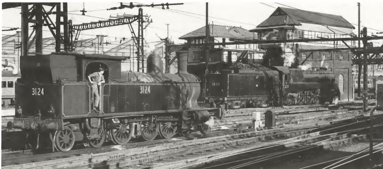
Yard shunter 3124 and crew watch 3809 backing down Sydney yard to couple onto and depart from Sydney terminal station on No.49 South, to Moss Vale, at 3.54pm. Sydney East signal box can be seen behind 3809. Of interest is the extended bunker fitted to 3124.
