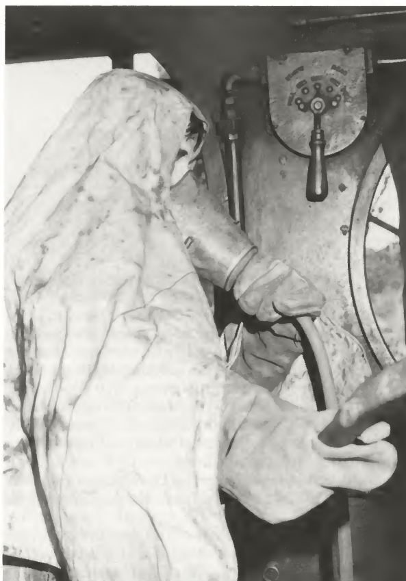
Hood, gauntlets and mask in use. It was necessary to hold the mask to the mouth and nose, drive the engine and be prepared to control slipping by operation of the sanding valves, all in a blackened cab with copious amounts of steam, fumes, smoke, noise and dust.
