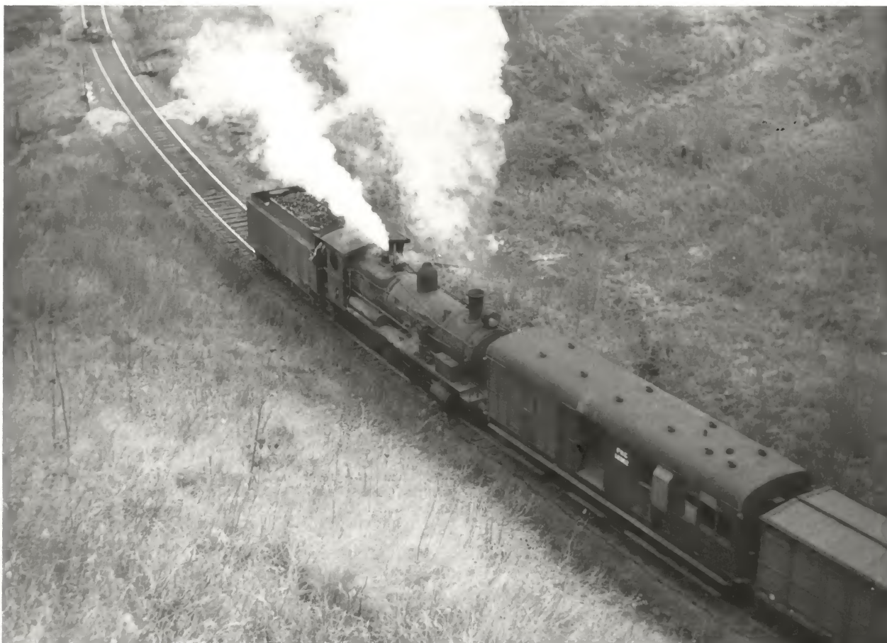
The bank engine (5483) also has a clean fire as it approaches the tunnel. No doubt the experienced Murrurundi crews know how to prepare for travel through the narrow confines. Note the fettler on his trike following along behind.
