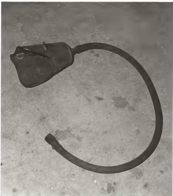
Breathing mask supplied to each engineman. The mask was of metal construction and was fitted with a tube, to be connected to the engine air supply.
