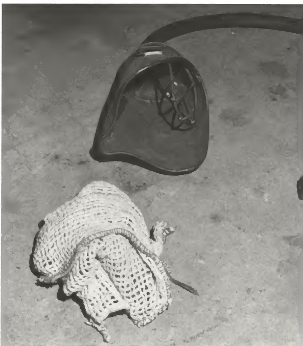
The mask was fitted with a hinged wire gauze cover and a wet sweat rag or sponge cloth could be inserted behind the cover to act as a filter.
