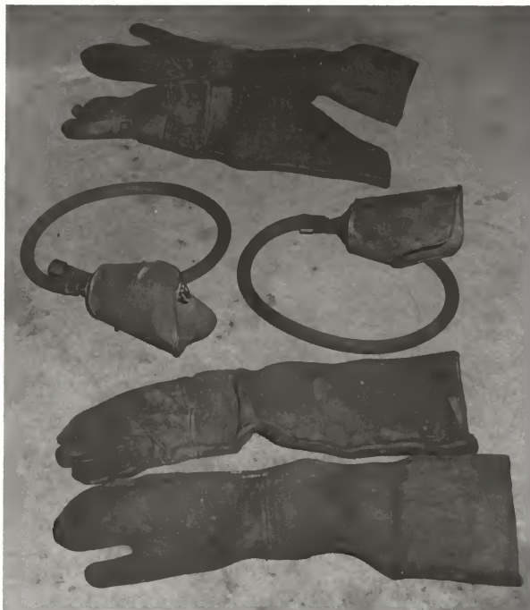
Respirator kits included hoods (not shown), four gauntlets (long gloves) and two masks fitted with flexible air tubes.
