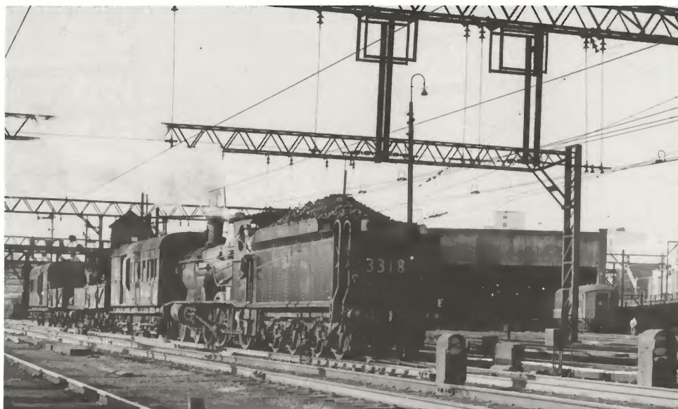
The crew of 3318 pose for the photographer on Monday, 16 July 1962 as the rubbish or 'kibble' train moves through Sydney yard. A typical consist for the train is shown here with five-ton crane locomotive 1044 at the centre and an S truck and goods brake van at each end. The eastern carriage cleaning sheds can be seen at right of picture.
