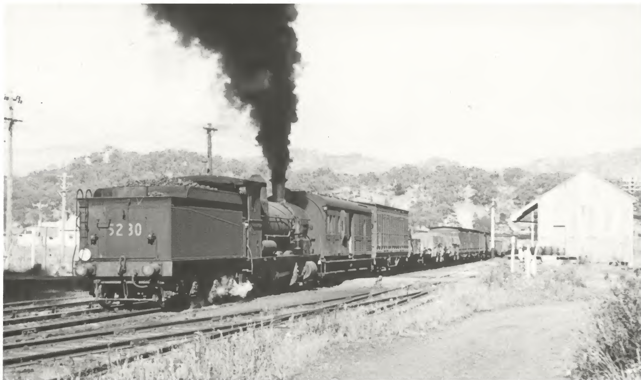
Where it all started. Double-heading of down goods trains from Murrurundi to Ardglen was banned as a result of fatal accidents in the tunnel. All assisting was from rear-end bankers. Engine 5230 earns its keep as it banks a down goods (with 5442 in front) out of Murrurundi yard, heading for the range and the tunnel, in March 1963.
