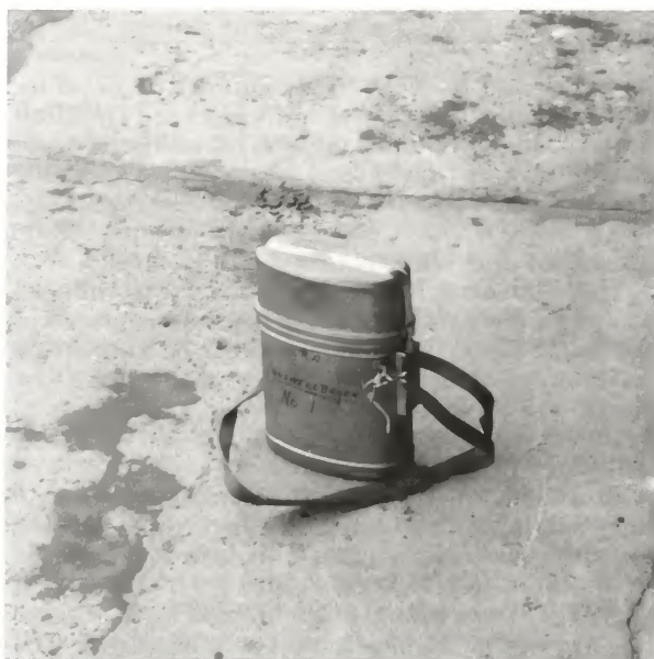
The breathing equipment is provided in sealed metal containers, two of which are supplied in the box shown previously. The containers are sealed for security reasons, and should the seal be broken, indicating use, the equipment is withdrawn for reconditioning. The container is shown at Muswellbrook.
