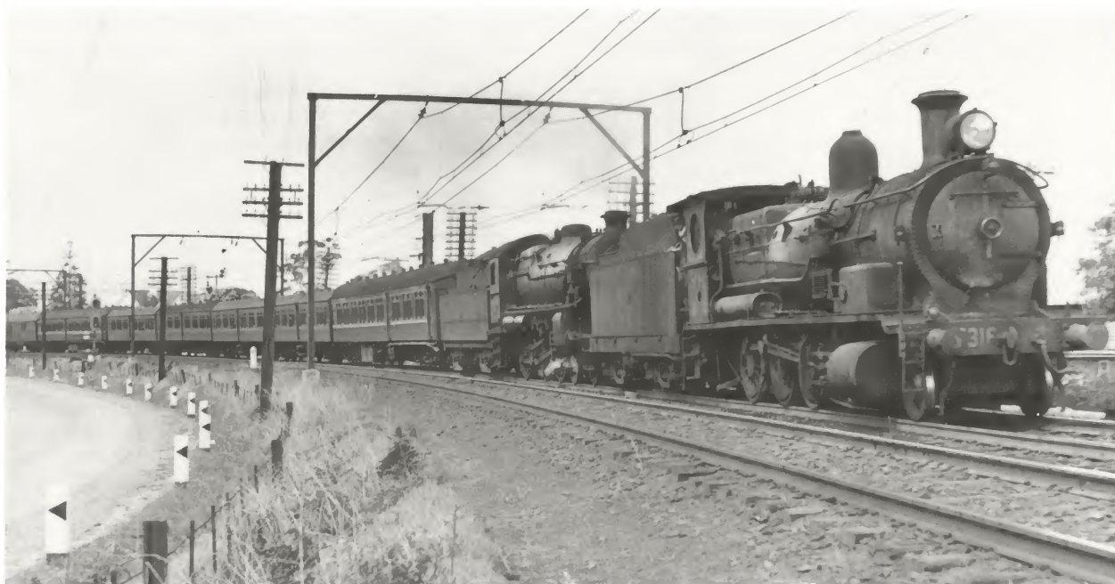
Electrification of the western line to Lithgow is not far distant as 5316 assists train engine 3647 at the head of No.25 Bathurst passenger. Enfield engine 5316 was on loan to Valley Heights depot, where it was attached to the 36 for the climb to Katoomba. The additional marker lamps, on the front buffer beam and smokebox, of 5316 are of interest. The train was photographed near Springwood on Wednesday, 19 September 1956.
