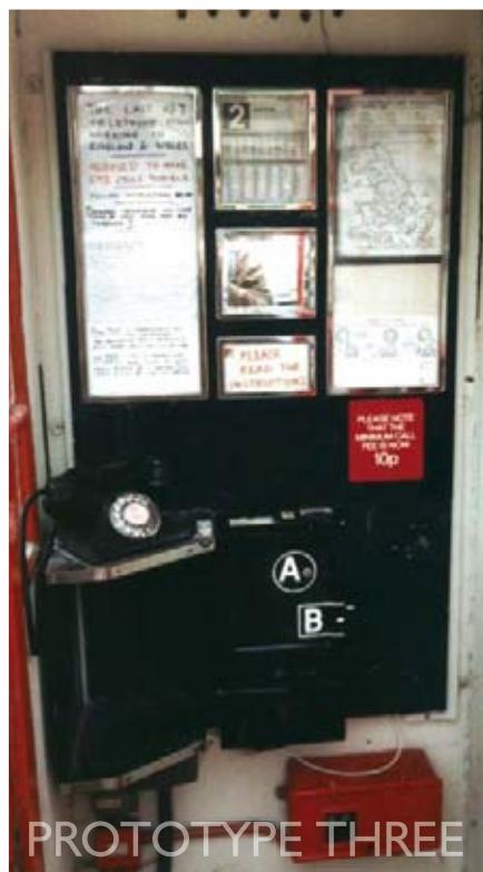
PROTOTYPE THREE The classic 'Button B' phone box interior. These disappeared in the 1960s. True 'phone box spotters will notice that this is in a K1 box at the Tramway Museum, Crich.
