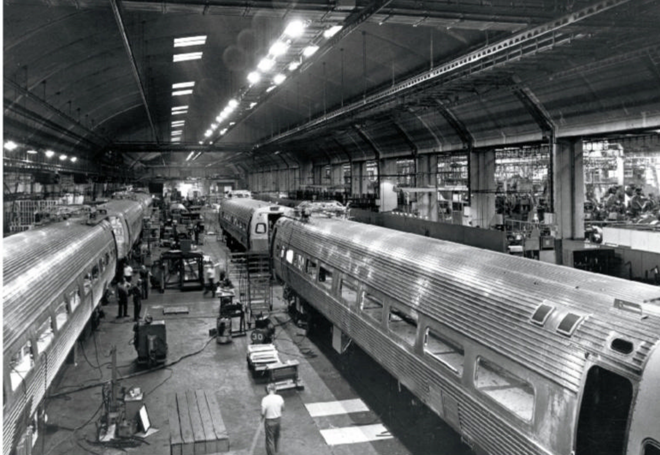
Partially completed Metroliner M.U. cars occupy the shop floor at the Red Lion plant. Here Budd built 61 Metroliners in the late 1960s and 642 nonpowered Amfleet versions in the 1970s and '80s. Budd
