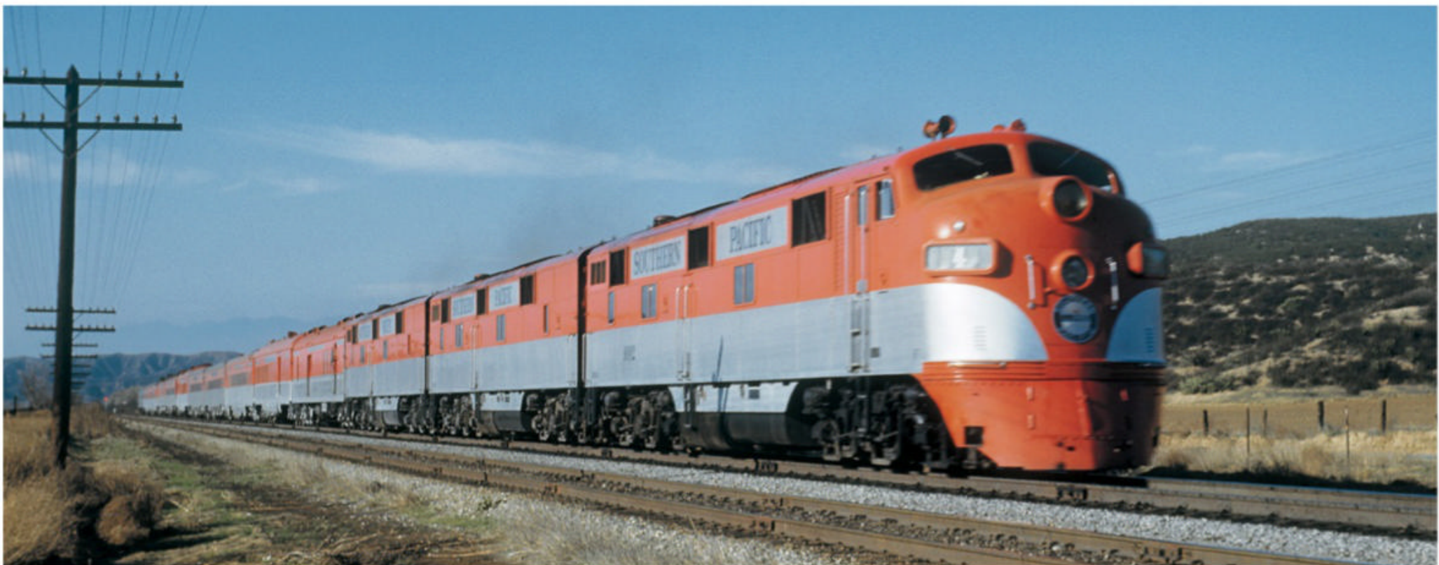
Put on hold for the duration, passenger-train dieselization came roaring back after World War II; EMD's E7 of 1945 led the way, becoming the top-selling passenger diesel of all time. Three Southern Pacific E7s whisk the Golden State east at Nicklin, Calif., in January 1948. Frank Peterson, Alan Miller collection
