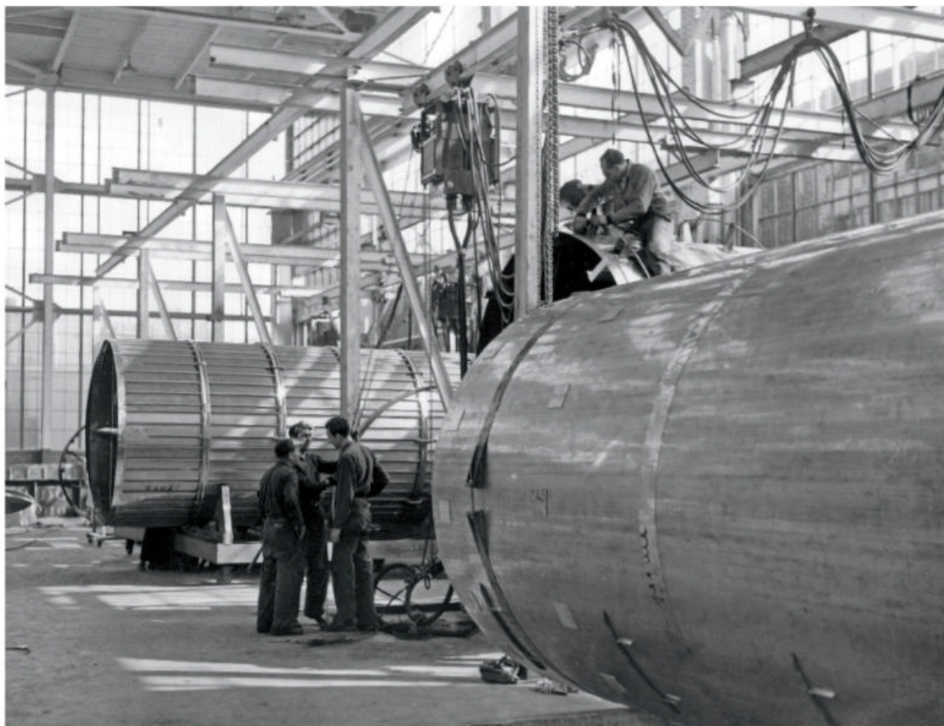
Workers fabricate smokestacks of weight-saving stainless steel for Navy destroyers at Budd's Hunting Park Avenue plant in October 1941. Kevin J. Holland collection
