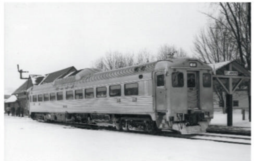
The Rail Diesel Car, introduced in 1949, was a big postwar success for Budd. Prototype 2960, demonstrating on Canadian Pacific, pauses at St. Jovite, Quebec. CLASSIC TRAINS collection
