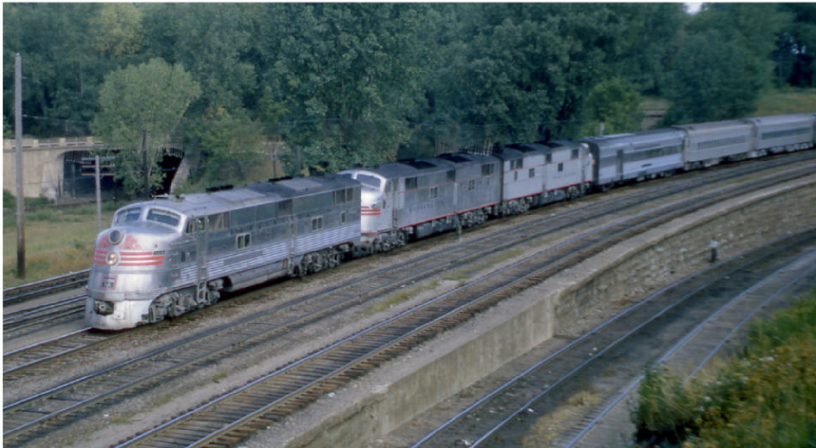
After 1939, Zephyr power progressed through EMD's E5, E7, E8, and E9 models. On August 5, 1964, an E5 and two E7s (with stainless and painted flanks) lead the Chicago-bound Morning Zephyr in St. Paul. Tom Smart, Brian Schmidt coll.
