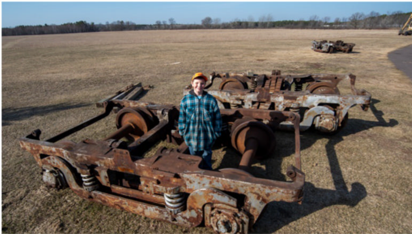
Alexander Vreeland, 11, stands within one of the MTZ's trucks on April 3, 2021, prior to its rebuilding. The trucks are being completely rebuilt after disassembly, bead-blasting, repairs, and repainting.
