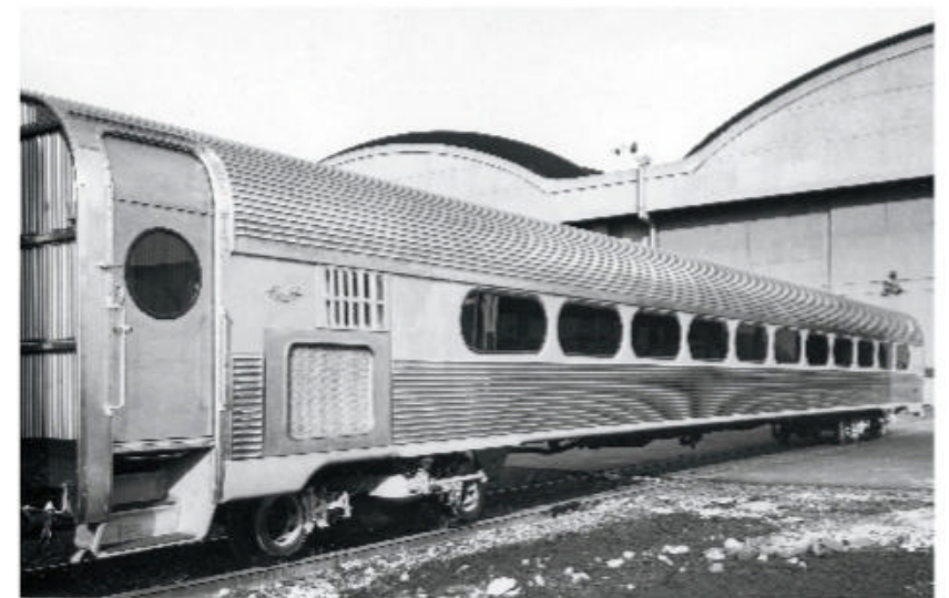
Intended as a platform for a variety of car types, Budd's Pioneer III coach of 1956 remained a loner, although it was the basis for PRR and Reading electric multiple-unit cars. Budd
