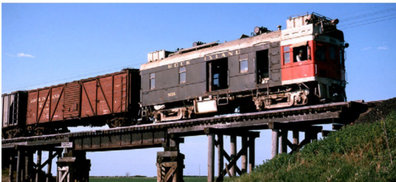
Rock Island's 15 EMC-powered units of 1927-29 (some converted from baggage cars, others built new) could haul train-sized loads; RI 9006 still worked branches out of Fairbury, Nebr., in 1962. Frank Tatnall
