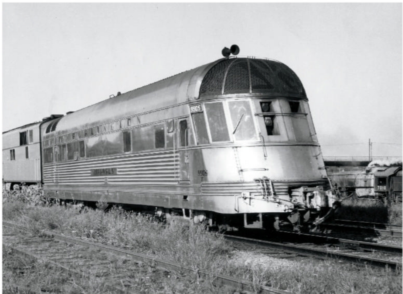
Fifteen years after the top photo on the opposite page, motor 9905 has been put into the general passenger pool and converted to a B unit. It's at Omaha with an E7 on September 13, 1952. Charles E. Winters
