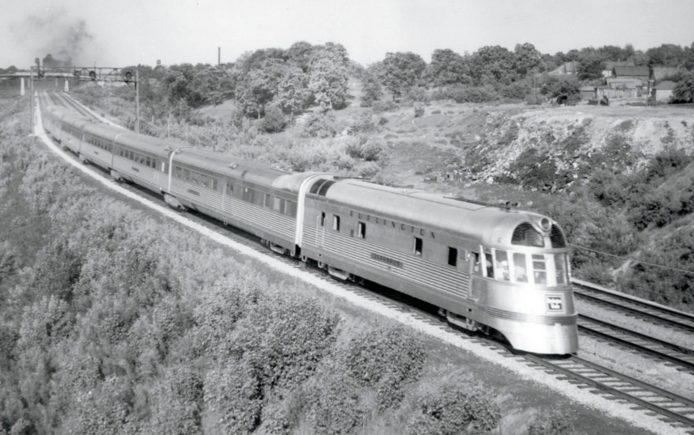
CB&Q 9905, named Zephyrus , heels to the curve on the east side of Aurora, Ill., with the Afternoon Zephyr for Minneapolis in June 1937. This is the original configuration of the 1936 Twin Zephyrs : a diesel locomotive ("motor" in CB&Q parlance) and six articulated cars. L. E. Griffith
