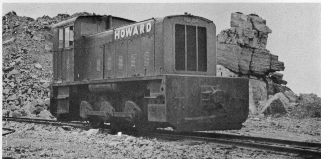
INDUSTRIAL DIESELS — (4) JOHN HOWARD & CO. LTD, HEADLAND QUARRY, ANGLESEY. (NGN73/17 & 55/17) One of the two 3ft 6ins gauge 165HP Rustons, No. 384143 of 1955 an 0-6-0 Diesel Electric, which have been scrapped on site. Rail transport soon proved unsatisfactory on this contract and the rail system was already out of use when the photo was taken in July 1969.
