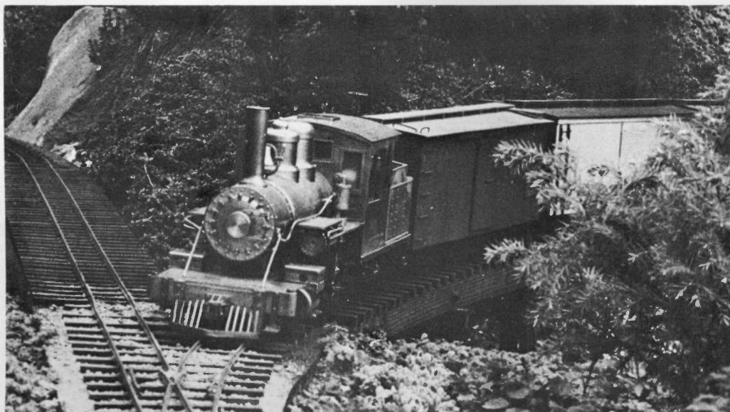
SANDY RIVER & RANGELEY LAKES R.R. \frac{1}{3} scale model of No.10 — on a 2\frac{1}{2} chain (55") Garden curve.
