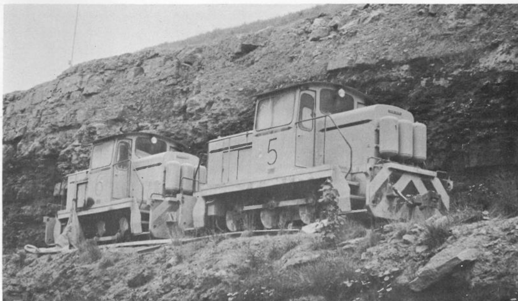
INDUSTRIAL DIESELS — (2) A.P.C.M. LTD, DUNBAR CEMENT WORKS, EAST LoTHIAN. (NGN72/18) The two 3ft. 6ins. gauge English Electric 0-6-0 Diesel Hydraulics of 1966, Nos. D926 and D925, stand out of use and awaiting a decision as to their fate after only four years service. (Pete Nicholson)
