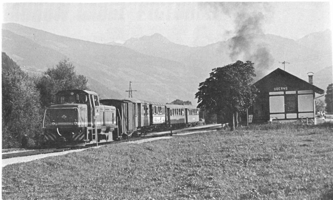
2nd Place – Category B (Narrow Gauge Internal Combustion). By Peter Shoesmith of Birmingham. Photo : Zillertalbahn, Tyrol, Austria. 760mm gauge "D8" 8-wheel diesel hydraulic (Orenstein & Koppel 26615 of 1967) at Uderns with a train for Mayrhofen, passing a Jenbach bound steam train. 7 September 1972.
