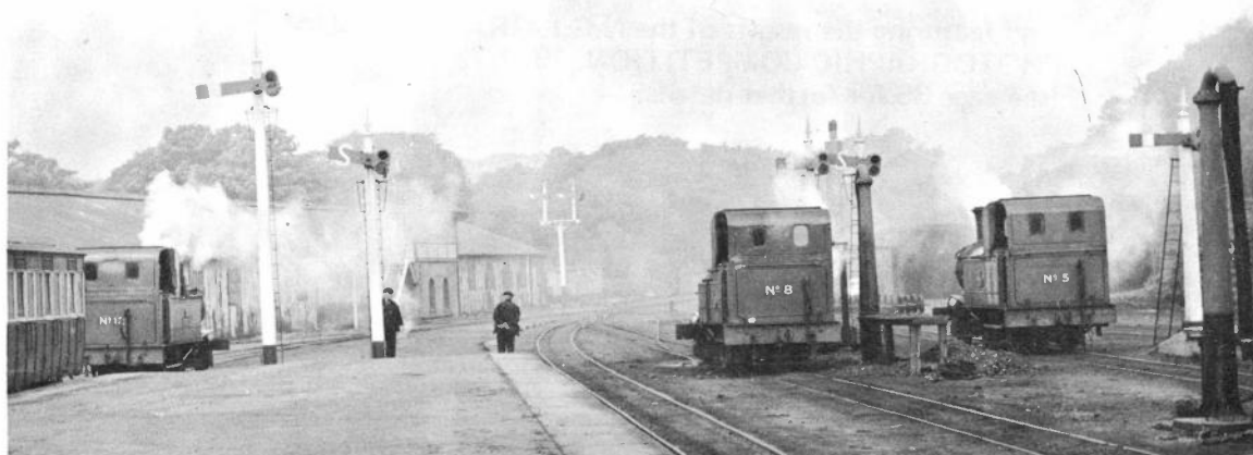
"THREE LITTLE ENGINES — on the three foot". Douglas Station, Isle of Man 12/8/65. Waiting to back onto their respective Port Erin, Peel and Ramsey trains are Beyer-Peacock 2-4-0Ts 12, HUTCHINSON (5126 of 1908), 8 FENELLA (3610 of 1894) and 5 MONA (1417 of 1874) — all in red livery. (Alan Bowler)
