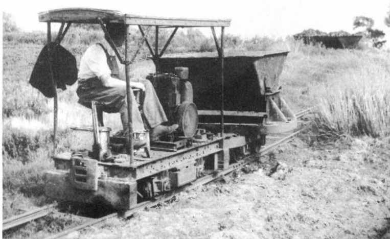
BLITHE VALLEY WORKS, CHECKLEY. 4wheel Diesel (ex Petrol) Lister No. 39419 of 1953. Type 'R' ascending the tip 2/9/71.
