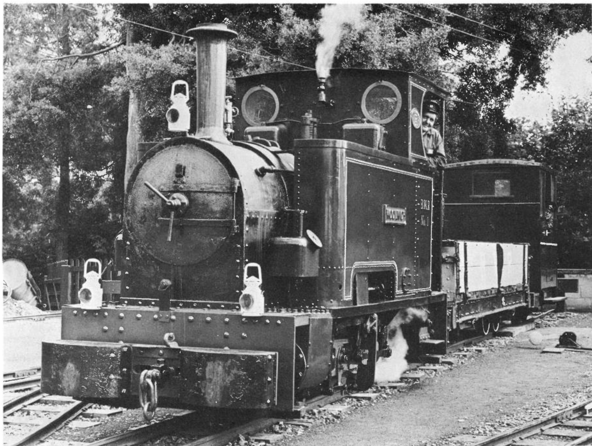
No. 1748, WOOLWICH — the hardest worked Avonside in Britain and quite a 'monster' for only 1ft 6in gauge. It is now the only survivor of a class of 16 built during the First World War for the Royal Arsenal at Woolwich, London. It was purchased for use at Bicton in 1962 and fitted with a conventional chimney. This loco set a trend now being followed by several other railways today as it is oil-fired. (Richard Tarr, Courtesy The Clinton Devon Estates)
