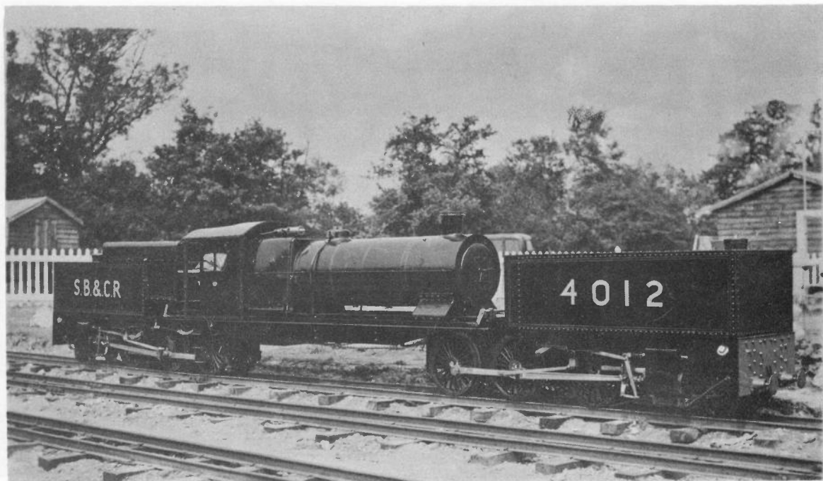
10 1/4 in gauge Super Power, one of the two Kitson built 2-6-0 & 0-6-2 Garratt built 1938 with 4 cylinders 3 1/2 in x 5 in. Weight 2ton 5cwt capable of hauling trains of 100 passengers. (collection:- R.N. Redman).
